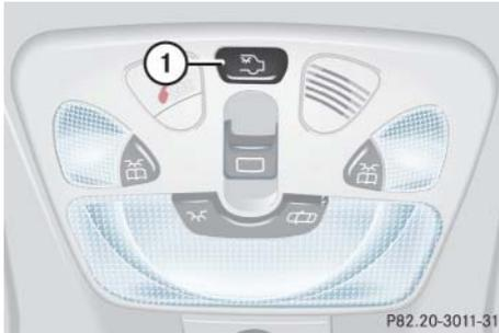
① Switch for cargo compartment lamps
