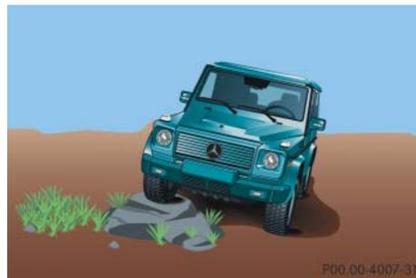
**!** *Obstacles can damage the vehicle underbody or suspension components. If possible, use the assistance of a second person outside the vehicle to scout the path you intend to take and check for adequate ground clearance when you cross obstacles with your vehicle. The person assisting you outside the vehicle should always be a safe distance away from the vehicle and positioned so that he or she cannot get hurt in case of any unexpected vehicle movement.*
