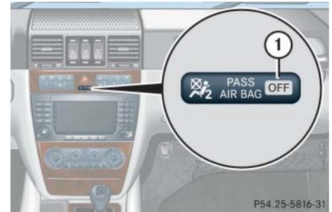
① Front passenger front air bag off indicator lamp
