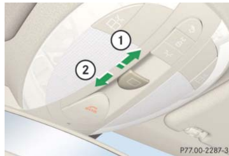
Roof panel switch
