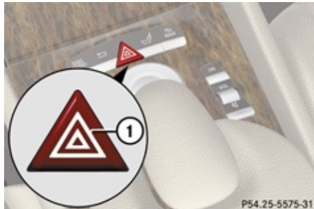
① Hazard warning flasher switch
