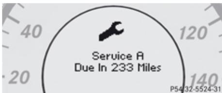
The maintenance services will be indicated by showing a service type A through type H in the multifunction display. Types A through H are classified based on estimated time needed to perform the maintenance service, ranging: from Service A
