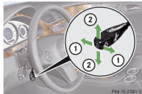
① Adjusting steering wheel, in or out
