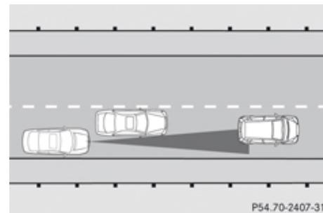
A vehicle traveling in your lane but offset from your direct line of travel may not be detected by DISTRONIC. There will be insufficient distance to the preceding vehicle.
