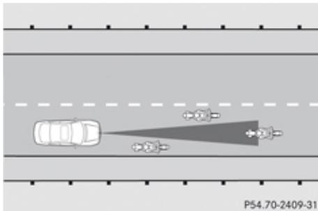
Because of their narrow profile, the vehicles traveling near the outer edges of the lane have not yet been detected by Distronic. There will be insufficient distance to the preceding vehicles.
