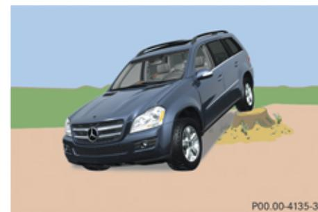
**!** Obstacles can damage the vehicle underbody or suspension components. If
