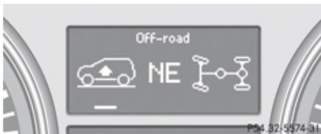
The vehicle is raised from off-road level 1 to off-road level 2.
