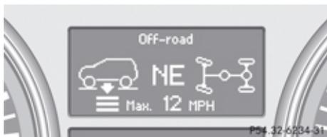
The vehicle is lowered to off-road level 2.
