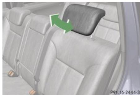
The angle of the head restraint for the outer second-row seats or the third-row seats can be adjusted manually.
