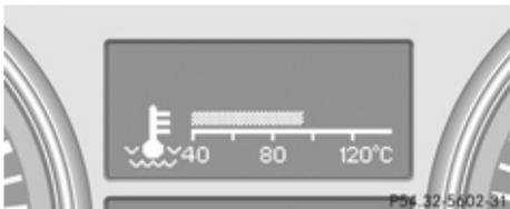
During severe operating conditions, e.g. stop-and-go traffic, the coolant temperature may rise close to 248°F (120°C).
