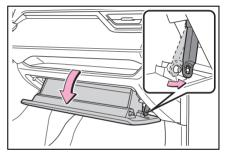
3 Push in each side of the glove box to disconnect the claws, and then slowly and fully open the glove box while supporting it.
