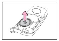
3 Remove the depleted battery.
