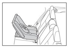
3 Run the seat belt through the child restraint system and insert the plate into the buckle. Make sure that the belt is not twisted.
