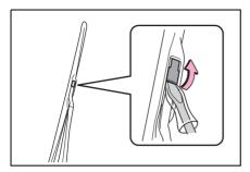
3 Slide the wiper blade to remove it from the wiper arm.
