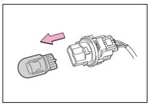
3 Install a new light bulb then install the bulb base to the light unit by inserting it and turning the bulb base clockwise.
