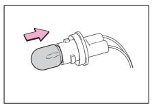
Install the bulb base to the light unit by inserting it and turning the bulb base clockwise
