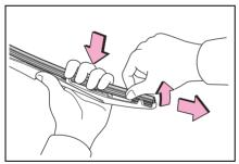
4 Remove the 2 metal plates from the old wiper insert and install them to the replacement wiper insert.
