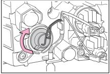
6 Align the grooves on the light unit with the claws, and insert the light unit straight so that the pin on the light unit fit into the hole.
