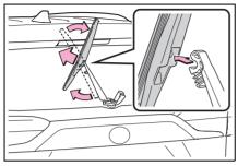
3 Pull the wiper insert out past the stopper on the wiper blade, and then continue to pull until it is completely removed.
