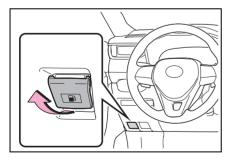
2 Turn the fuel tank cap slowly to open it and put it into the holder on the fuel filler door.
