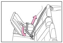
6 After installing the child restraint system, rock it back and forth to ensure that it is installed securely. (→P.58)
