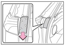
2 Remove the screws and remove the unit.
