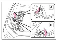
Engine compartment: Type B fuse box
