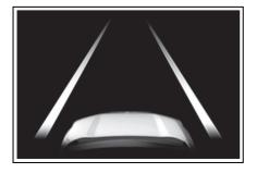
Indicates that the system is recognizing white (yellow) lines or a course\*. When the vehicle departs from its lane, the white line displayed on the side the vehicle departs from flashes orange.
