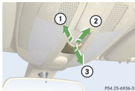
Roof panel switch
