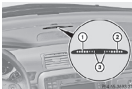
Front area warning indicators
