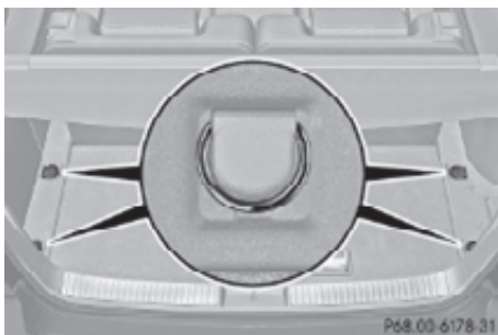
Cargo tie down rings, cargo compartment
