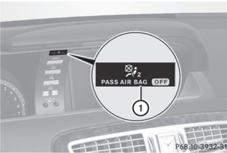
If the SmartKey has been removed from the ignition lock or is in position **0**, indicator lamp
