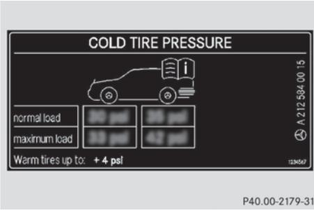
Tire pressure table for all approved tires installed at the factory (example)
