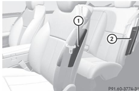
Front side impact air bags ① and rear side impact air bags ② are deployed next to the outer seat cushions.
