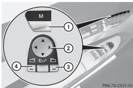
▶ Make sure that the vehicle is stationary and that the SmartKey is in position **2** in the ignition lock.
