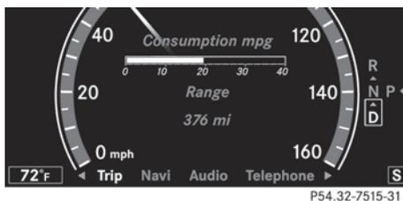
The approximate range which can be covered depends on the fuel level and your current driving style. If there is only a small amount of fuel left in the fuel tank, the display shows a vehicle being refueled instead of the range.
