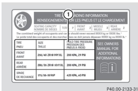
You will find recommended tire pressure specifications **1** for cold tires and for a fully loaded vehicle on the Tire and Loading Information placard. The tire pressure specifications apply to tires which are installed at the factory.
