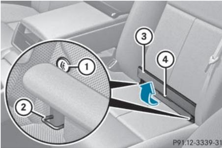
Installation instruction ① indicates the installation point of securing ring ②.
