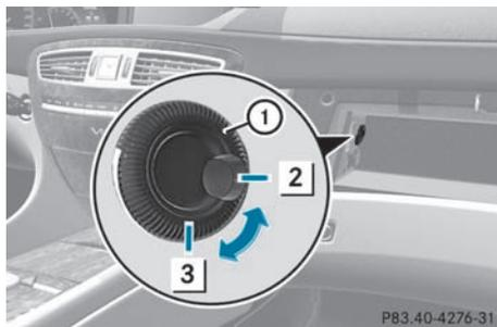
► **To open:** turn thumbwheel ① counter-clockwise from position ③ to position ②.
