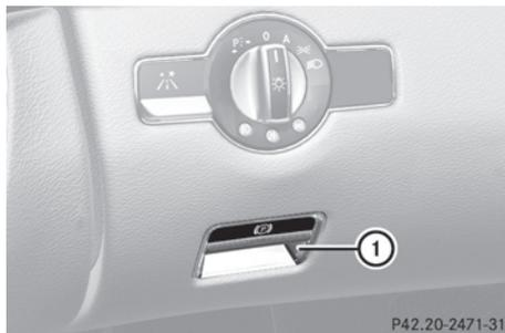
**Releasing the electric parking brake manually**
