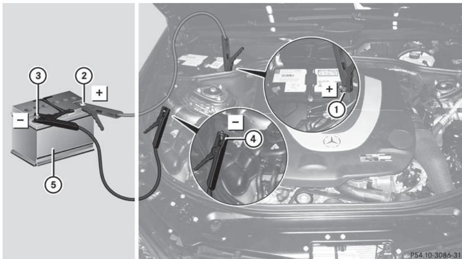
Position number ⑤ identifies the charged battery of the other vehicle or an equivalent jump-starting device.
