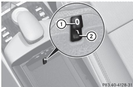
► **To switch the ventilation on/off:** push rocker switch down ② or up ①.
