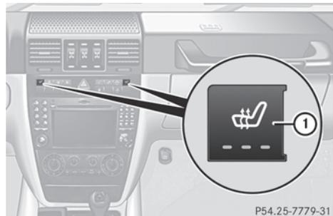
**i** The system automatically switches down from level **3** to level **2** after approximately five minutes.
