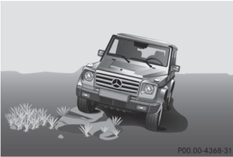
**!** Obstacles could damage the floor of the vehicle or components of the chassis. Ask passengers for guidance when driving over large obstacles. The passenger should always keep a safe distance from the vehicle when doing so in order to avoid injury as a result of unexpected vehicle movements. After driving off-road or over obstacles, check the vehicle for possible damage, especially to the underbody and the components of the chassis.
