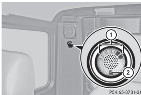
The warning display is divided into four yellow and two red segments ①. The ultrasonic backing up aid is ready for use when you hear a warning tone and segment ② lights up briefly.
