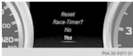
If you switch off the engine, the RACETIMER is reset to "0" after 30 seconds. All laps are deleted.
