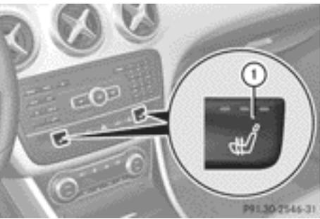
The three red indicator lamps in the button indicate the heating level you have selected. The system automatically switches down from level **3** to level **2** after approximately eight minutes. The system automatically switches down from level **2** to level **1** after approximately ten minutes. The system automatically switches off approximately 20 minutes after it is set to level **1**.
