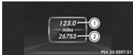
▶ Press and hold the
