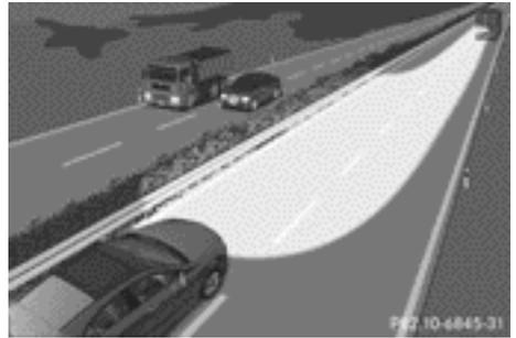
Motorway mode increases the range of the beam.
