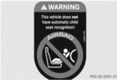
If the front-passenger seat of your vehicle does not have automatic child seat recognition, this is indicated by a special sticker. The sticker is affixed to the side of the dashboard on the front-passenger side. The sticker is visible when you open the front-passenger door.
