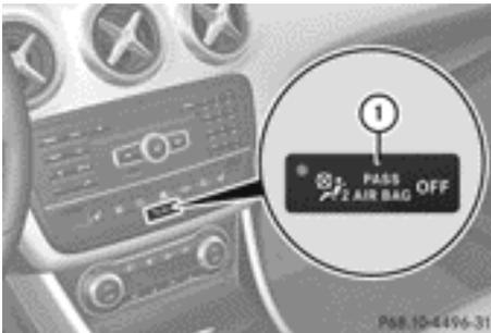
The sensor system for child restraint systems in the front-passenger seat detects whether a special Mercedes-Benz child seat with a transponder for automatic child seat recognition has been fitted. In this case,
