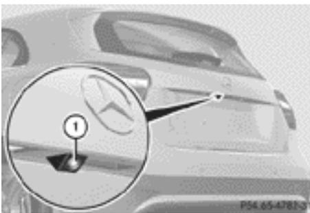
Reversing camera ① is in the boot lid handle. The reversing camera extends, when it is activated.
