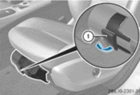
The fire extinguisher is located underneath the front of the driver's seat.
