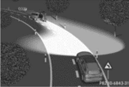
The active light function is a system that moves the headlamps according to the steering movements of the front wheels. In this way, relevant areas remain illuminated while driving. This allows you to recognise pedestrians, cyclists and animals.
