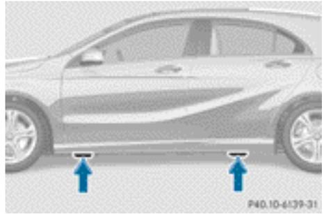
The jacking points are located just behind the front wheel arches and just in front of the rear wheel arches (arrows).
