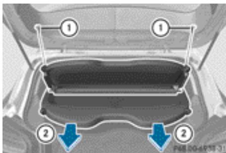
**!** The maximum load which may be placed on the rear shelf is 2.5 kg.
