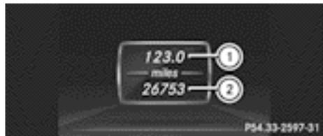
▶ Press and hold the
