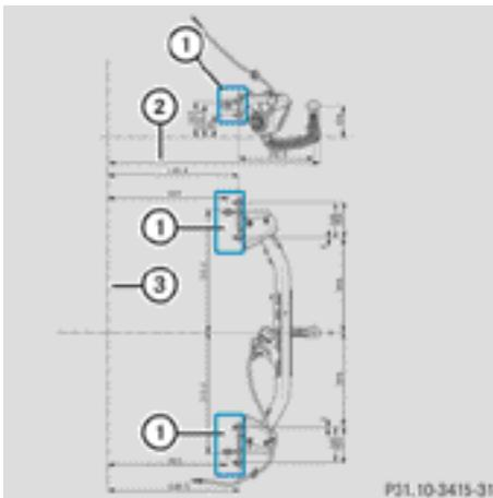
Example: anchorage points for the trailer tow hitch
