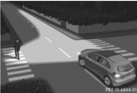
The cornering light function improves the illumination of the road over a wide angle in the direction you are turning, enabling better visibility in tight bends, for example. The cornering light function can only be activated when the dipped-beam headlamps are switched on.
