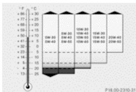
Viscosity describes the flow characteristics of a fluid. If an engine oil has a high viscosity rating, it flows slowly; the lower the viscosity, the faster it flows.
