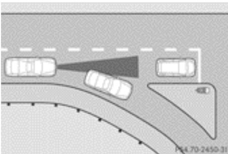
DISTRONIC PLUS does not brake for obstacles or stationary vehicles. If, for example, the
