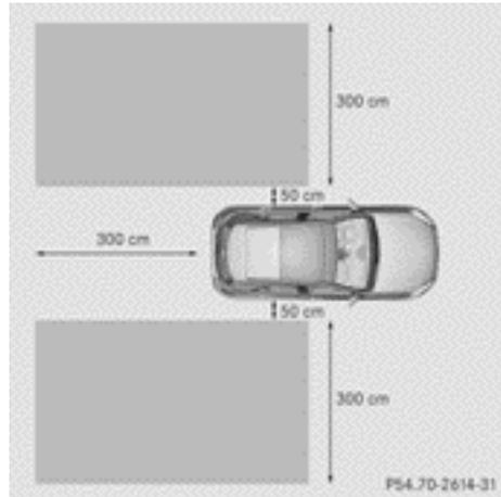
Blind Spot Assist monitors the area up to 3.0 m behind your vehicle and directly next to your vehicle, as shown in the diagram. For this purpose, Blind Spot Assist uses radar sensors in the rear bumper.
