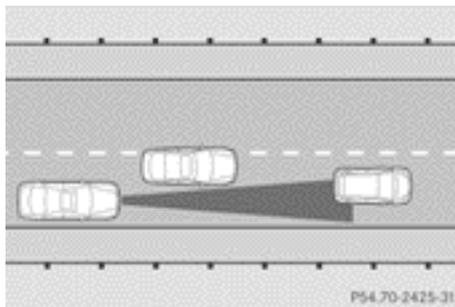
DISTRONIC PLUS may not detect vehicles which are not driving in the middle of their lane. The distance to the vehicle in front will be too short.
