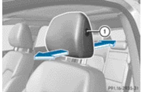
This function allows you to adjust the distance between the head restraint and the back of the head.
