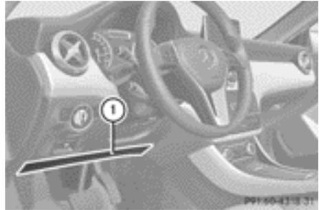
Driver's kneebag ① deploys under the steering column. The driver's kneebag is triggered together with the front airbag. The driver's kneebag is designed to operate together with the front airbag in frontal impacts if certain thresholds are exceeded. The driver's kneebag operates best in conjunction with correctly positioned and fastened seat belts.
