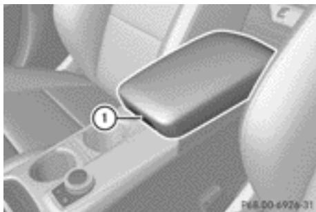
► **To open:** on vehicles with moveable armrests, make sure that the armrest is in the rearmost position.
