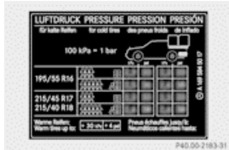
If a tyre size precedes a tyre pressure, the following tyre pressure information is only valid for that tyre size.
