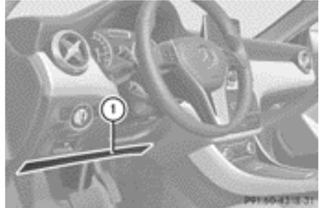
Driver's kneebag ① deploys under the steering column. The driver's kneebag is triggered together with the front airbag. The driver's kneebag is designed to operate together with the front airbag in frontal impacts if certain thresholds are exceeded. The driver's kneebag operates best in conjunction with correctly positioned and fastened seat belts.
