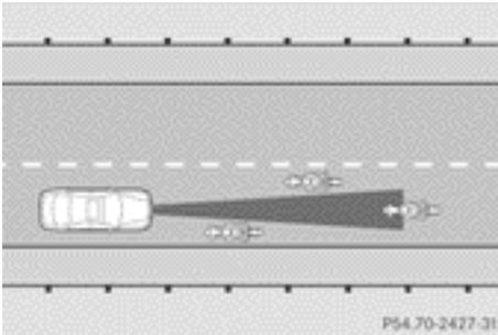
DISTRONIC PLUS has not yet detected the vehicle in front on the edge of the carriage-way, because of its narrow width. The distance to the vehicle in front will be too short.
