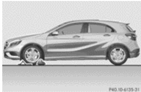
Securing the vehicle on level ground
