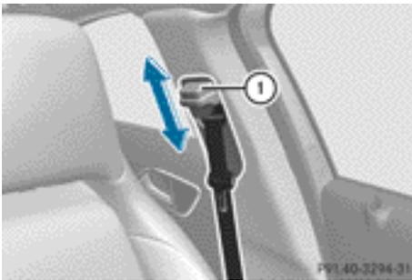
You can adjust the belt height for the front seats. Adjust the belt to a height that allows the upper part of the seat belt to be routed across the centre of your shoulder.
