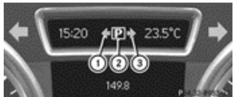
Example: detected parking space for a vehicle with automatic transmission
