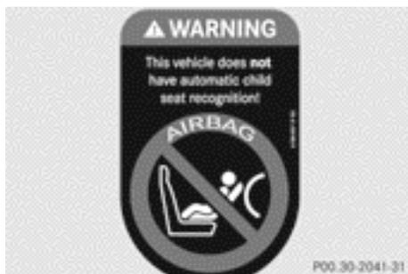
If the front-passenger seat of your vehicle does not have an air bag deactivation system, this is indicated by a special sticker. The sticker is affixed to the side of the dashboard on the front-passenger side. The sticker is visible when you open the front-passenger door.
