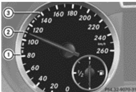
DISTRONIC PLUS displays in the speedometer
