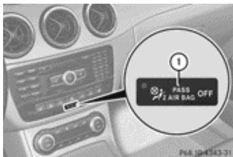
The sensor system for the air bag deactivation system detects whether a special Mercedes-Benz child seat with a transponder for the air bag deactivation system has been installed. In this case,
