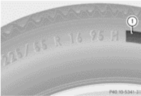
In addition to the load bearing index, load index ① may be imprinted after the letters that identify speed index ⑥ (▷ page 313) on the sidewall of the tire.
