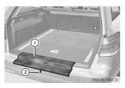
The EASY-PACK rear sill protector is attached to the underside of the EASY-PACK folding cargo compartment floor by means of magnets. It is designed to prevent clothing becoming stained and the paintwork being scratched when loading.
