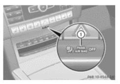
If the SmartKey is removed from the ignition lock or is in position 0, PASSENGER AIR BAG OFF indicator lamp (1) does not light up.
