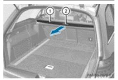
► To extend: pull cargo compartment cover (1) back by grab handle (2) and clip it into the retainers on the left and right.
