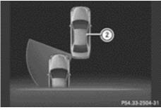
If Active Blind Spot Assist detects a risk of a lateral collision in the monitoring range, a course-correcting brake application is carried out. This is meant to assist you in avoiding a collision.
