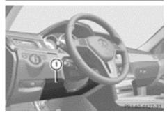
Driver's knee bag (1) deploys under the steering column. It is deployed together with the front air bags. The driver's knee bag is designed to operate together with the front
