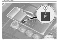
▶ When the vehicle is stationary, press P button (1).
