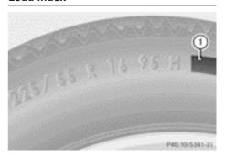
In addition to the load bearing index, load index ① may be imprinted after the letters that identify speed index ⑥ on the sidewall of the tire ( $\triangleright$  page 389).
