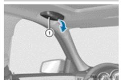
There is a compartment to stow eyeglasses in the headliner on the driver's side.
