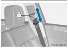
You can adjust the seat belt height on the front seats. **Wagon:** you can also adjust the belt height on the outer rear seats. Adjust the belt to a height that allows the upper part of the seat belt to be routed across the center of your shoulder.
