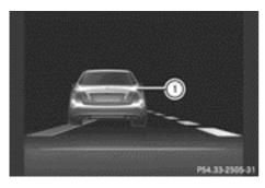
If you leave your lane, under certain circumstances the vehicle will brake briefly on one side. This is meant to assist you in bringing the vehicle back to the original lane. If a lane-correcting brake application occurs, display (1) appears in the multifunction display.
