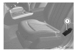
Pelvis air bags ① enhance the level of protection of the vehicle occupants on the side of the vehicle on which the impact occurs.
