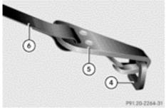
The Top Tether anchorages are attached to the rear of the rear seat backrests.
