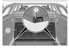
You must remove the seat cushion if you wish to lift the trunk floor, e.g. if the vehicle has a flat tire.
