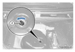
► Turn DEF filler cap ② counter-clockwise and open it. Filler cap ② is secured with a plastic strip.
