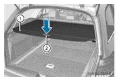
► To retract: unhook cargo compartment cover (1) from the retainers on the left and right and guide it forwards by grab handle (2) until it is fully retracted.
