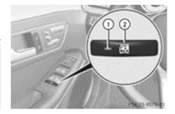
▶ To activate/deactivate: press button ②. If indicator lamp (1) is lit, operation of the rear side windows is disabled. Operation is only possible using the switches in the driver's door. If indicator lamp (1) is off, operation is possible using the switches in the rear compartment.
