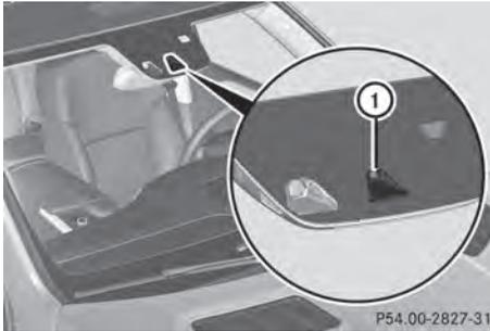
Active Lane Keeping Assist monitors the area in front of your vehicle by means of camera ① at the top of the windshield. Active Lane Keeping Assist detects lane markings on the road and warns you before you leave your lane unintentionally. If you do not react to the warning, a lane-correcting application of the brakes can bring the vehicle back into the original lane.
