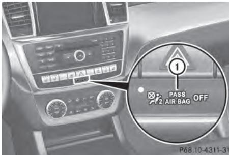
If the SmartKey has been removed from the ignition lock or is in position **0**, the
