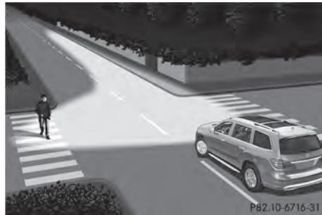
The cornering light function improves the illumination of the road over a wide angle in the direction you are turning, enabling better visibility in tight bends, for example. It can only be activated when the low-beam headlamps are switched on.
