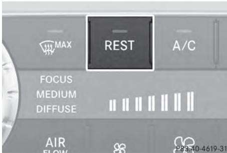
It is possible to make use of the residual heat of the engine to continue heating the stationary vehicle for up to 30 minutes after the engine has been switched off. The heating time depends on the temperature that has been set.
