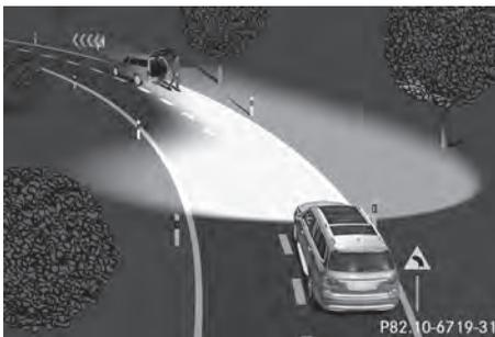
The active light function is a system that moves the headlamps according to the steering movements of the front wheels. In this way, relevant areas remain illuminated while driving. This allows you to recognize pedestrians, cyclists and animals.
