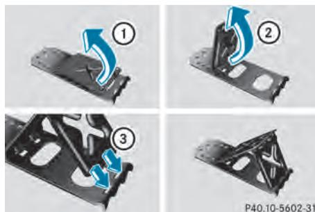
If your vehicle is equipped with a wheel chock, it can be found in the tire-change tool kit (▷ page 382).
