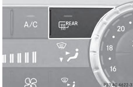
The rear window defroster has a high current draw. You should therefore switch it off as soon as the rear window is clear. Otherwise, the rear window defroster switches off automatically after several minutes.
