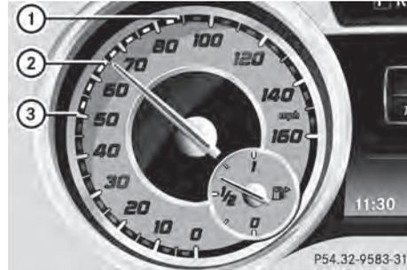
Example: DISTRONIC PLUS displays in the speedometer
