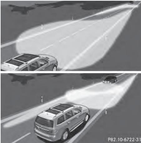
You can use this function to set the headlamps to change between low beam and high beam automatically. The system recognizes vehicles with their lights on, either approaching from the opposite direction or traveling in front of your vehicle, and consequently switches the headlamps from high beam to low beam.
