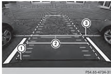
① Red guide line at a distance of approximately 10 in (0.25 m) from the rear of the vehicle
