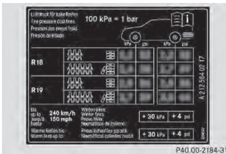
Some tire pressure tables show only the rim diameters instead of the full tire size, e.g. **R18**. The rim diameter is part of the tire size and can be found on the tire sidewall (▷ page 417).
