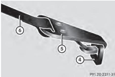
Top Tether provides an additional connection between a child restraint system, secured with a LATCH-type (ISOFIX) child seat mount, and the rear seat. This helps reduce the risk of injury even further.
