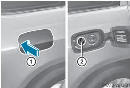
The fuel filler flap is unlocked or locked automatically when you open or close the vehicle with the SmartKey or with KEYLESS-GO.
