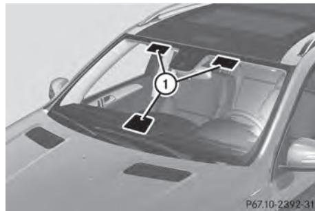
The infrared reflecting glass prevents the vehicle interior from becoming too hot. It also blocks radio waves up into the gigahertz range.
