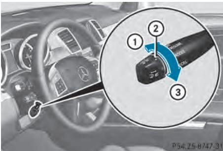
You can set the specified minimum distance for DISTRONIC PLUS by varying the time span between one and two seconds. With this function, you can set the minimum distance that DISTRONIC PLUS keeps to the vehicle in front, dependent on vehicle speed. You can
