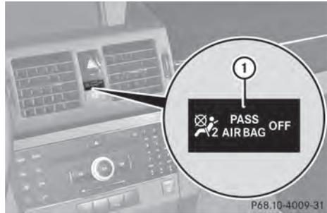
If the SmartKey has been removed from the ignition lock or is in position **0**, the
