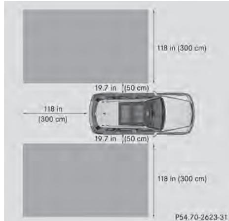
Blind Spot Assist monitors the area up to 10 ft (3m) behind your vehicle and directly next to your vehicle, as shown in the diagram. If the lanes are narrow, vehicles driving in the lane beyond the lane next to your vehicle may be indicated, especially if the vehicles are not driving in the middle of their lane. This may be the case if there are vehicles driving at the inner edge of their lanes.
