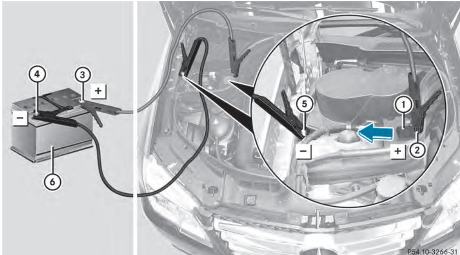
Position number ⑥ identifies the charged battery of the other vehicle or an equivalent jump-starting device.
