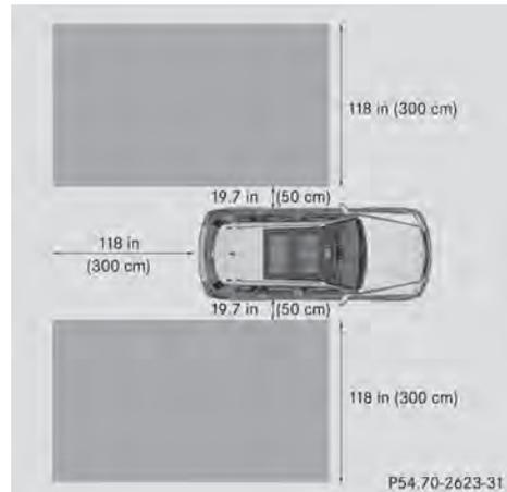
Active Blind Spot Assist monitors the area up to 10 ft (3 m) behind your vehicle and directly next to your vehicle, as shown in the diagram. For this purpose, Active Blind Spot Assist uses radar sensors in the rear bumper.
