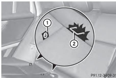
Installation instructions (1) indicate the installation location of securing rings (2).
