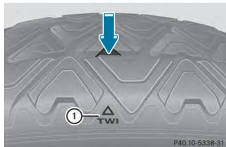
Bar indicator ① for tread wear is integrated into the tire tread.
