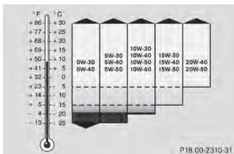
Viscosity describes the flow characteristics of a fluid. If an engine oil has a high viscosity,
