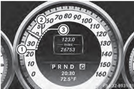
When DISTRONIC PLUS is activated, one or two segments ② in the set speed range light up.
