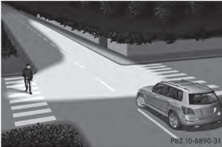
The cornering light function improves the illumination of the road over a wide angle in the direction you are turning, enabling better visibility in tight bends, for example. The cornering light function can only be activated when the low-beam headlamps are switched on.
