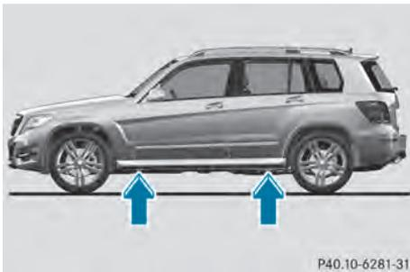
The jacking points are located just behind the wheel housings of the front wheels and just in front of the wheel housings of the rear wheels (arrows).
