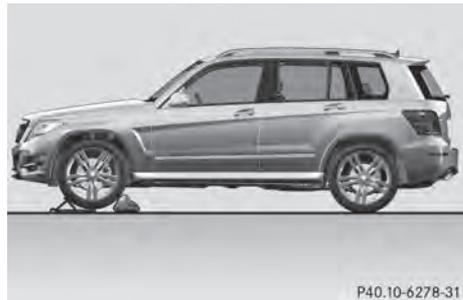
Securing the vehicle on level ground
