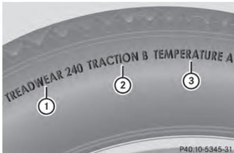
Uniform Tire Quality Grading Standards are U.S. government specifications. Their purpose is to provide drivers with uniform reliable information on tire performance data. Tire manufacturers have to grade tires using three performance factors: tread wear ①, tire traction ② and heat resistance ③. All tires sold in North America are provided with the corresponding quality class mark on the sidewall of the tire, even though these regulations do not apply to Canada.
