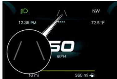
Lane Markings Not Detected
