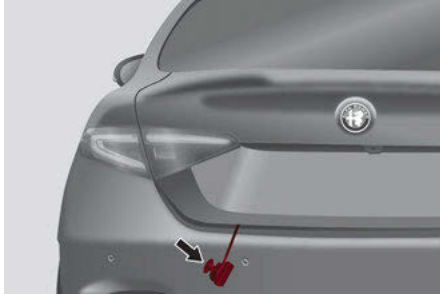
Manual Release Cord Shown With Trunk Closed
