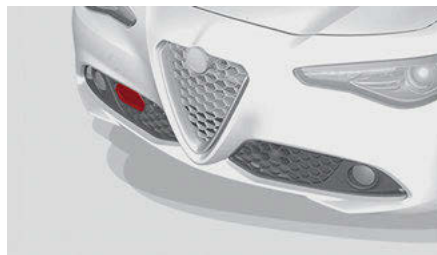
Front Fascia/Bumper Radar Location
