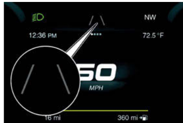
Lane Markings Not Detected
