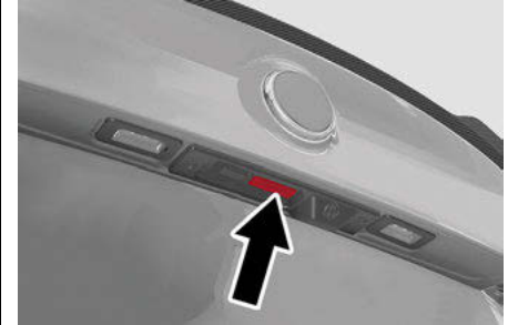
Exterior Trunk Lid Release Switch (Vehicles With Passive Entry)
