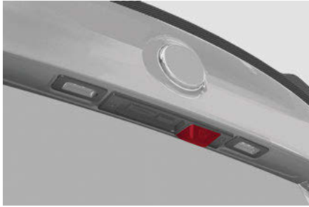
Rear Back Up Camera Location Camera Activation/Deactivation
