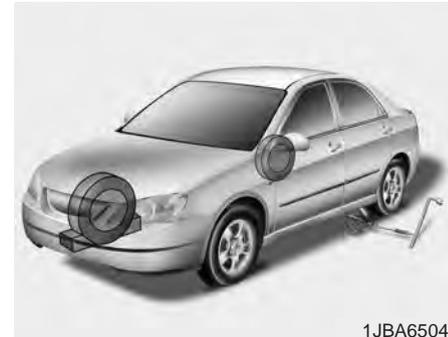
4. Remove the wheel lug nut wrench, jack, jack handle, and spare tire from the vehicle.
