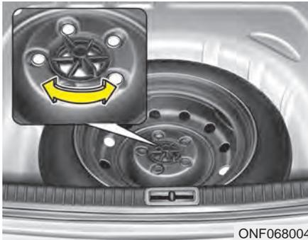
Turn the tire hold-down wing bolt counterclockwise.
