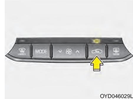
The air intake control is used to select outside (fresh) air position or recirculated air position.
