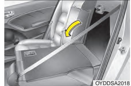
5. Pull the lock release lever (1) and fold the rear seatback forward and down firmly.
