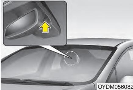
The Lane Keeping Assist System detects lane markers on the road, and assists the driver's steering to help keep the vehicle between lanes.
