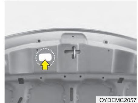
The refrigerant label is located on the underside of the hood.
