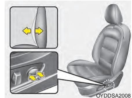
Press the front portion of the switch to increase support, or the rear portion of the switch to decrease support.
