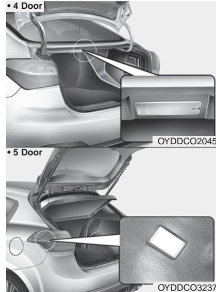
The luggage lamp comes on as long as the trunk lid (tailgate) is open. To prevent unnecessary charging system drain, close the trunk lid (tailgate) securely after using the luggage room.
