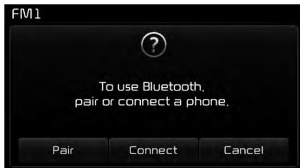
If *Bluetooth*® Wireless Technology devices are paired but none are currently connected, pressing the [PHONE] button or the [CALL] button on the steering wheel control displays the following screen. Press the [Pair] to pair a new device or press the [Connect] to connect a previously paired device.
