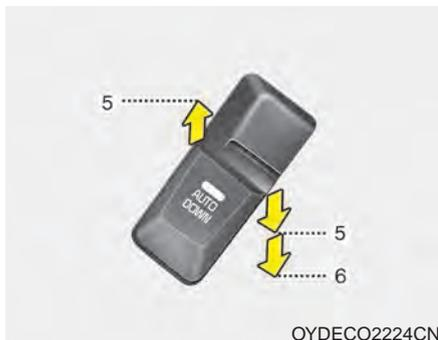
Pressing the power window switch momentarily to the second detent position (6) completely lowers the driver's window even when the switch is released. To stop the window at the desired position while the window is in operation, momentarily pull up the switch to the opposite direction of the window movement.
