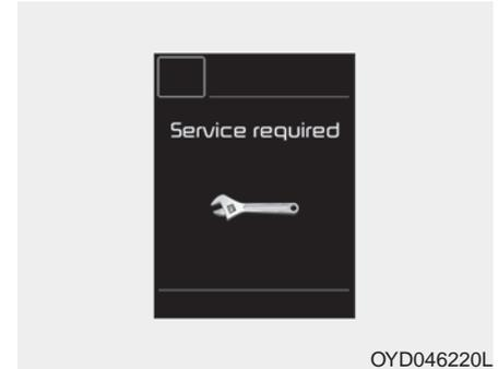
If you do not have your vehicle serviced according to the already inputted service interval, "Service required" message is displayed for several seconds each time you set the ignition switch or Engine Start/Stop Button to the ON position.
