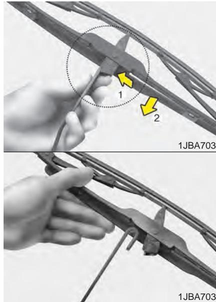
2. Compress the clip (1) and slide the blade assembly downward (2).
