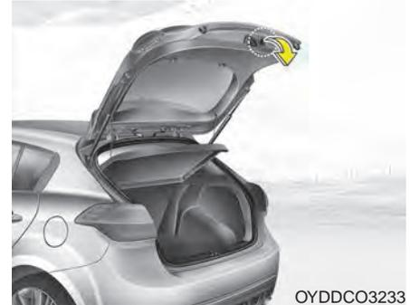
To close the tailgate, lower and push down the tailgate firmly. Make sure that the tailgate is securely latched.
