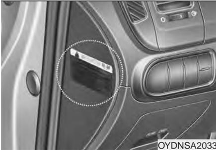
Air bag warning labels, some required by the U.S. National Highway Traffic Safety Administration (NHTSA), are attached to alert the driver and passengers of potential risks of the air bag system.
