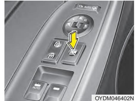
The driver can disable the power window switches on the rear passengers' doors by pressing the power window lock switch to the lock position (pressed).
