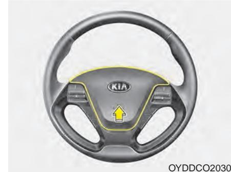
To sound the horn, press the horn symbol on your steering wheel. Check the horn regularly to be sure it operates properly.
