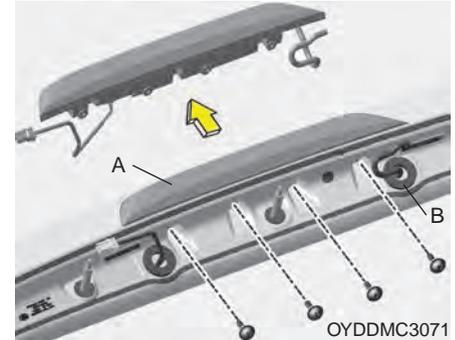
5. Remove the high mounted stop lamp assembly (A) after loosening the nuts and washer nozzle (B).
