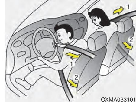
Your vehicle is equipped with driver's and front passenger's pre-tensioner seat belts.
