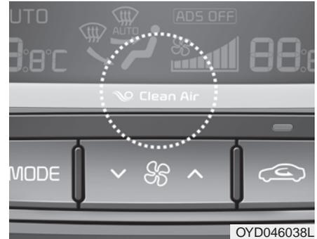
When the ignition switch is in the ON position, the clean air function turns on automatically.
