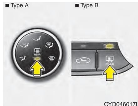
The defroster heats the window to remove frost, fog and thin ice from the interior and exterior of the rear window, while the engine is running. To activate the rear window defroster, press the rear window defroster button located in the center fascia switch panel. The indicator on the rear window defroster button illuminates when the defroster is on.
