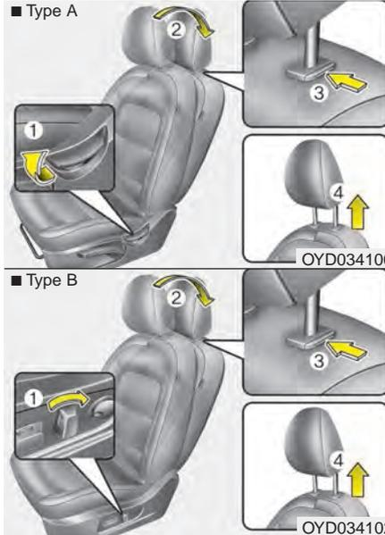
3. Press the headrest release button (3) while pulling the headrest up (4).
