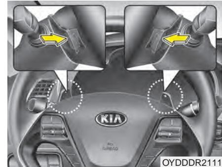
The paddle shifter is available when the shift lever is in the D position or the sport mode.
