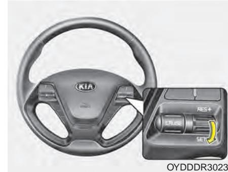
3. Move the lever down (to SET-), and release it at the desired speed. The SET indicator light in the instrument cluster will illuminate. Release the accelerator pedal at the same time. The desired speed will automatically be maintained.
