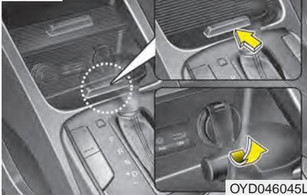
The power outlet is designed to provide power for mobile telephones or other devices designed to operate with vehicle electrical systems. The devices should draw less than 12V, 15A with the engine running.
