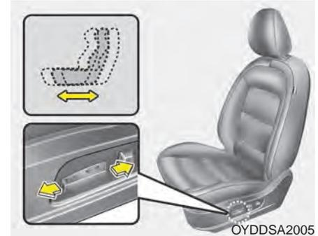
Push the control switch forward or backward to move the seat to the desired position. Release the switch once the seat reaches the desired position.
