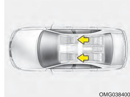
The driver's and front passenger's seats are equipped with a headrest for the occupant's safety and comfort. The headrest not only provides comfort for the driver and front passenger, but also helps protect the head and neck in the event of a collision.
