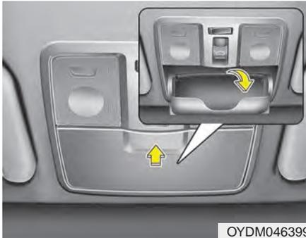
To open the sunglasses holder, press the cover and the holder will slowly open. Place your sunglasses with the lenses facing out. To close the sunglasses holder, push it up. Do not open the sunglasses holder while the vehicle is moving. The rear view mirror of the vehicle can be blocked by an open sunglasses holder.
