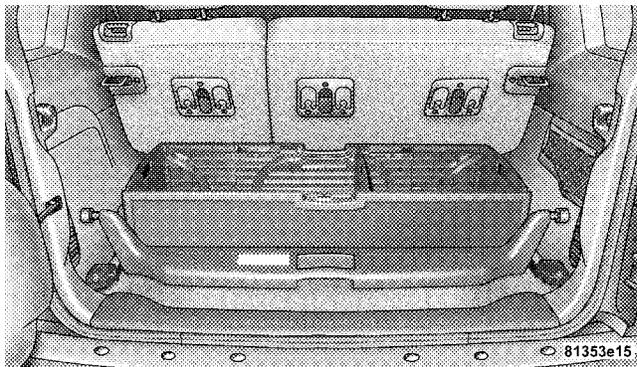
2. Lift up on the storage compartment dividers and lock into place.
