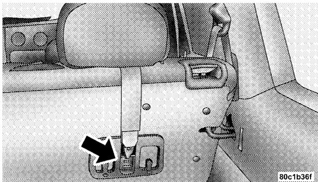
Many, but not all restraint systems will be equipped with separate straps on each side, with each having a hook or connector for attachment to the lower anchorage and a means of adjusting the tension in the strap. Forward-facing toddler restraints and some rear-facing infant
