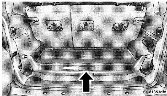
2. Place the rear corners of the cargo organizer into the supports located on the rear trim panel. Press down on the back of the cargo organizer to lock it into place.
