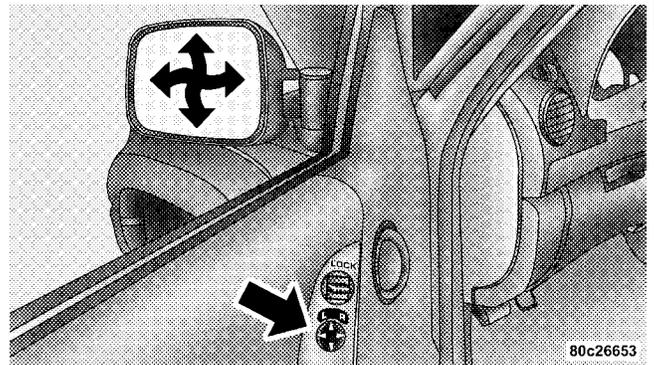
**Heated Remote Control Mirrors — If Equipped**
