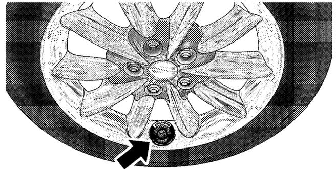
7. Repeat step 6 working clockwise around the vehicle (Left Front, Right Front, Right Rear, Left Rear, Spare) until all five TPM sensor positions are trained.
