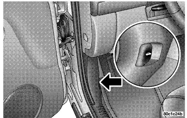
Then, reach under the hood and slide the safety latch to the right and lift the hood.
