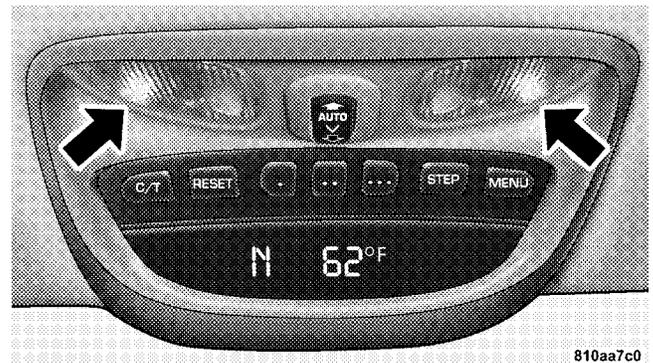
The dome/reading lights illuminate when a door or the swing gate is opened or when the interior lights are turned on by rotating the dimmer control located on the multi-function lever.
