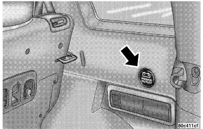
The rear power outlet is a direct feed from the battery so it receives power whether the ignition is in the ON or OFF position.
