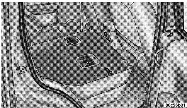
**NOTE:** When lifting up on the release handle, the seatback will release easier if you do not pull forward on the seatback; only lift up on the release handle until the seatback disengages, then fold the seat forward.
