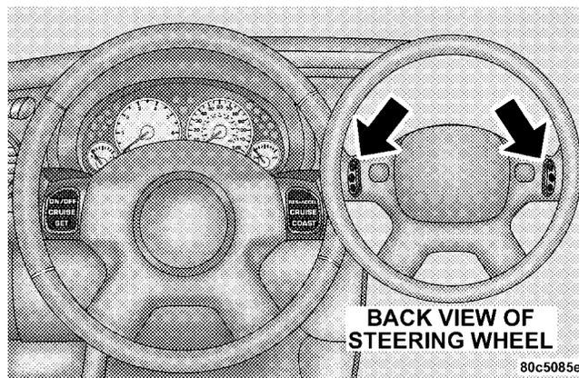
The right hand control is a rocker type switch with a push-button in the center and controls the volume and mode of the sound system. Pressing the top of the rocker switch will increase the volume and pressing the bottom of the rocker switch will decrease the volume.
