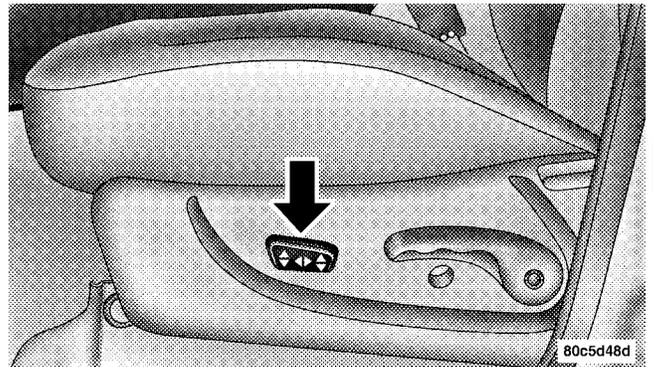
This seat also has a manual recline lever located just to the rear of the power seat switch. Pull up on the lever to recline the seat.
