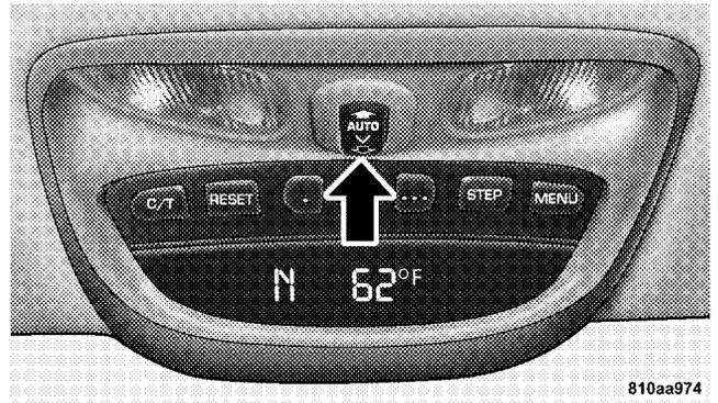
Press and hold the “V” button in the center of the sunroof switch to open the vent. The sunroof can be stopped at any position between closed and full vent. To close the sunroof from the vent position, press and hold the switch forward. Releasing the switch will stop the movement of the sunroof and the sunroof will remain in the partial vent position until the switch is pushed forward again.
