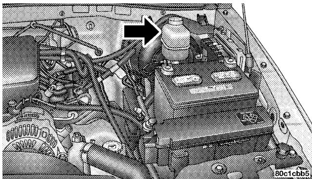
Be sure to clean the top of the master cylinder area before removing the cap. If necessary, add fluid to bring the fluid level up to the requirements described on the brake fluid reservoir. With disc brakes, fluid level can be expected to fall as the brake pads wear. However, low fluid level may be caused by a leak and a checkup may be needed.
