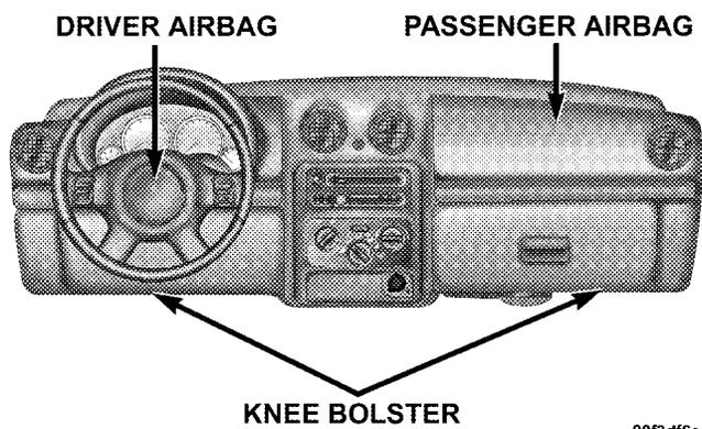
This vehicle has airbags for both the driver and right front passenger as a supplement to the seat belt restraint systems. The driver's front airbag is mounted in the steering wheel. The passenger side airbag is mounted in the instrument panel, above the glove compartment. The words SRS/AIRBAG are embossed on the airbag covers.
