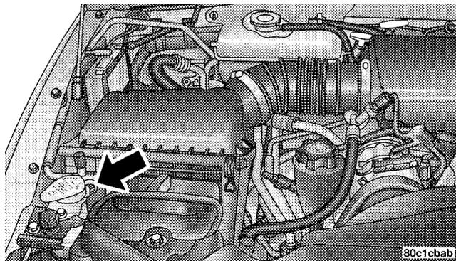
The fluid reservoir for the windshield washers and the rear window washer is shared. It is located in the front of the engine compartment on the passenger side and
