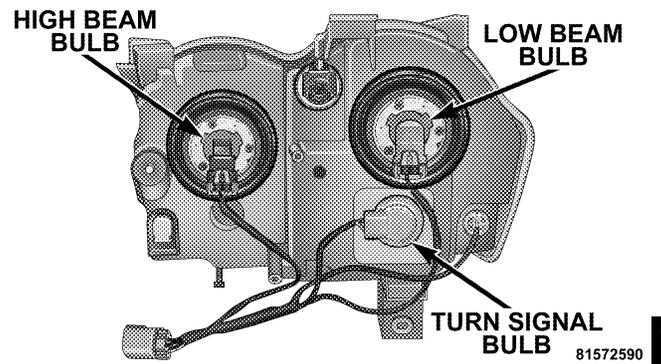
4. Disconnect the electrical connector and replace the bulb.
