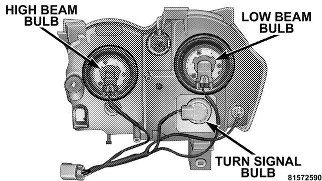
4. Disconnect the electrical connector and replace the bulb.
