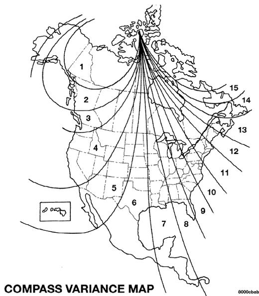
To set the variance: Turn the ignition ON and set the display to "Compass/Temperature." Press the C/T button approximately 5 to 10 seconds. The last variance zone number will be displayed. Press the STEP button to select the new variance zone and press the RESET button to resume normal operation.
