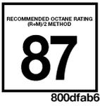
All engines (except 5.7L engines) are designed to meet all emissions regulations and provide excellent fuel economy and performance when using high quality unleaded "regular" gasoline having an octane rating of 87. The use of premium gasoline is not recommended. Under normal conditions, the use of premium gasoline will not provide a benefit over high quality regular gasolines, and in some circumstances may result in poorer performance.
