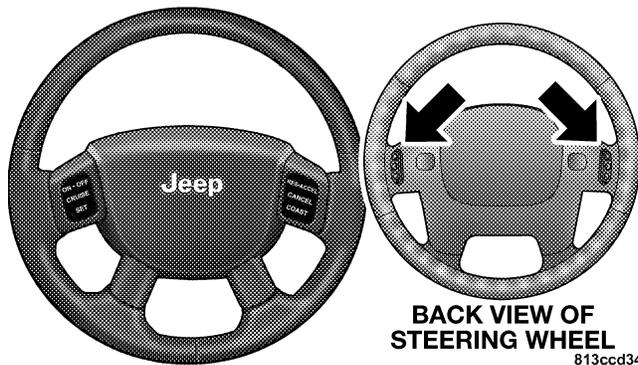
The right hand control is a rocker type switch with a push-button in the center and controls the volume and mode of the sound system. Pressing the top of the rocker
