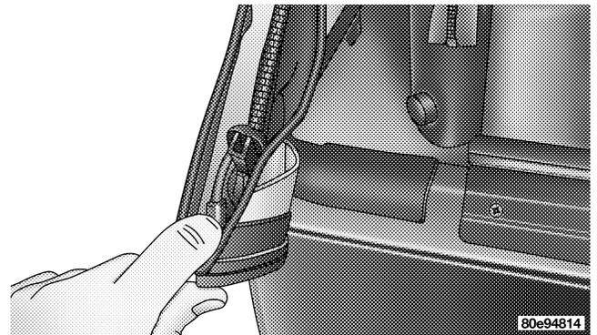
12. Zip in the rear window beginning from the left using both zipper ends. Run the upper zipper around the window leaving the lower zipper at the start.
