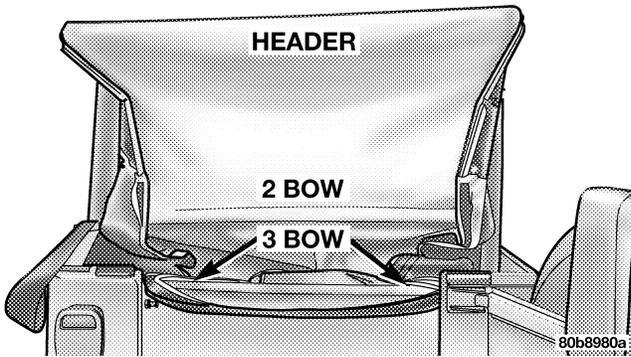
12. Move to the side of the vehicle and pull the side bow forward and down. You will see the 3 bow rise from the rear of the vehicle.
