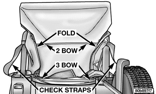
14. Tuck the top material between the 2 bow and the header.
