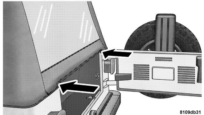
13. Tuck the lower retainers on the rear window under the tailgate clips.
