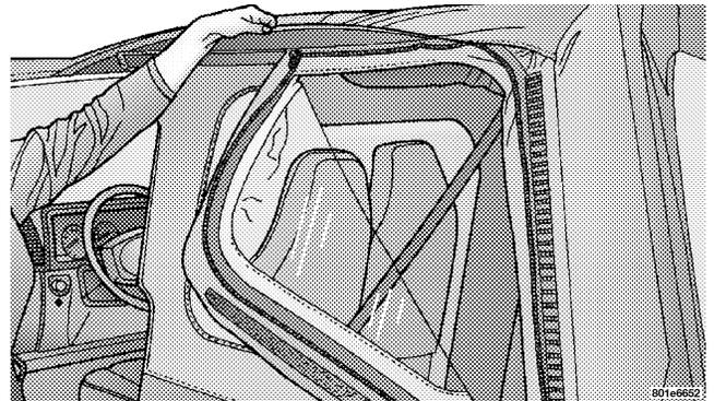
10. Tuck the bottom retainer of the quarter window into the bottom retainer, beginning from the rear and working to the front of the vehicle. Repeat this step for the other side.
