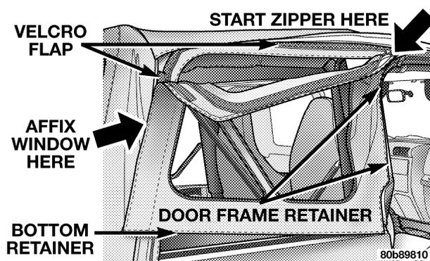
20. Tuck in the bottom retainers on the quarter windows into the bodyside retainer, beginning from the rear and working to the front of the vehicle. Repeat this step for the other side.
