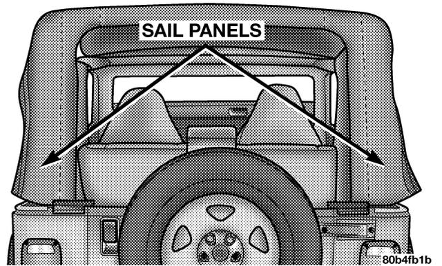
7. Align the sail panel retainer to the edge of the bodyside retainer at the rear. Tuck the sail panel into the bodyside retainer beginning from the rear and working to the corner. Tuck the retainer around the corner and continue forward.
