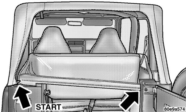
13. Tuck the retainer bar into the tailgate clips.
