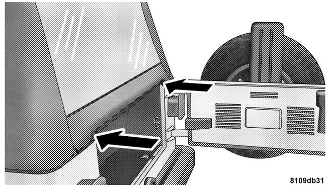
24. Tuck the lower retainers on both sides of the rear window under the tailgate clips. Reinstall the left sail panel if it was untucked to get the rear window zipper started.
