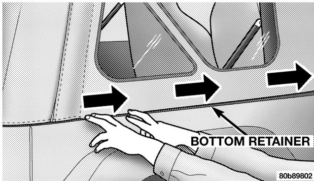
11. To assist in getting the zipper started, lay the retainer bar inside the vehicle on the wheel wells and uninstall half of the left sail panel from the bodyside retainer beginning at the tailgate to expose zipper ends.
