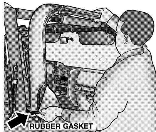
3. Slide door frame forward until the pin holes in the top line up with the holes in the side bar. Screw in the knobs and tighten, beginning with the front knob. Repeat procedures on the other side.
