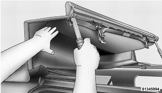
5. Locate strap to secure the header to the sport bar. Wrap strap around sport bar and hook to header and tighten.
