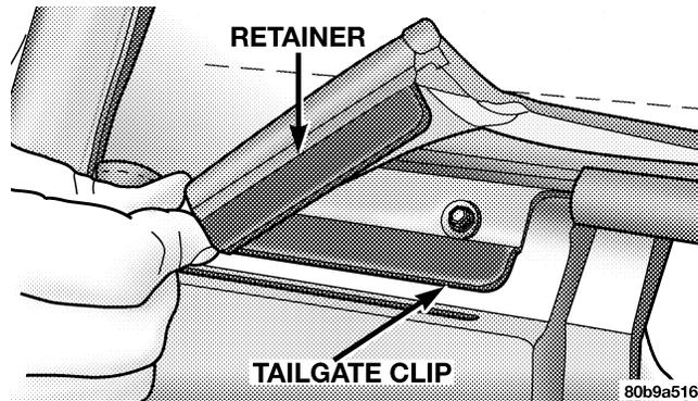
15. Tuck the drip rail retainers into the door frame slot above the door on both sides.
