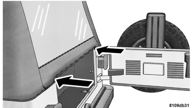
14. Tuck the lower retainers of the rear window under the tailgate clips. Reinstall the left corner if it was untucked to get the rear window zipper started.
