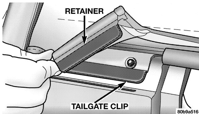
14. Reinstall the corner of the sail panel that was untucked to get the rear window zipper started.
