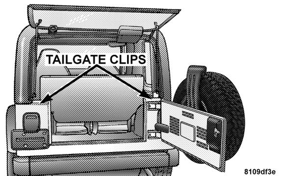
6. Pull the retainer bar straight out from the tailgate clips.
