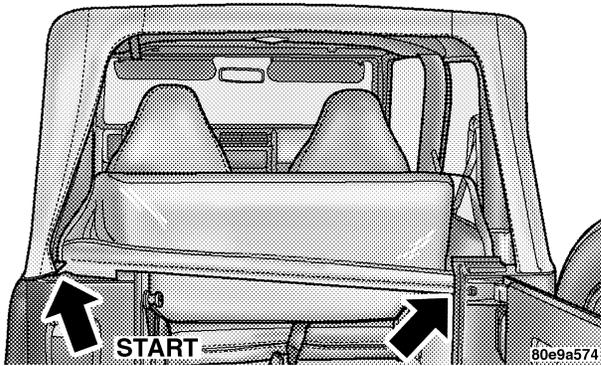
12. Tuck the retainer bar into the upper portion of the tailgate clips.
