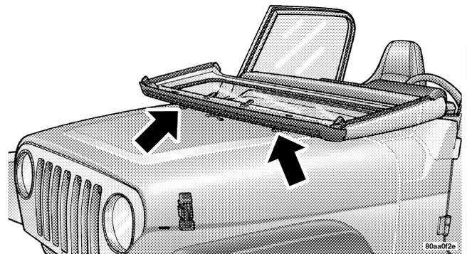
9. Secure the windshield by passing the remaining cinch strap, found in the glove box, through the footman hoop on the center of the hood and on the center of the windshield frame. Tighten the strap to secure the windshield in place.
