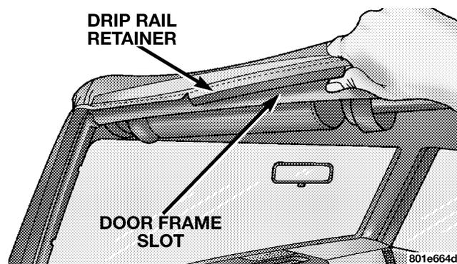
16. Fully engage the header latch.
