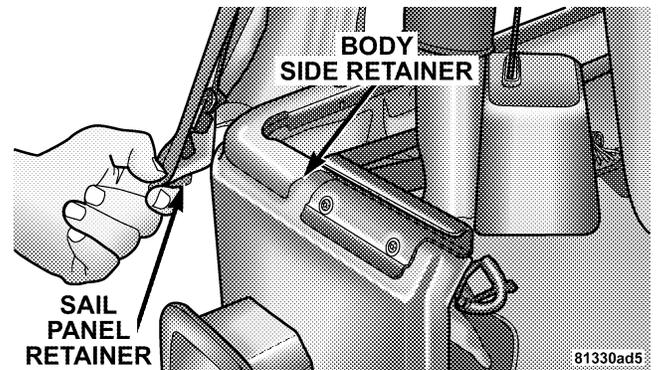
8. To install the quarter window, affix the rear corner of the window temporarily to the Velcro®. Start and zip the zipper only about 1 inch (2.5 cm). At this time it is necessary to tuck in the door frame retainer.
