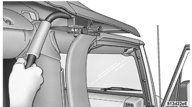
12. As you begin to lower the top, wrap the sail panels so that they rest on the roof of the vehicle.
