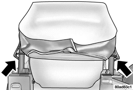
13. Make sure the sides of the top are folded inward as the top continues to fold, and check straps are clear of the vehicle. Tuck the top between the 2 bow and 2-1/2 bow and 2-1/2 bow and 3 bow as it folds.
