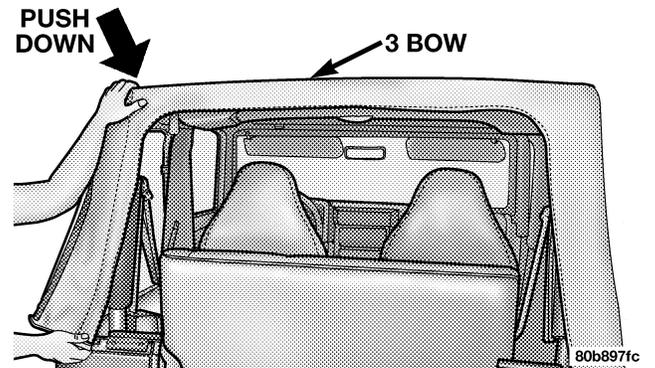
8. To install the quarter windows, affix the upper rear corner of the window temporarily using the Velcro®. Next, start the zipper about 1 inch (2.5 cm) at the upper forward corner of the window. At this time it is necessary to tuck in the door frame retainer.
