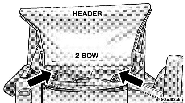
14. After the top is folded down, ensure that the drip rail retainers are tucked in inward as shown. This is to avoid unnecessary wear to the fabric.
