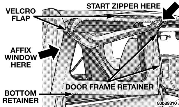
9. After the door frame retainer has been completely tucked in, finish zipping in the window. Then affix the Velcro® flaps around the window.
