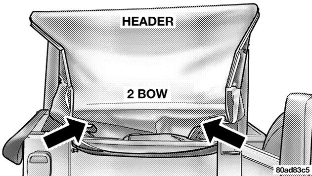
15. After the top is folded down, ensure that the drip rail retainers are tucked in inward as shown. This is to avoid unnecessary wear to the fabric.
