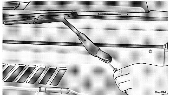
7. Remove the black round headed windshield Torx® head screw on each side of the base of the windshield.
