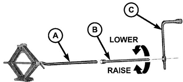
4. Locate the jack as shown. For the front axle, place it under the front lower control arm as shown. For the rear axle, place it under the axle near the wheel to be changed. Ensure the jack is closest to the inside of the wheel when jacking on the rear axle. **Do not raise the vehicle until you are sure the jack is fully engaged.**
