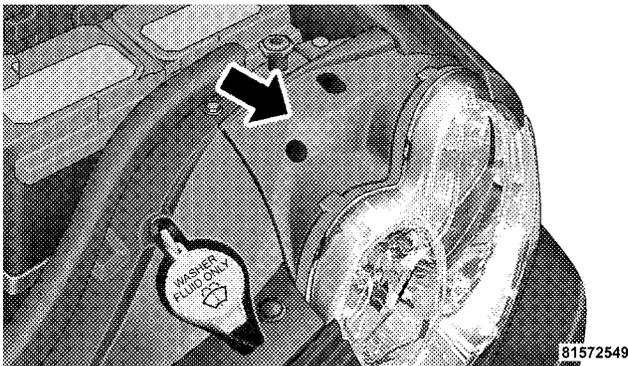
3. Turn the low or high beam bulb 1/4 turn counter clockwise to remove from housing.
