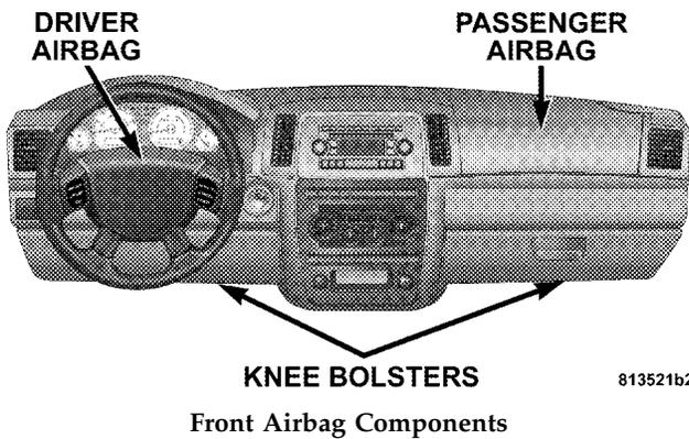
This vehicle has airbags for both the driver and right front passenger as a supplement to the seat belt restraint systems. The driver's front airbag is mounted in the steering wheel. The passenger side airbag is mounted in the instrument panel, above the glove compartment. The words SRS/AIRBAG are embossed on the airbag covers.
