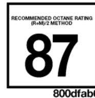
Your engine is designed to meet all emissions regulations and provide excellent fuel economy and performance when using high quality unleaded gasoline having an octane rating of 87. The use of premium gasoline is not recommended. The use of
