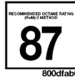
Your engine is designed to meet all emissions regulations and provide excellent fuel economy and performance when using high quality unleaded gasoline having an octane rating of 87. The use of premium gasoline is not recommended. The use of premium gasoline will provide no benefit over high quality regular gasoline, and in some circumstances may result in poorer performance.
