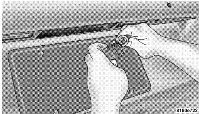
**Removing Socket from Lamp**
