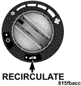
Use this button to choose between outside air intake or recirculation of the air inside the vehicle. A lamp will illuminate when you are in recirculate mode. Only use the recirculate mode to temporarily block out any outside odors, smoke, or dust and to cool the interior rapidly upon initial start up in very hot or humid weather.
