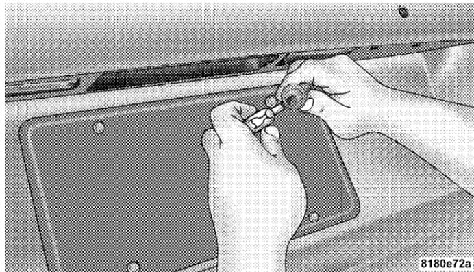
**Removing Bulb From Socket**
