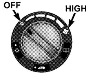
Use this control to regulate the amount of air forced through the system in any mode you select. The fan speed increases as you move the control to the right from the OFF position.
