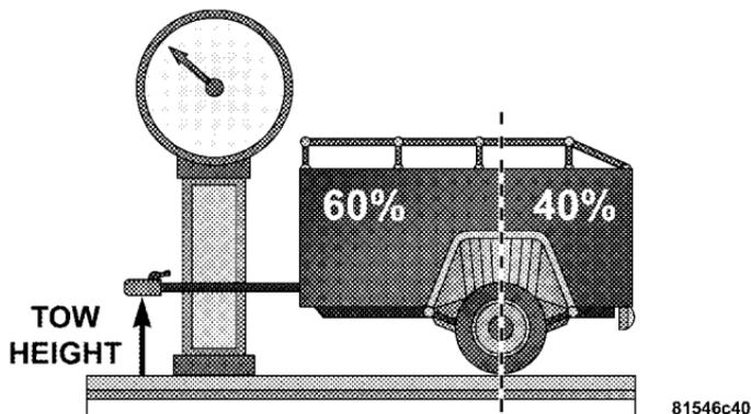
Consider the following items when computing the weight on the rear axle of the vehicle:
