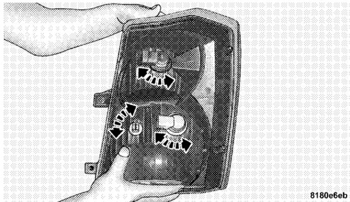
**Removing Socket and Bulb**
