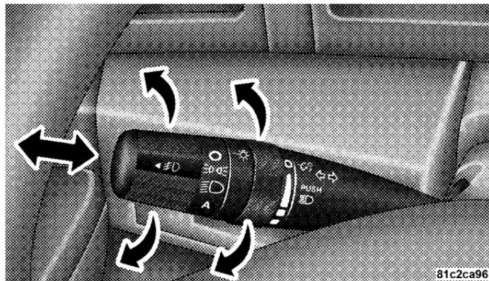
**Headlight Switch****Automatic Headlight System — If Equipped**
