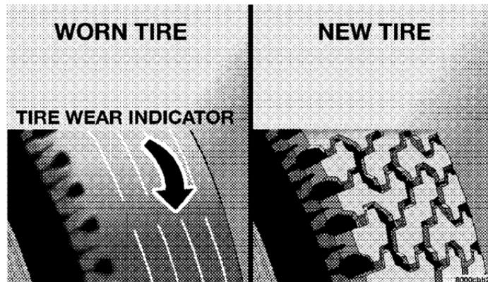
These indicators are molded into the bottom of the tread grooves. They will appear as bands when the tread depth becomes 1/16 inch (2 mm). When the indicators appear in 2 or more adjacent grooves, the tire should be replaced.
