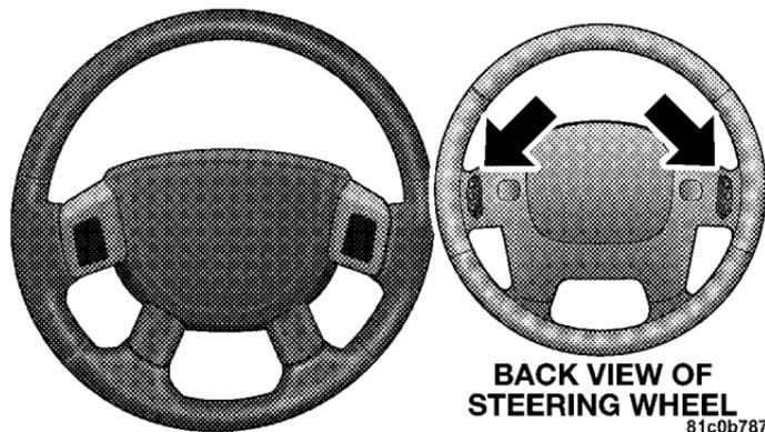
The right hand control is a rocker type switch with a push-button in the center and controls the volume and
