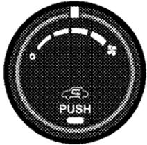
Use this control to regulate the amount of air forced through the ventilation system in any mode. The blower speed increases as you move the control to the right from the “0” (Off) position. There are four blower speeds.
