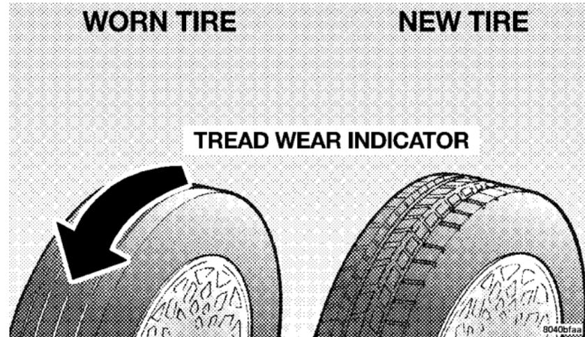
These indicators are molded into the bottom of the tread grooves. They will appear as bands when the tread depth becomes 1/16 in (2 mm). When the tread is worn to the tread wear indicators, the tire should be replaced.
