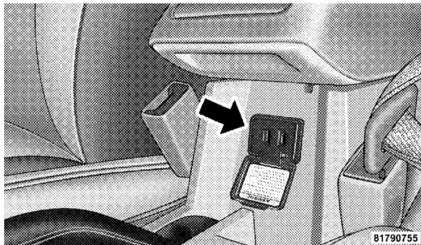
Power Outlet — 115 Volts (150 Watts)
