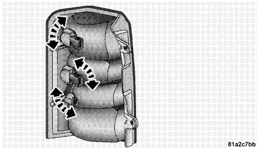
Removing Socket and Bulb
