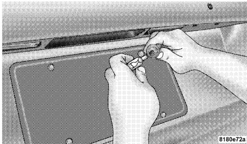
Removing Bulb From Socket
