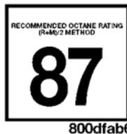
All engines (except 5.7L engines) are designed to meet all emissions regulations and provide excellent fuel economy and performance when using high quality unleaded "regular" gasoline having an octane rating of 87. The use of premium gasoline is not recommended. Under normal conditions, the use of premium gasoline will not provide a benefit over high quality regular gasoline, and in some circumstances may result in poorer performance.
