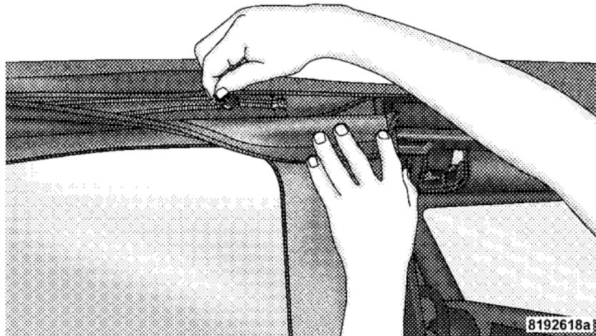
15. Insert the front retainer of the window into the door channel, making sure the retainer is fully seated and properly positioned on the door frame. Failure to do so can result in wind and water leaks or damage to the window.
