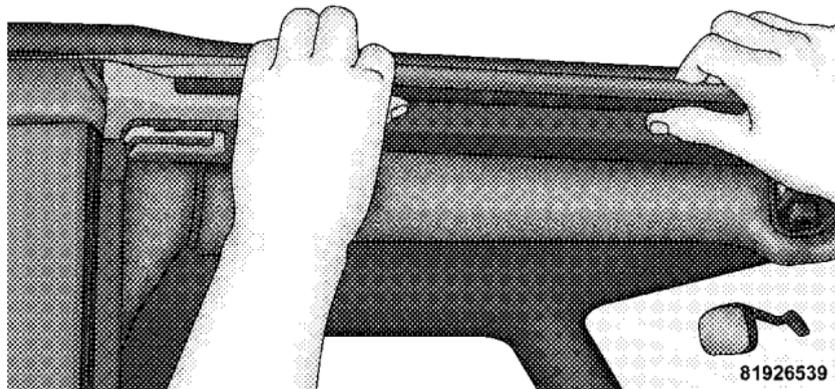
24. Ensure plastic retainer is tucked in properly at B-pillar, not pinching the seal.
