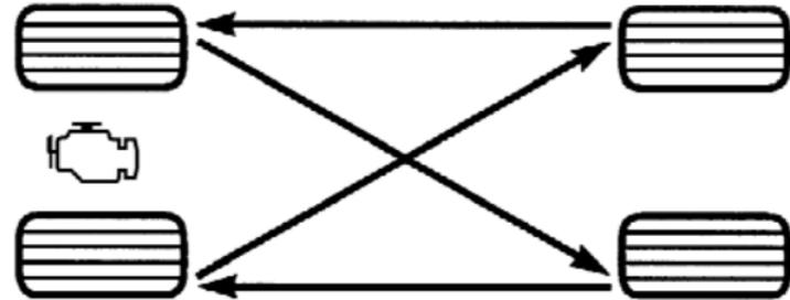
These effects can be reduced by timely rotation of tires. The benefits of rotation are especially worthwhile with aggressive tread designs such as those on On/Off-Road type tires. Rotation will increase tread life, help to maintain mud, snow, and wet traction levels, and contribute to a smooth, quiet ride.
