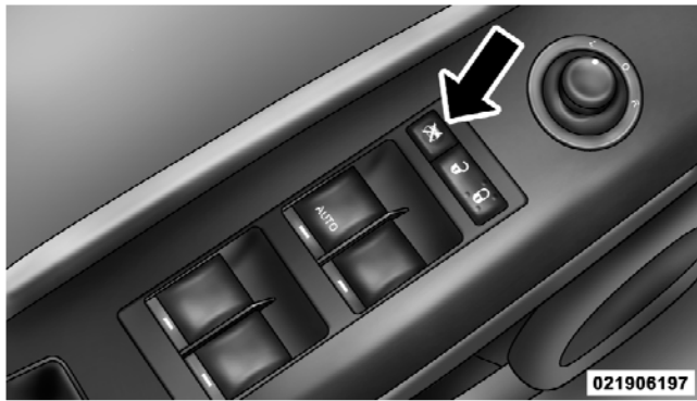
Window Lockout Switch
