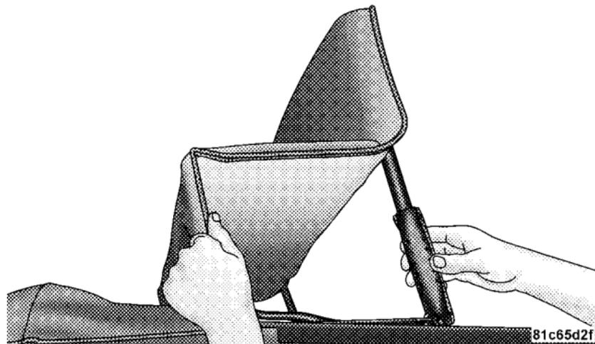
6. Locate the straps to secure the side bows. Wrap the straps around the bows as shown. Repeat on the other side.
