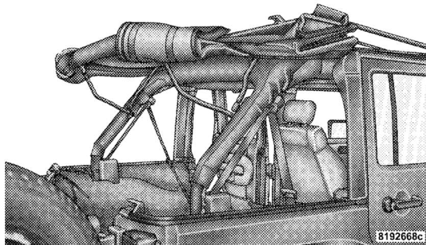
12. The swing gate brackets do not need to be removed unless the hard top is being installed. To remove the swing gate brackets, pull the front of the bracket forward while rolling the entire bracket back in toward the vehicle to disengage.
