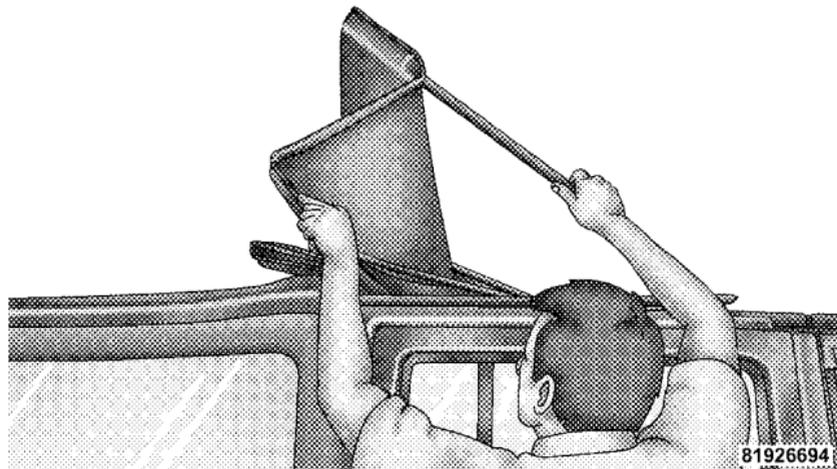
15. Fold the top material so that the plastic retainers form a "W" as shown. Enter the vehicle and move the material into two folds.
