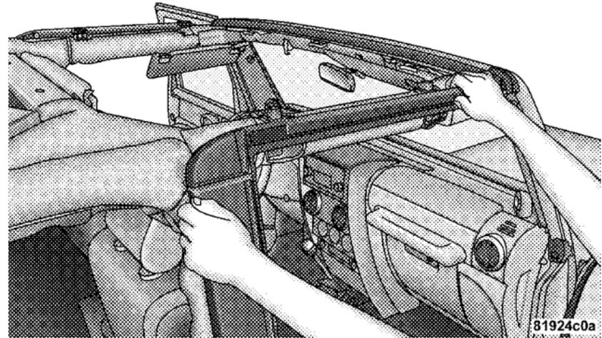
5. Starting with the front knob, screw in and tighten both knobs. Repeat on the other side.
