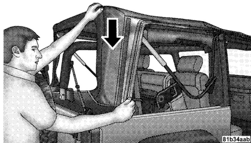
11. To install the side windows, affix the window temporarily by attaching to the Velcro® in the rear corner. Start the zipper but close only about 1 in (2.5 cm).
