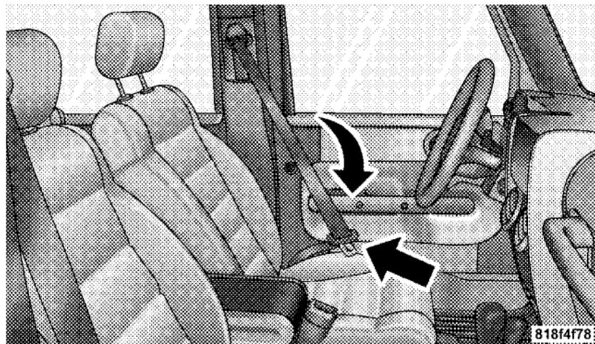
**Pulling Out the Lap/Shoulder Belt Latch Plate**
