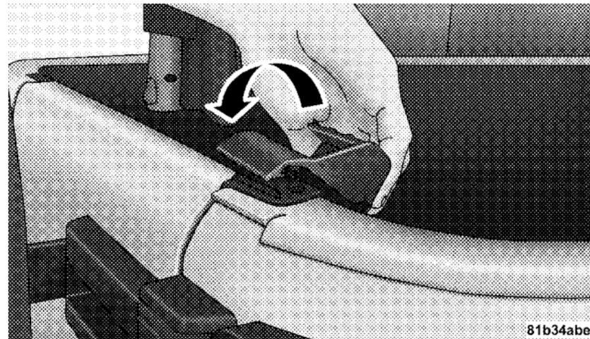
9. Move to the rear of the vehicle and gently pull the sail panels over the rear roof bow.
