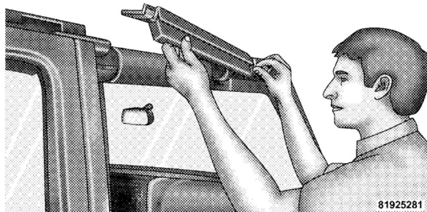
6. Loosely install both knobs beginning with the front knob (long knob). Then, install the middle knob (short knob) through the front and rear door frames and screw into the top of the B-pillar.
