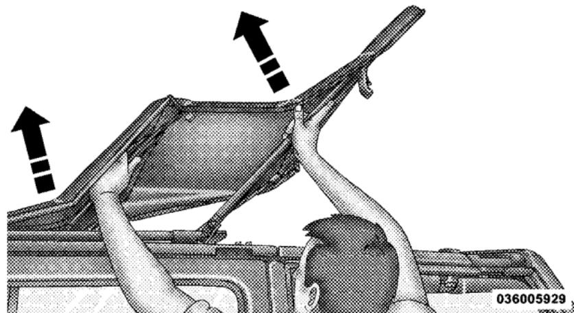
9. Before attaching the header latches, be sure the top retainers above the doors do not get trapped between the top and the door frame. Also, make certain the feet at
