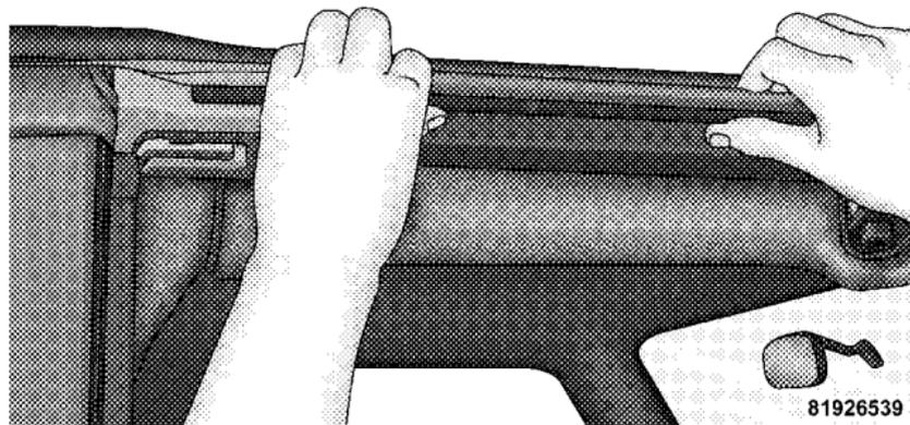
22. Ensure the plastic retainer is tucked in properly at the B-pillar and not pinching the seal.
