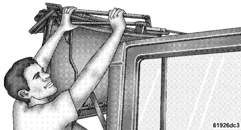
18. Gently slide the side bows off the door frame track and lower the top down into the vehicle.
