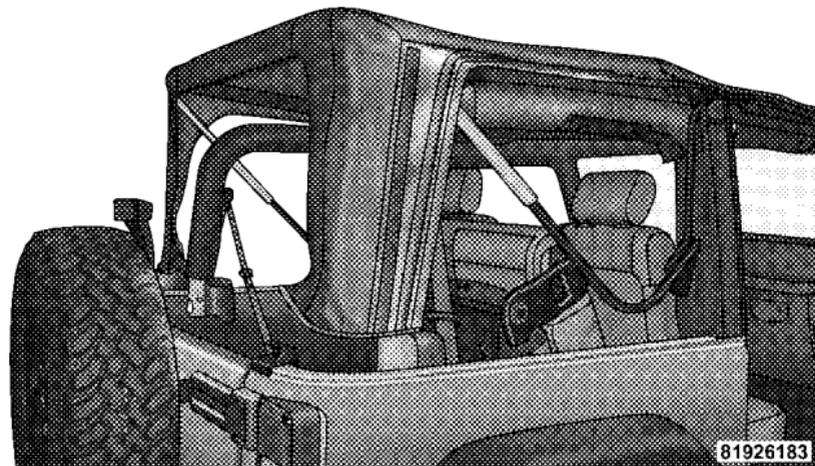
10. Partially install the sail panel retainers into the body side channel, leaving the last 3 in (7.6 cm) toward the rear window loose (on both sides). Pulling down on the rear roof bow (3-bow) will aid to reach the channel with the retainers.
