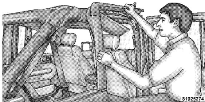
3. Position the top of the door frame against the metal sport bar and press onto the side bar making sure not to pinch the material of the sports bar covers and to ensure it is properly positioned on the seal above the front of the rear door.
