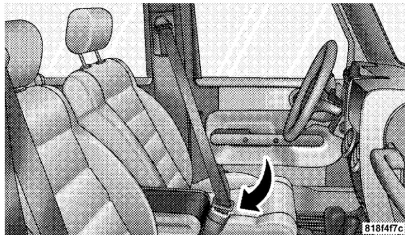
**Inserting Latch Plate into Buckle**
