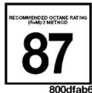
All engines are designed to meet all emissions regulations and provide excellent fuel economy and performance when using high quality unleaded “regular” gasoline having an octane rating of 87. The use of premium gasoline is not recommended, as it will not provide any benefit over regular gasoline in these engines.
