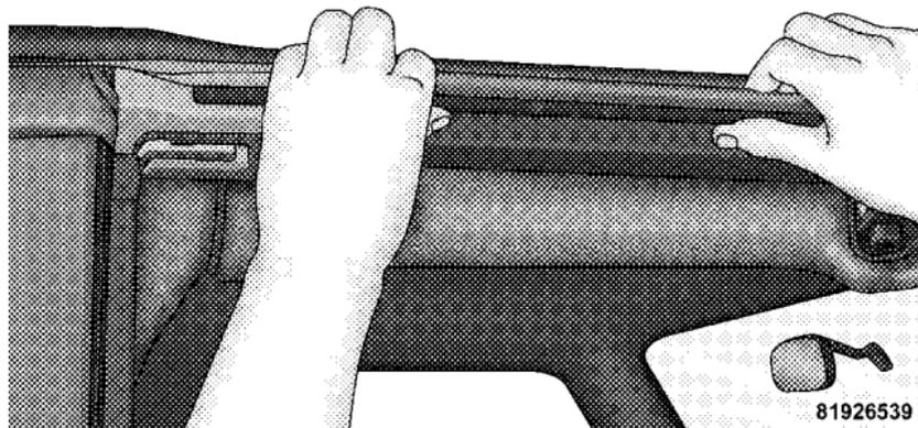
20. Close the header latches and return the sun visors to their secured position.
