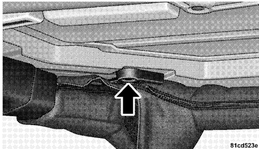
4. Turn the rear fasteners (knobs) (located on the overhead speaker bar assembly) counter-clockwise until they can be removed.
