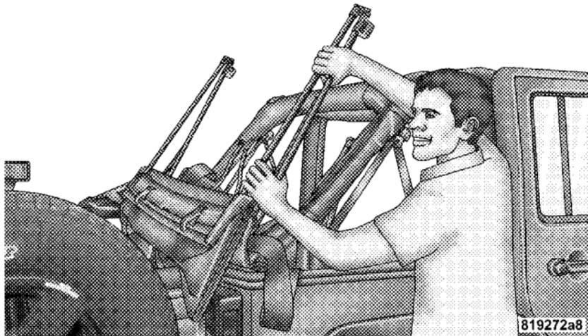
19. Tuck the fabric and the check straps between the bows as far inside as possible. This will keep any portion of the top from flapping outside of the vehicle.
