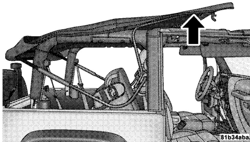
17. Tuck the fabric and the check straps between the bows and as far inward as possible. This will keep any portion of the top from flapping outside of the vehicle.
