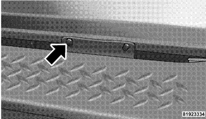
2. Remove one bolt from the underside of the vehicle.
