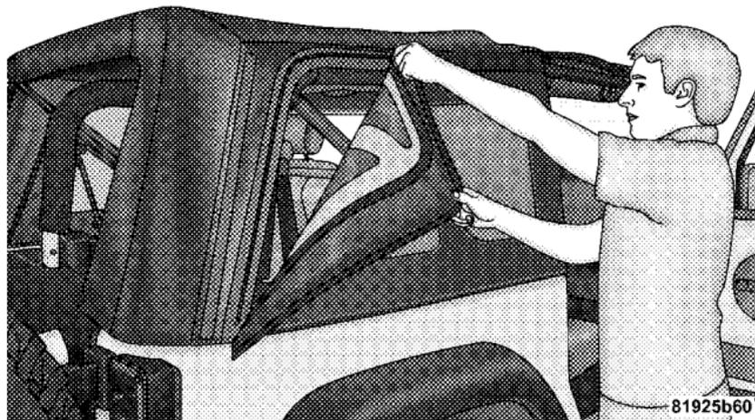
9. Once unzipped, remove the side window retainers from the door channel and body side channel. Repeat this step on the opposite side.
