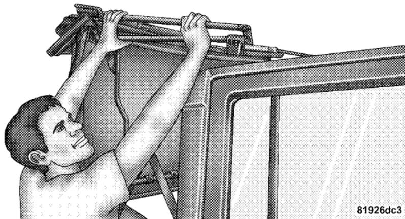
6. Ensure that the top locks into the Sunrider® locking mechanisms that are located above the front of the rear doors.
