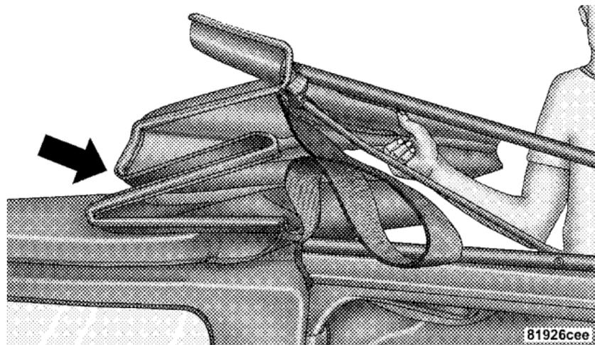
16. Release the side bows by pressing down on the latch above the front of the rear door. Push the top rearward to disengage. Repeat this step on the other side.
