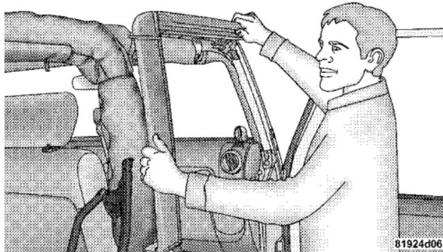
3. After the door frame pin has been set into the body side hole, carefully set the front of the door frame into the rubber seal at the top of the windshield.
