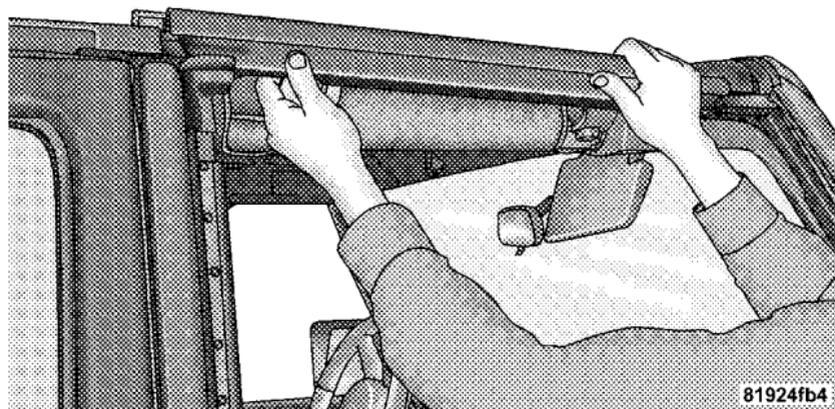
3. Pull the frame toward you with your front hand to remove the frame from the vehicle.
