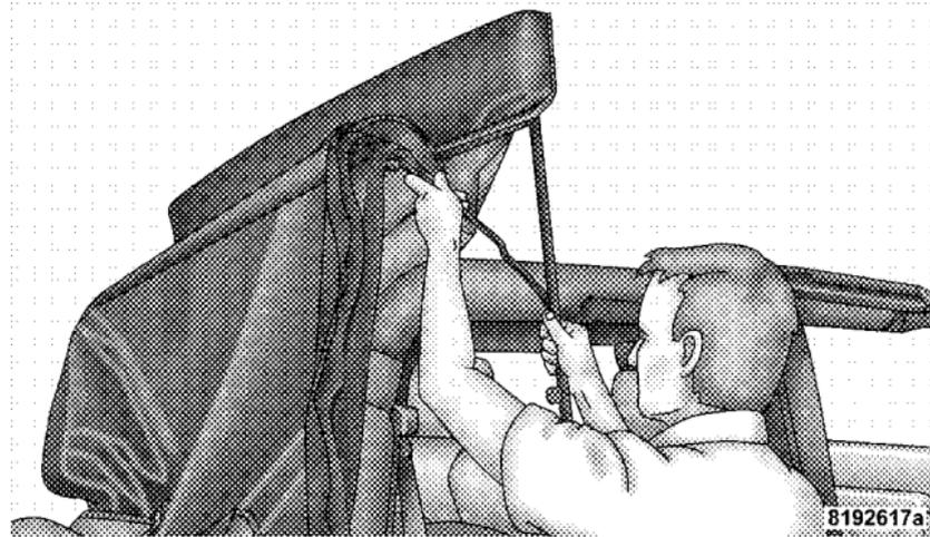
5. Before attaching the header latches, be sure that the top retainers above the door are not trapped between the top and the door frame.
