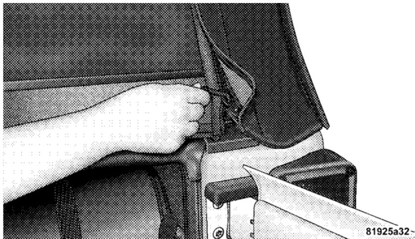
7. Undo the Velcro® that runs along the top and rear edge of the side window.
