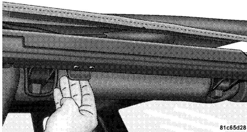
16. Before lowering the top, open the swing gate to prevent possible damage to the rear center high-mounted brake light. Move to the front of the vehicle. Grasp the side bow behind the header and lift the top, folding it toward the rear of the vehicle.
