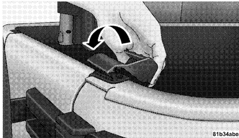
12. Ensure that the straps are positioned correctly before pulling the sail panels over the rear roof bow (4-bow).
