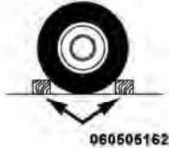
6. Block both the front and rear of the wheel diagonally opposite of the jacking position. For example, if changing the right front tire, block the left rear wheel.
