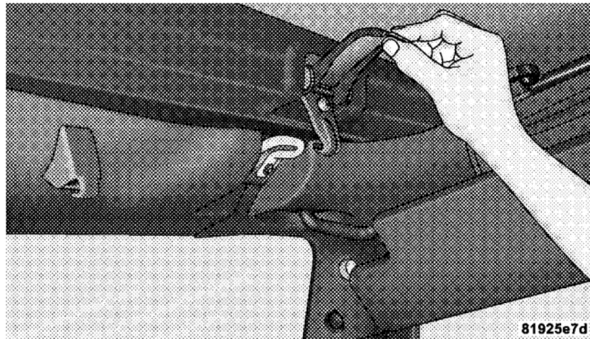
4. Grasp the front side bow behind the header, and lift the top.
