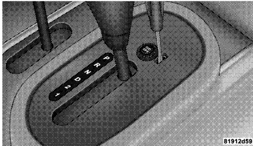
**Brake/Transmission Interlock Manual Override**
