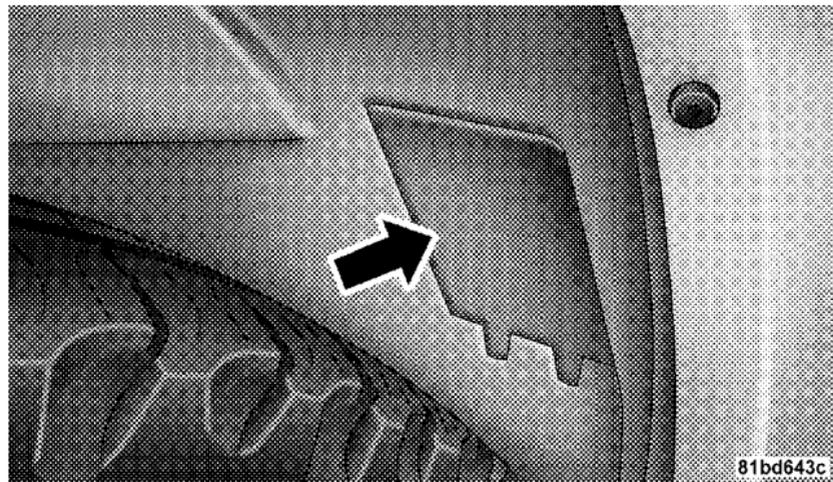
3. Reach through the access hole to access the back of the front fog lamp housing on the back of the front fascia.
