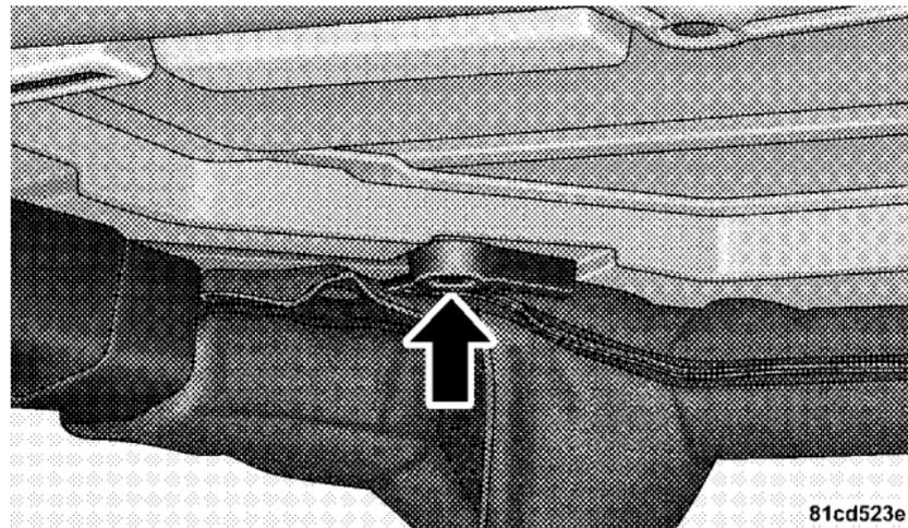
5. Unlatch the header panel latch located at the top of the windshield.
