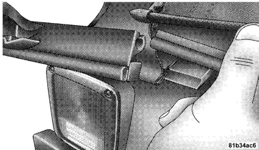
16. Install the rear window by starting both zipper ends at the lower left corner of the rear window opening. Ensure that the zippers are properly started and aligned before zipping to prevent damage.
