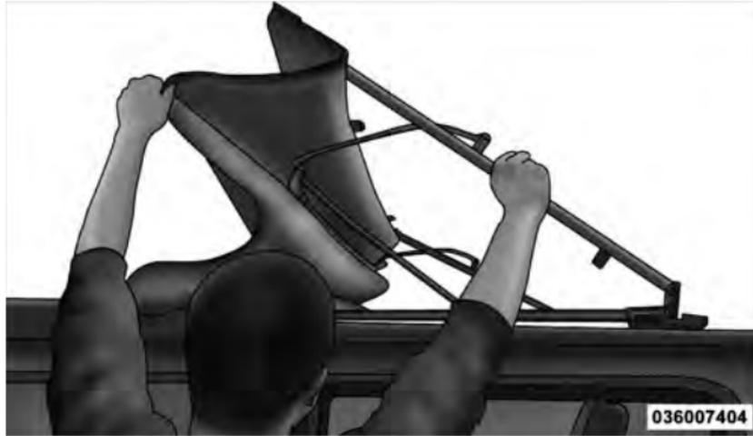
16. Fold the top so that the material forms a "W" as shown. Enter the vehicle and move the material into two folds.
