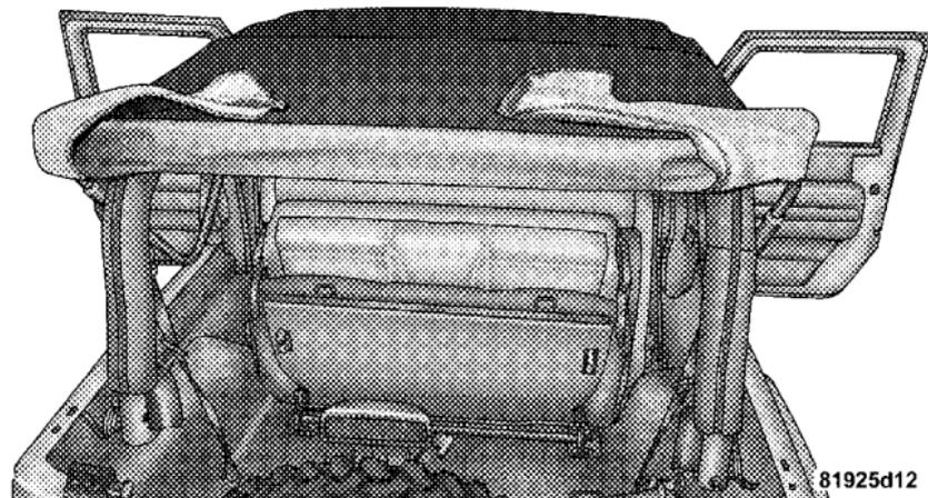
13. The swing gate brackets do not need to be removed unless the hard top is being installed. To remove the swing gate brackets, pull the front of the bracket forward while rolling the entire bracket back in toward the vehicle to disengage.
