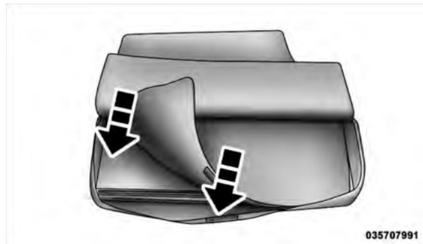
Insert the left-side Freedom panel into the bag with the latches facing upward.
