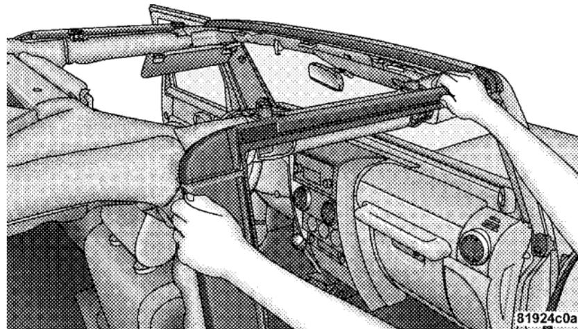
5. Starting with the front knob, screw in and tighten both knobs. Repeat on the other side.
