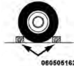
6. Block both the front and rear of the wheel diagonally opposite of the jacking position. For example, if changing the right front tire, block the left rear wheel.
