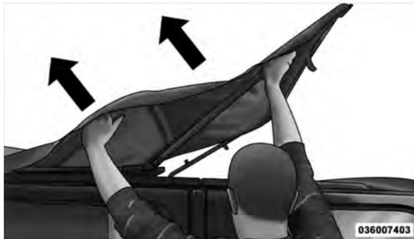
15. Fold back the front section of the top, pulling the fabric rearward. Gently rest the header on top of the rear portion of the deck.
