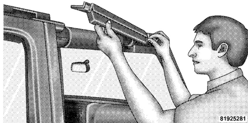
6. Clip the front of the door rail over the side bar making sure that the material for the side bar cover is not pinched by the door frame.
