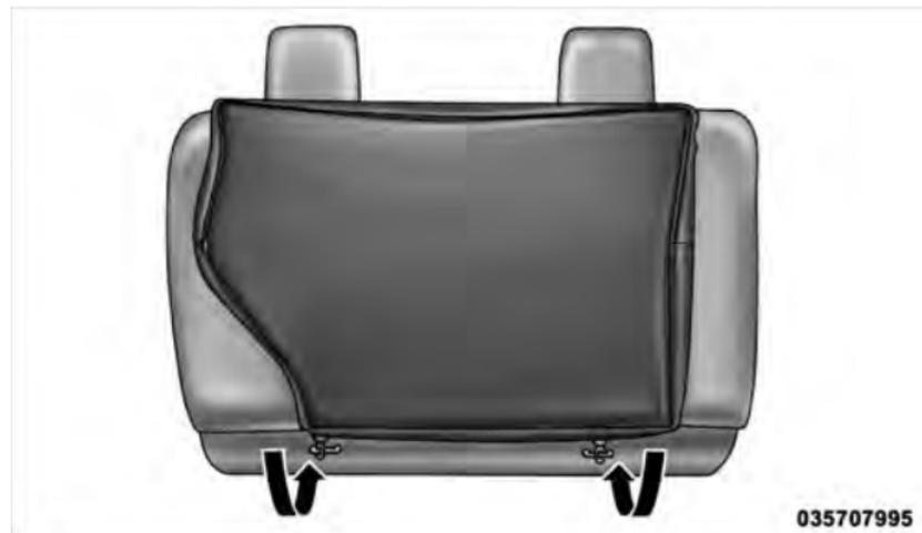
Wrap the upper strap around the rear head restraints and loop the strap through the buckle. Pull on the strap to tighten the Freedom bag securely against the rear seat.
