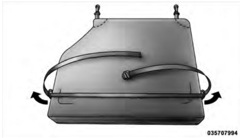
Lift the Freedom bag into the vehicle with the hooks and straps facing the back of the rear seat. Attach the clips at the bottom of the bag to the child restraint anchorages, located at the base of the rear seat.
