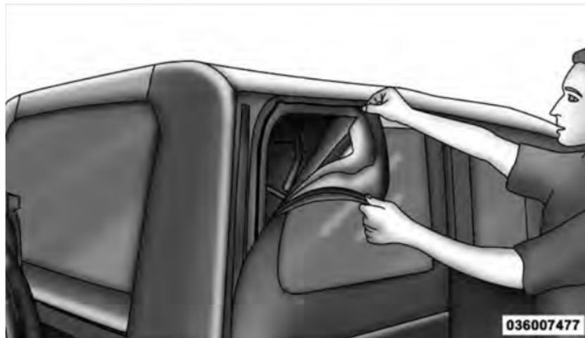
10. Once unzipped, remove the side window retainers from the door channel and body side channel. Repeat this step on the opposite side.
