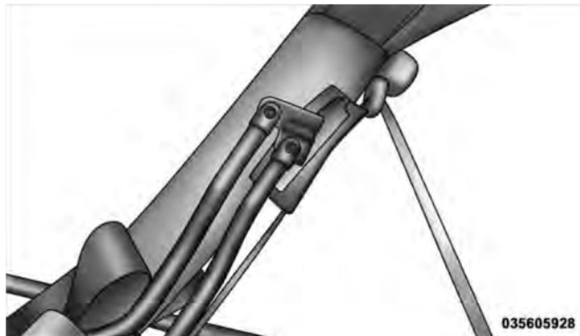
b. Lay the soft top into the rear of the vehicle with the bows pointing forward and the curved portion of the bows facing upward.
