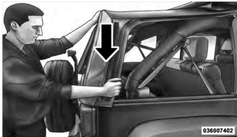
3. Rotate the header forward.
