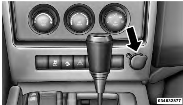
Front Power Outlet
