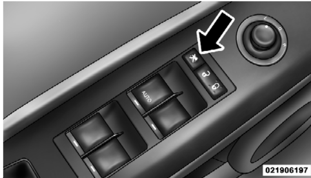
Window Lockout Switch
