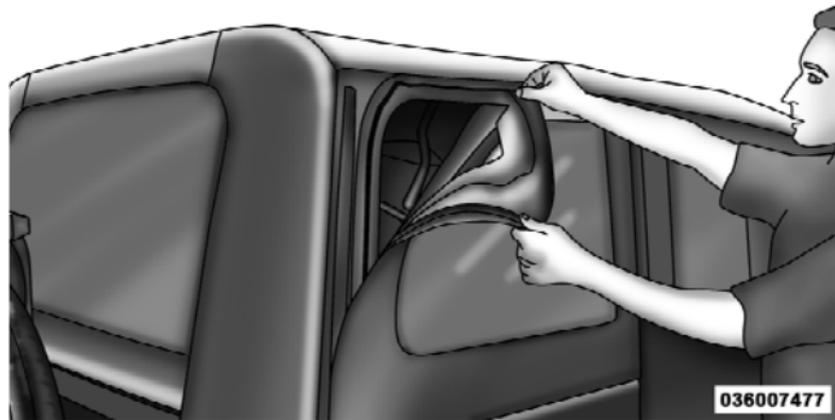
2. Release header latches from the windshield frame.
