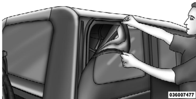
10. Once unzipped, remove the side window retainers from the door channel and body side channel. Repeat this step on the opposite side.
