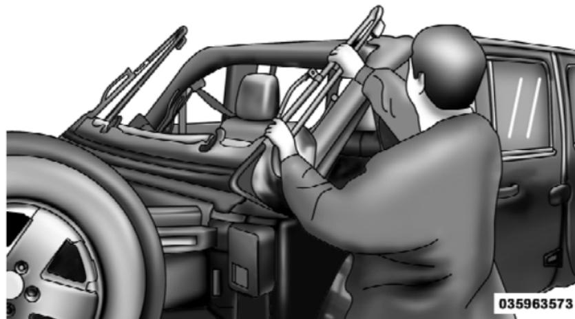
**NOTE:** Ensure the fabric does not overhang the sides of the vehicle.
