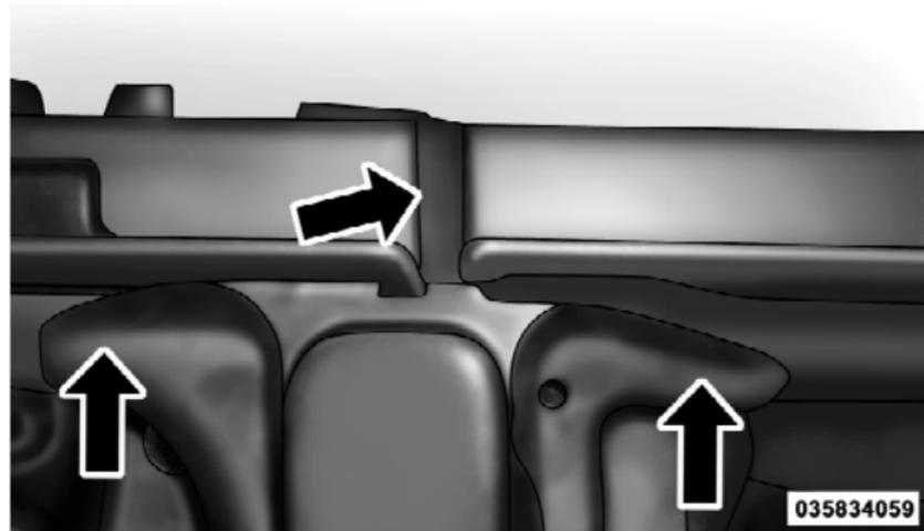
8. Loosely install both knobs beginning with the front knob (long knob). Then, install the middle knob (short knob) through the front and rear door frames and screw into the top of the B-pillar.
