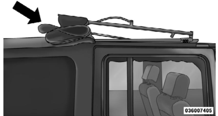
17. Release the side bows by pressing down on the latch above the front of the rear door. Push the top rearward to disengage. Repeat this step on the other side.
