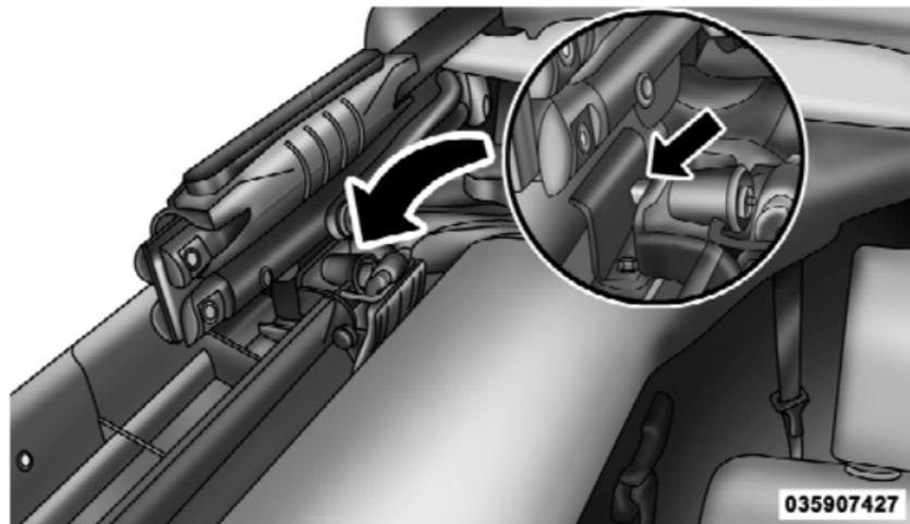
6. Open the header latches and engage the hook on each side onto the windshield loops (do not close the latches).
