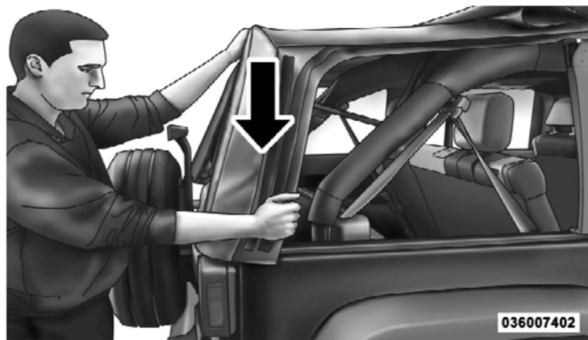
3. Rotate the header forward.
