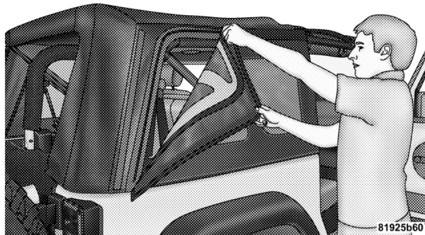
10. Once unzipped, remove the side window retainers from the door channel and body side channel. Repeat this step on the opposite side.
