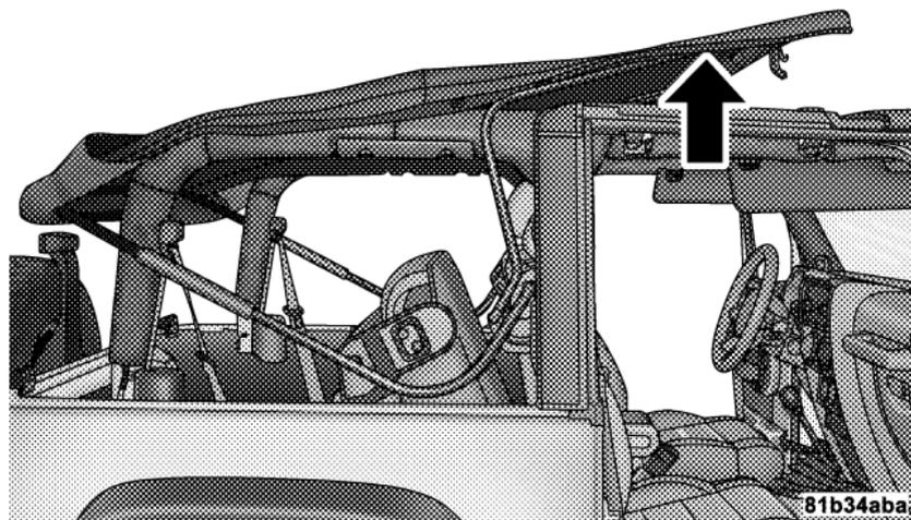
18. Tuck the fabric and the check straps between the bows and as far inward as possible. This will keep any portion of the top from flapping outside of the vehicle.
