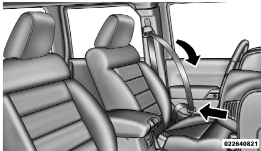
**Pulling Out The Lap/Shoulder Belt Latch Plate**
