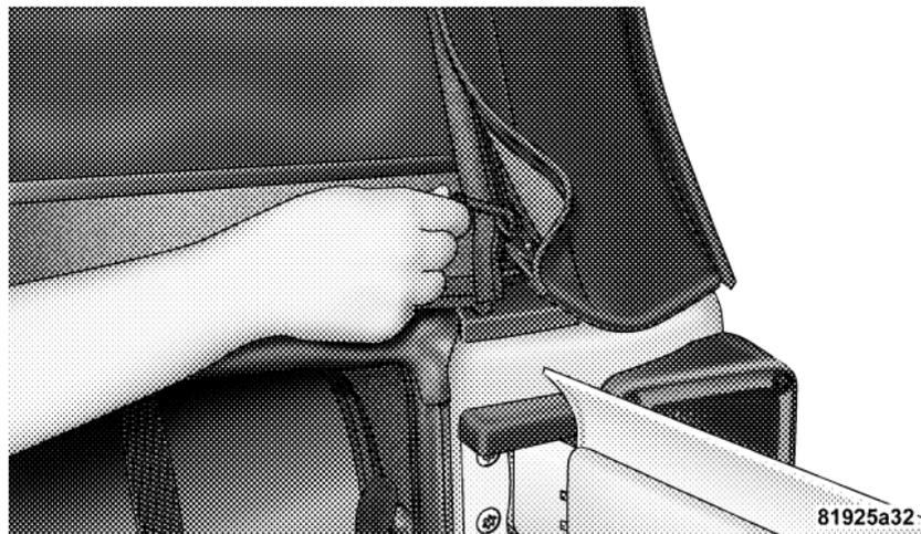
6. Remove the rear window retainer from the swing gate bracket on both the left and right sides.
