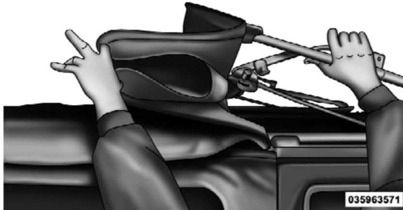
16. Fold the top so that the material forms a "W" as shown. Enter the vehicle and move the material into two folds.
