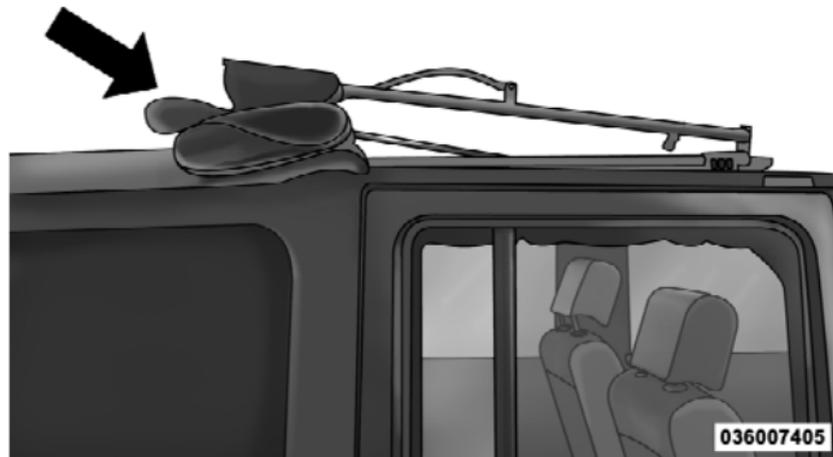
6. Secure the top by using the two provided straps. Each strap will wrap around the side bow and Velcro® to itself; use one strap on each side of the vehicle.
