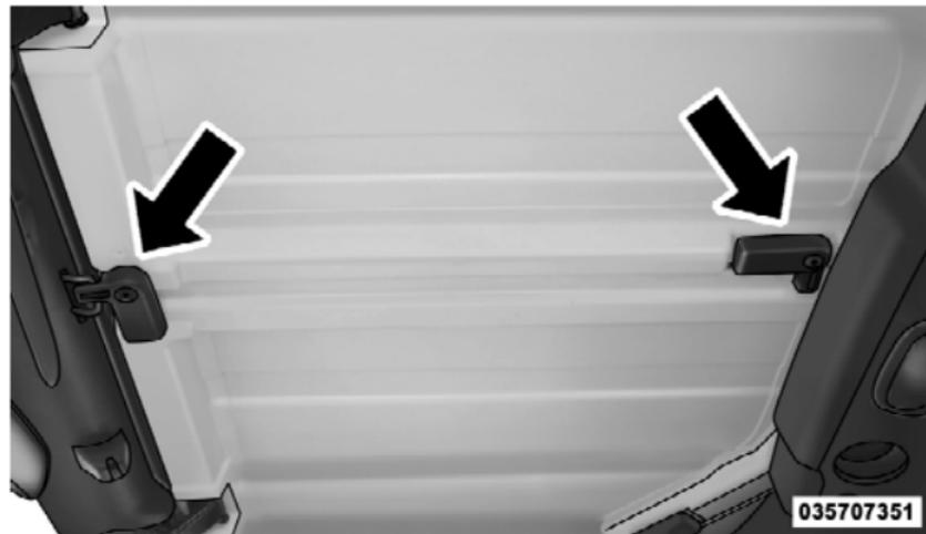
4. Turn the rear L-shaped lock (located above the shoulder belt anchorage).
