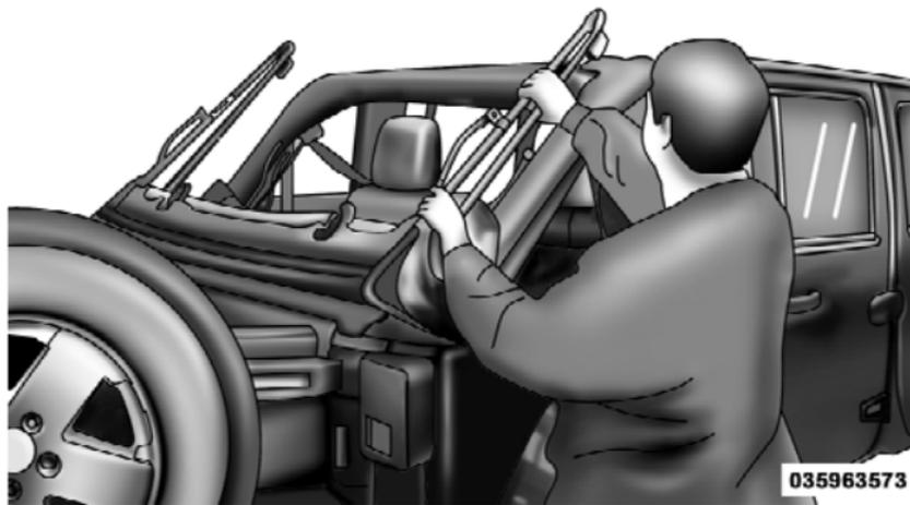
5. Insert the slider feature of the knuckles into the door frame tracks and slide the top forward.
