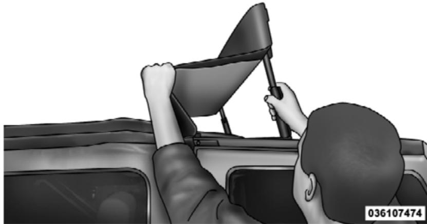
5. Locate the straps to secure the side bows. Wrap the straps around the bows as shown. Repeat on the other side.
