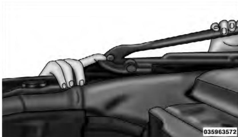
18. Before lowering the top, open the swing gate to prevent possible damage to the rear center high-mounted brake light. Grasp the folded side bows and slide the top along the door frame track to the rear door frame.
