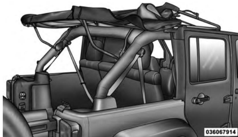
13. The swing gate brackets do not need to be removed unless the hard top is being installed. To remove the swing gate brackets, pull the front of the bracket forward while rolling the entire bracket back in toward the vehicle to disengage.
