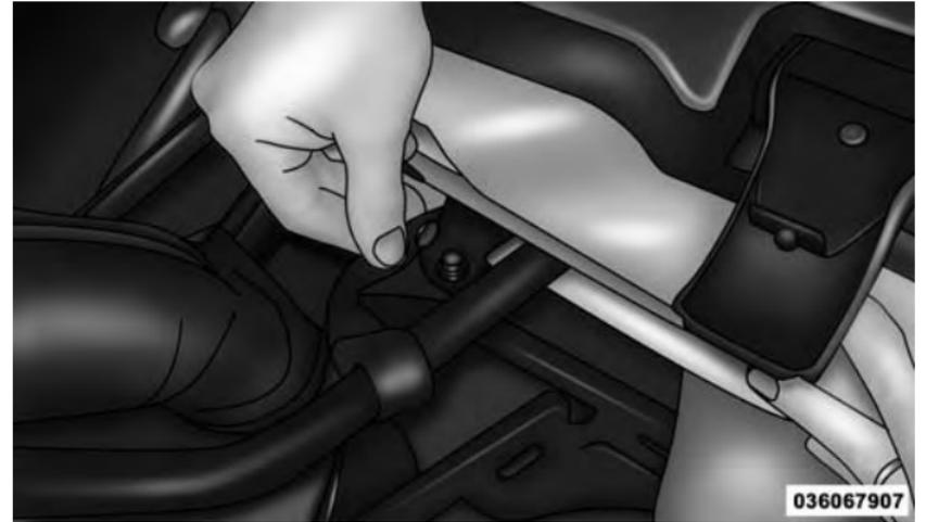
8. Remove the swing gate bar (black metal bar for bottom of rear window) and set aside.
