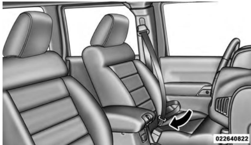
Inserting Latch Plate Into Buckle
