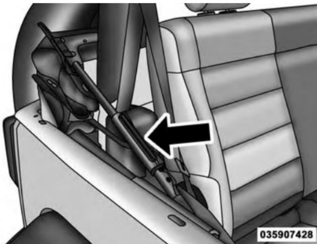
4. Standing on the side of the vehicle, lift the top by the side bow and the 2-bow (middle bow) up and over the sports bar until the header rests on the top of the windshield frame.
