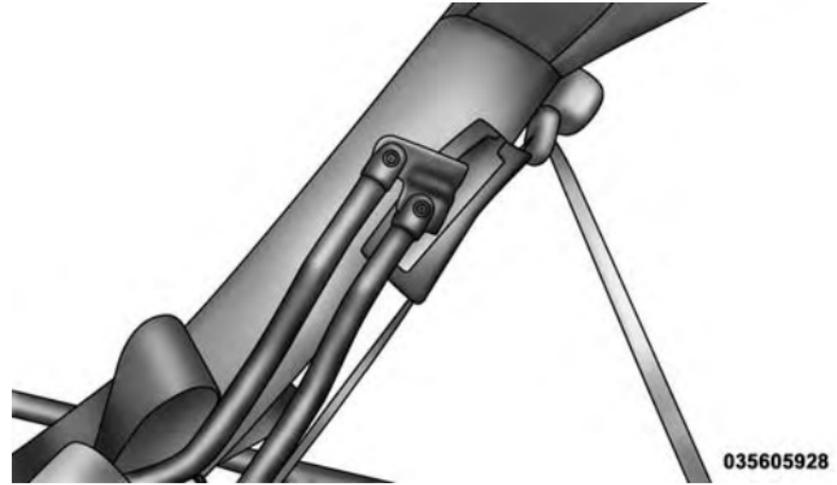
2. Lay the soft top into the rear of the vehicle with the bows pointing forward and the curved portion of the bows facing upward.
