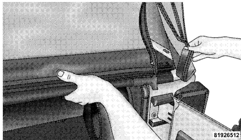
17. Insert the rear window retainer into the swing gate bracket on both the left and right sides.
