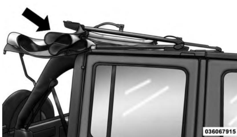
17. Release the side bows by pressing down on the latch above the front of the rear door. Push the top rearward to disengage. Repeat this step on the other side.
