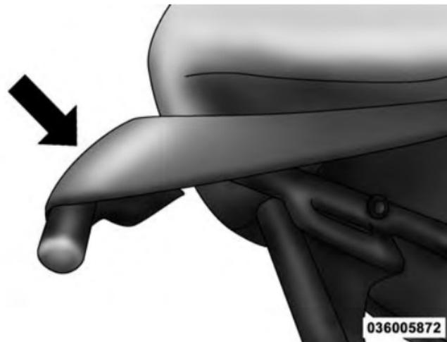
Partially install the sail panel retainers into the body side channel, leaving the last 3 in (7.6 cm) toward the rear window loose (on both sides). Pulling down on the rear roof bow (4-bow) will aid in reaching the channel with the retainers.
