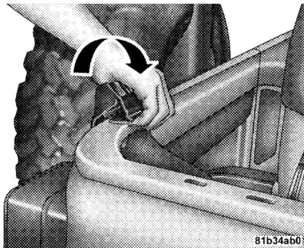
14. Grasp the front side bow behind the header, and lift the top.
