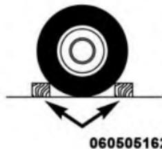
Block both the front and rear of the wheel diagonally opposite of the jacking position. For example, if changing the right front tire, block the left rear wheel.
