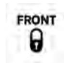
Indicates when the front axle lock has been activated.
