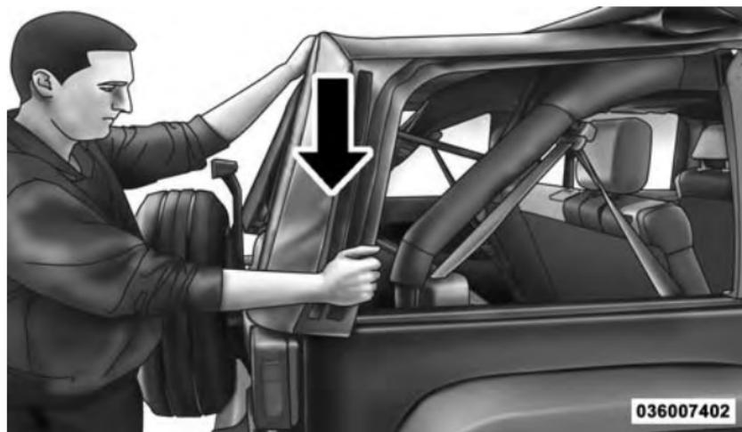
3. Rotate the header forward.
