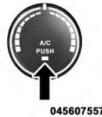
Press this button to engage the Air Conditioning. A light will illuminate when the Air Conditioning system is engaged. Rotating the dial left into the blue area of the scale indicates cooler temperatures, while rotating right into the red area indicates warmer temperatures.
