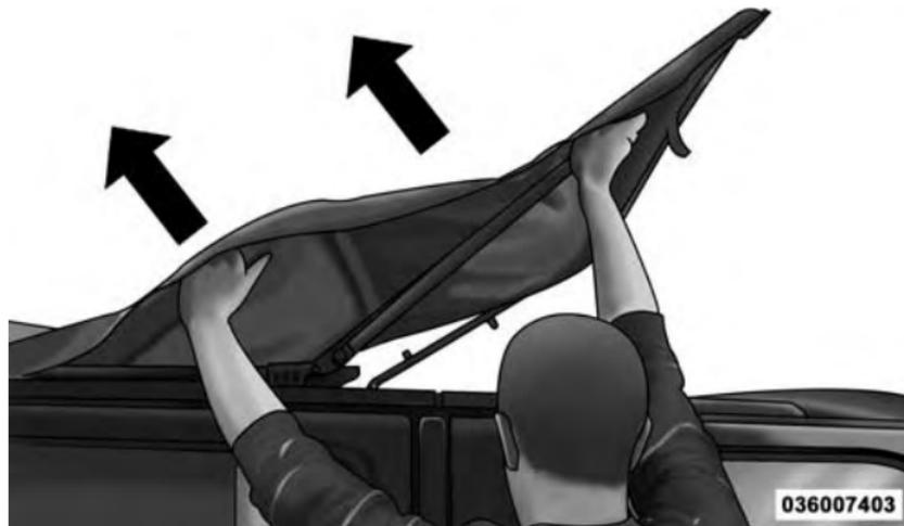
4. Fold back the front section of the top and gently rest the header on top of the rear portion of the deck.
