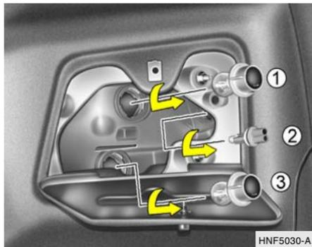
3. To replace the rear combination light (stop/tail light, rear side marker light and rear turn signal light), remove it from the bulb holder and install the new bulb.
