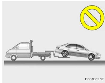
A vehicle with an automatic transaxle should never be towed from the rear with the front wheels on the ground. This can cause serious damage to the transaxle.
