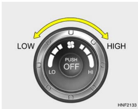
The fan speed can be set to the desired speed by turning the fan speed control knob. The higher the fan speed is, the more air is delivered. Pressing the "OFF" button turns off the fan.
