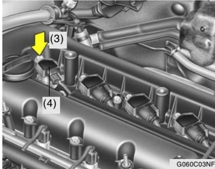
6. Remove the mounting bolt (3) of the ignition coil with a socket wrench.
