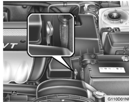
2. Remove the transaxle dipstick, wipe it clean, reinsert the dipstick as far as it will go, then remove it again. Now check the fluid level on the dipstick. It should be in the "HOT" range on the dipstick.
