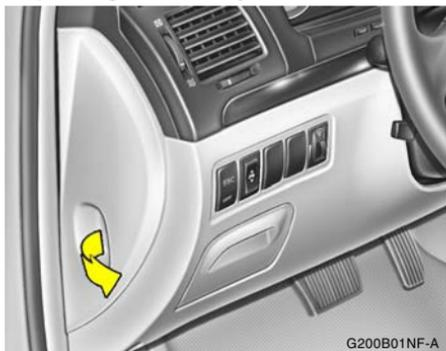
The fuse box for the lights and other electrical accessories will be found on the left side of the instrument panel. Inside the box you will find a list showing the circuits protected by each fuse. If any of your car's lights or other electrical accessories stop working, a blown fuse could be the reason. If the fuse has burned out, you will see that the metal strip inside the fuse has burned through. If you suspect a blown fuse, follow this procedure:
