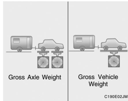
2. The total gross vehicle weight with trailer must not exceed the Gross Vehicle Weight Rating (GVWR) shown on the vehicle identification plate (see page 8-2). The total gross vehicle weight is the combined weight of the vehicle, driver, all passengers and their luggage, cargo, hitch, trailer tongue load and other optional equipment.
