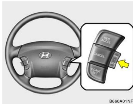
1. Push the cruise control ON/OFF switch. The "CRUISE" indicator light in the instrument cluster will illuminate. This turns the system on.
