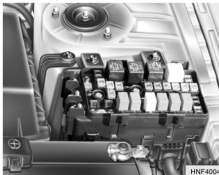
A fusible link will melt if the electrical circuits from the battery are ever overloaded, thus preventing damage to the entire wiring harness. (This could be caused by a short in the system drawing too much current.) If this ever happens, have a Hyundai dealer determine the cause, repair the system and replace the fusible link. The fusible links are located in a relay box in the engine compartment for easy inspection.
