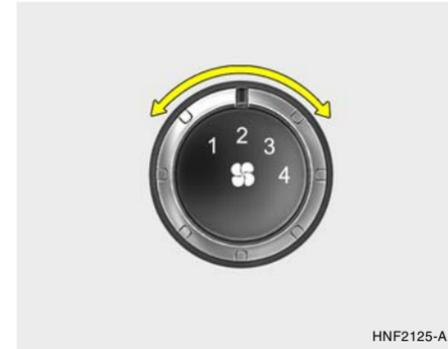
This is used to select the blower fan speed. The blower fan speed, and therefore the volume of air delivered from the system, may be controlled manually by setting the blower control between the "1" and "4" position. 1 is the lowest fan speed and 4 is the highest fan speed.
