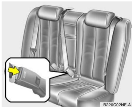
When you want to release the seat belt, press the button in the locking buckle.
