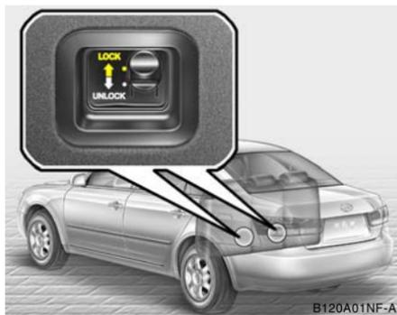
If the rear seatback lock knob (located on the backside of the rear seatback) is in the "LOCK" position when the rear seatbacks are upright and closed, it will not be possible to fold the rear seatback by using the seatback release lever. In this instance, move the lock knob to the "UNLOCK" position and fold the rear seatback. The rear seatback lock knob is designed to provide protection from unauthorized entry into the trunk.
