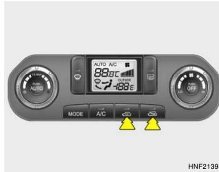
This is used to select fresh outside air or recirculation of inside air.
