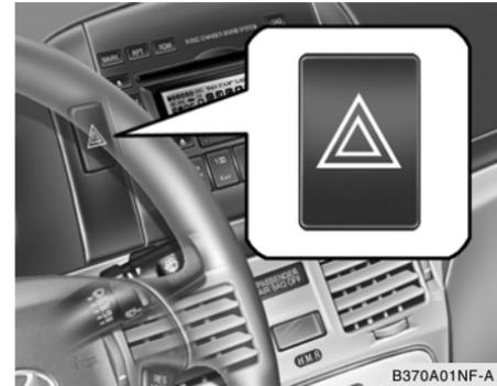
The hazard warning system should be used whenever you find it necessary to stop the car in a hazardous location. When you must make such an emergency stop, always pull off the road as far as possible.
