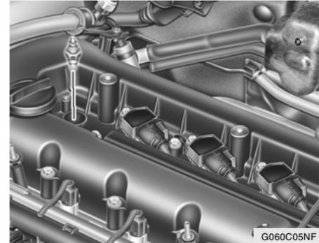
10. To install the new spark plug, guide the socket down over the spark plug, being careful not to damage the ceramic insulator.
