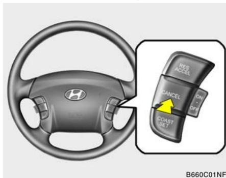
To disengage the cruise control system, push the control switch "CANCEL". Additionally, the following actions will disengage the system:
