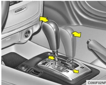
While the engine is idling, apply the brakes and move the gear selector lever from "P" to each of its other positions — "R", "N", "D" — and then return to "N" or "P". With the engine still idling:
