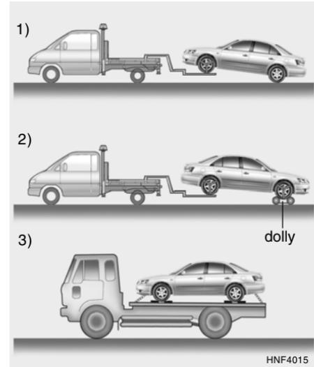
Your vehicle can be towed by wheel lift type truck (1), (2) or flatbed equipment (3).
