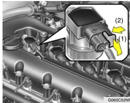
4. Pull the ignition connector key in the direction of (1).
