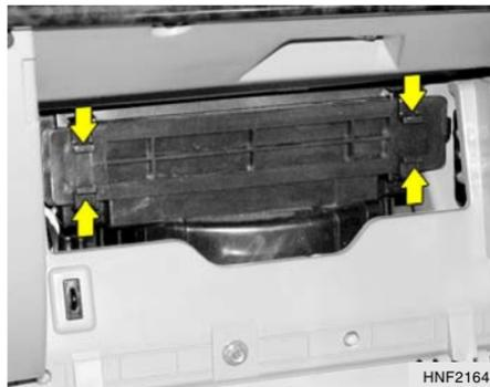
4. Remove the air conditioner filter cover by pressing both side clips.
