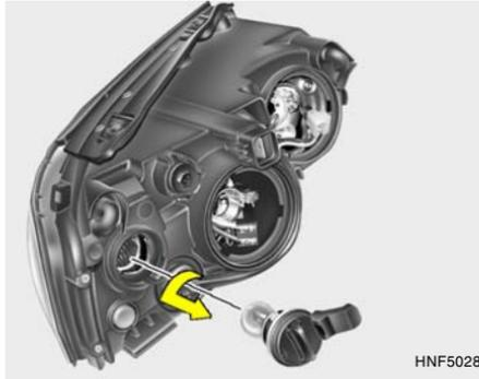
12. To replace the front turn signal light bulb (front position light), remove it from the bulb holder and install the new bulb.
