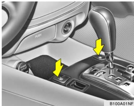
The seat warmer is provided to warm the front seats during cold weather. With the ignition key in the "ON" position, push either of the switches to warm the driver's seat or the front passenger's seat.
