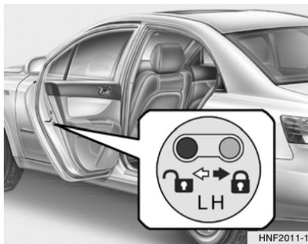
Your Hyundai is equipped with left and right side "child-protector" rear door locks. When the lock mechanism is engaged, the rear door cannot be opened from the inside. Its use is recommended whenever there are small children in the rear seat.
