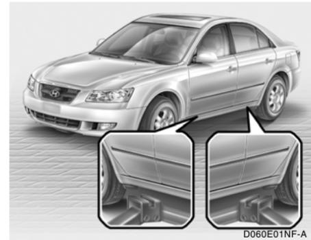
The base of the jack should be placed on firm, level ground. The jack should be positioned as shown in the drawing.
