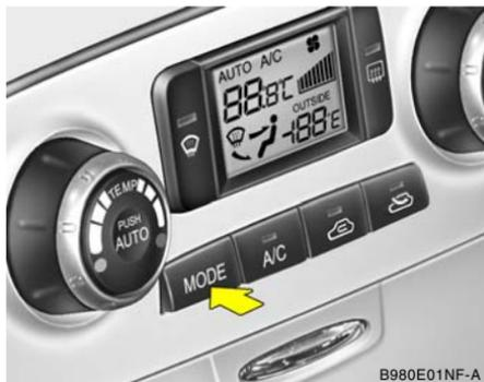
This is used to direct the flow of air. Air can be directed to the floor, dashboard outlets, or windshield. Four symbols are used to represent Face, Bi-Level, Floor, Floor-Defrost position.
