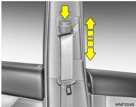
You can adjust the height of the shoulder belt anchor to one of 3 positions for maximum comfort and safety.
