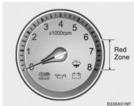
The tachometer registers the speed of your engine in revolutions per minute (rpm).
