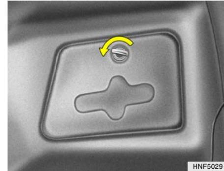
2. Remove the cover on the inside of the rear luggage trim by turning the knob counter-clockwise.
