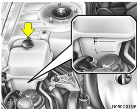
The coolant level can be seen on the side of the plastic coolant reservoir. The level of the coolant should be between the "L" and "F" lines on the reservoir when the engine is warm with it at idle. If the level is below the "L" mark, add engine coolant to bring it up to "F". If the level is low, inspect for coolant leaks and recheck the fluid level frequently. If the level drops again, visit your Hyundai dealer for an inspection and diagnosis of the reason.
