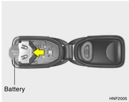
2. Remove the old battery from the case and note the polarity. Make sure the polarity of the new battery is the same(+side facing up), then insert it in the transmitter.
