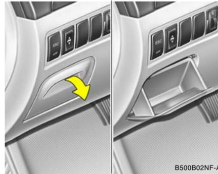
The multi box may be opened by pulling it out by its grip. It is used for storing small articles.
