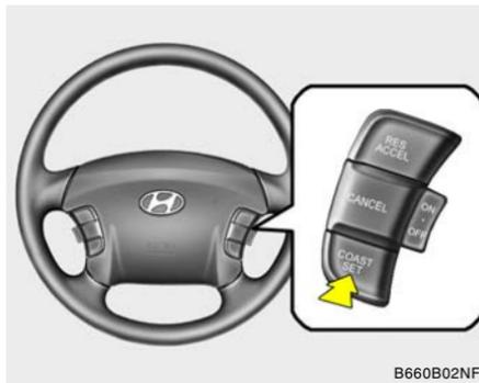
3. Push the "SET" (COAST) switch after you have set the vehicle speed at the desired speed.
