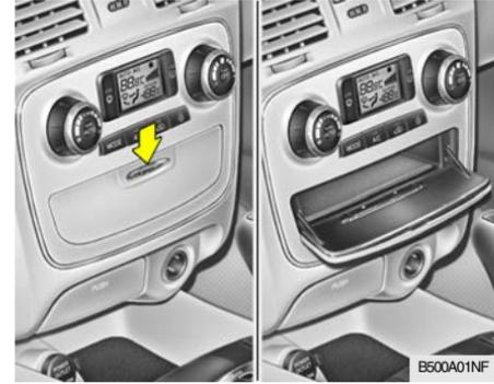
The accessory box may be opened by pushing the knob downward. It is used for storing small articles.
