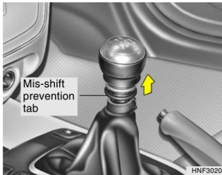
When shifting into reverse gear, pull the mis-shift prevention tab and shift into reverse gear position.
