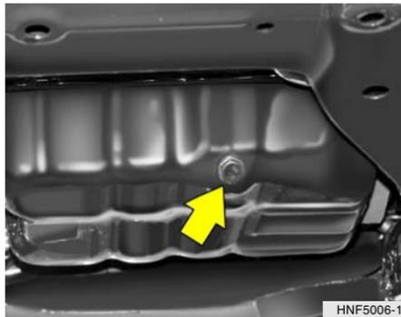
3. Slide underneath the car and loosen the drain plug by turning it counterclockwise with a wrench of the proper size. Be sure that a drain pan is in position to catch the oil as it drains out, then remove the drain plug.
