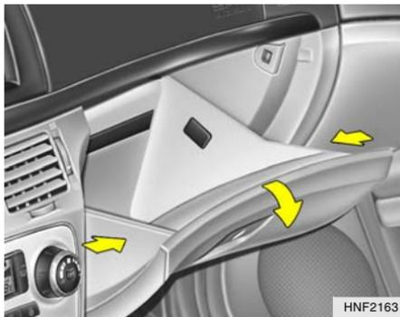
3. Lower the glove box down completely by pushing both sides of the glove box inward.
