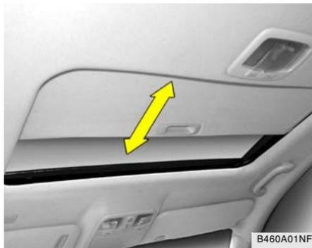
Your HYUNDAI is equipped with a sliding sunshade which you can manually adjust to let in light with the sunroof closed, or to block sunlight.
