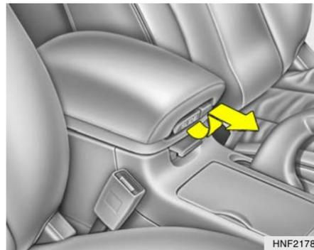
The center console box can be used as armrest. To use the console armrest, pull out the console box lid by pulling up the handle as shown.
