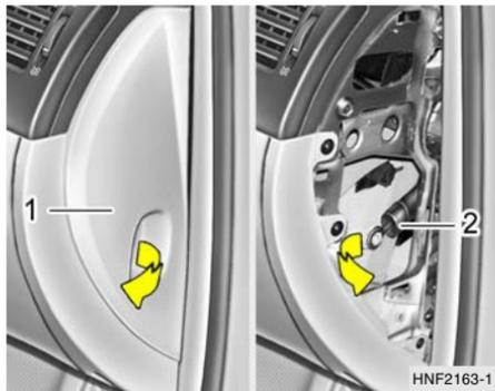
1. Remove the cover (1) which is located to the right side of the instrument panel by pulling it.
