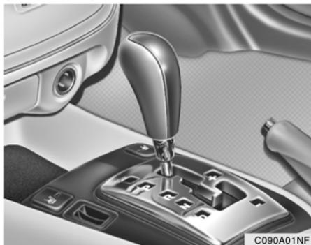
The highly efficient Hyundai automatic transaxle has four/five forward speeds and one reverse speed. The individual speeds are selected automatically, depending on the position of the speed selector lever. The selector lever has 2 gates; the main gate and the manual gate.
