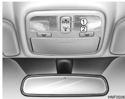
If your vehicle is equipped with this feature, you can slide or tilt your sunroof with the sunroof control buttons located on the overhead console.
