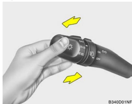
To turn on the headlight high beams, push the lever forward (away from you). The High Beam Indicator Light will come on at the same time. For low beams, pull the lever back toward you.
