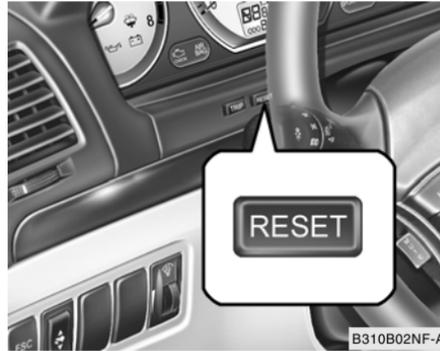
Push in the RESET switch more than 1 second to initialize the displayed information such as tripmeter, average speed, average fuel consumption and drive time.
