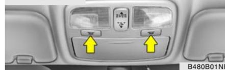
Push in the map light switch to turn the light on or off. This light produces a spot beam for convenient use as a map light at night or as a personal light for the driver and the passenger.
