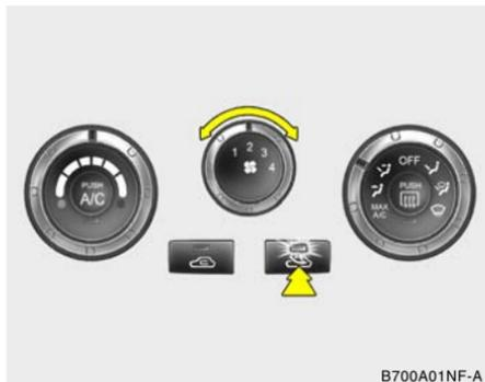
Your Hyundai is equipped with bi-level heating controls. This makes it possible to have cooler air from the dashboard vents and warmer air from the floor outlets at the same time. To use this feature:
