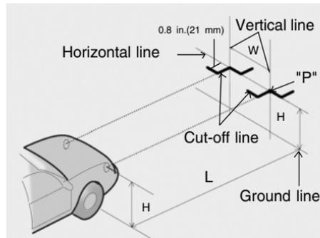
If the vehicle has had front body repair and the headlight assembly has been replaced, the headlight aiming should be checked using the aiming screen as shown in the illustration. Turn on the headlight switch (Low Beam Position).
