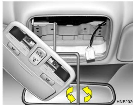
3. Insert the hexagonal head wrench provided with the vehicle into the socket. This wrench can be found in the vehicle's glove box.
