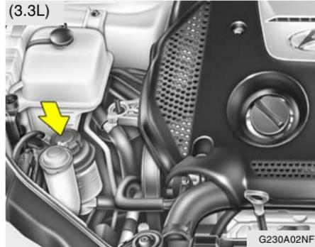
The power steering fluid level should be checked regularly. To check the power steering fluid level, be sure the engine is "OFF", then check
