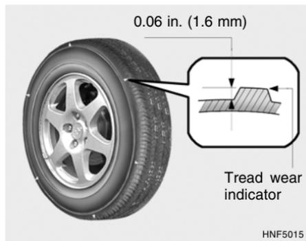
The original tires on your car have tread wear indicators. The location of tread wear indicators is shown by the "TWI" or "△" marks, etc. The tread wear indicators appear when the tread depth is 0.06 in. (1.6 mm). The tire should be replaced when these appear as a solid bar across two or more grooves of the tread. Always replace your tires with those of the recommended size. If you change wheels, the new wheel's rim width and offset must meet Hyundai specification.
