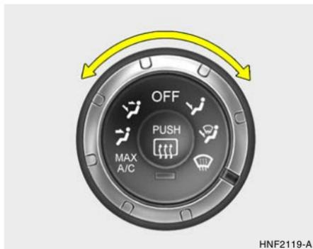
This is used to turn the blower fan on/off and to direct the flow of air. Air can be directed to the floor, dashboard outlets, or windshield. Five symbols are used to represent Face, Bi-Level, Floor, Floor-Defrost and Defrost air position. The MAX A/C mode is used to cool the inside of the vehicle faster. The "OFF" mode is used to turn the blower fan off.
