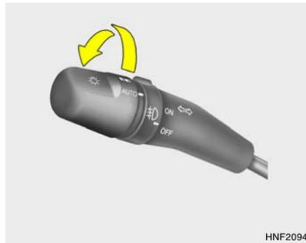
To operate the automatic light feature, turn the barrel on the end of the multi-function switch. If you set the multi-function switch to "AUTO", the tail lights and headlights will be turned automatically on or off according to external illumination conditions.
