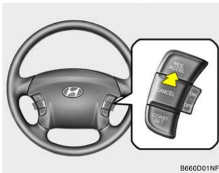
The vehicle will automatically resume the speed set prior to cancellation when you push the control switch "RESUME (ACCEL)" and release it to return (when travelling above 25 mph).
