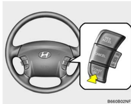
1. Push the control switch "SET (COAST)" and hold it. While the control switch is pushed, the vehicle speed will gradually decrease.
