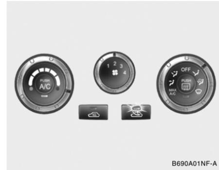
For normal heating operation, set the air flow control to the floor ( ) position. (The "Fresh" mode will be activated.)
