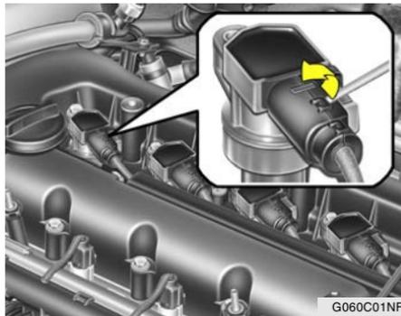
3. Remove the cover of the ignition connector with a flat-head screwdriver.
