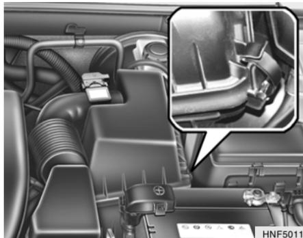
The replacement of the air cleaner filter is performed in the following manner.
