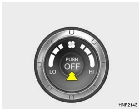
Press the "OFF" button to stop the operation of the heating and cooling system.
