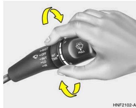
To use the intermittent wiper feature, place the wiper switch in the "INT" position. With the switch in this position, the interval between wipes can be varied from approximately 1 to 18 seconds by turning the interval adjuster barrel.
