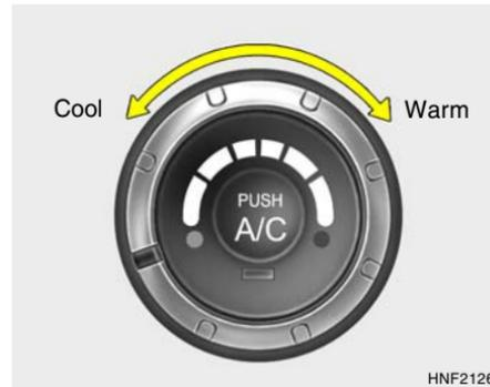
This is used to turn the heating system on and off and to select the degree of heating desired.
