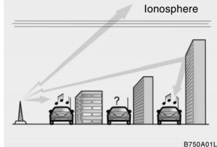
AM and FM radio signals are broadcast from transmitter towers located around your city. They are intercepted by the radio antenna on your car. This signal is then received by the radio and sent to your car speakers.
