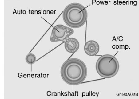
Drive belts should be checked periodically for proper tension and adjusted if necessary. At the same time, belts should be examined for cracks, wear, fraying or other evidence of deterioration and replaced if necessary.
