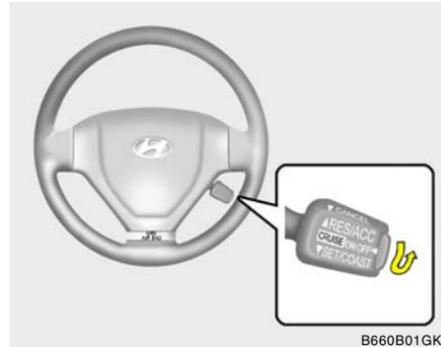
1. Push in the cruise control main switch on the end of the barrel. The "CRUISE" indicator light in the instrument cluster will be illuminated. This turns the system on.
