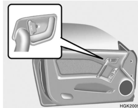
The doors can be locked without a key. To lock the doors first push the inside lock switch to the "LOCK" position so that the red mark on the switch is not visible, then close the door.
