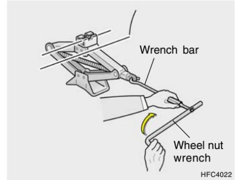
After inserting a bar into the wheel nut wrench, install the bar into the jack as shown in the drawing. To raise the vehicle, turn the jack handle clockwise. As the jack begins to raise the vehicle, double check that it is properly positioned and will not slip. If the jack is on soft ground or sand, place a board, brick, flat stone or other object under the base of the jack to keep it from sinking.
