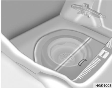
Remove the spare tire and remove the jack and tool bag from the trunk.
