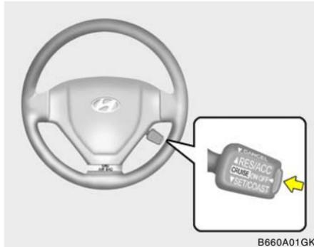
The cruise control system provides automatic speed control for your comfort when driving on freeways, tollroads, or other noncongested highways. This system is designed to function above approximately 25 mph (40 km/h).
