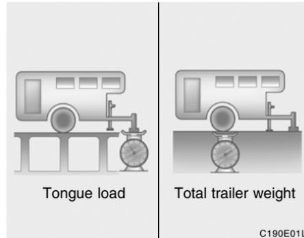
Tongue loads can be increased or decreased by redistributing the load in the trailer. This can be verified by checking the total weight of the loaded trailer and then checking the load on the tongue.
