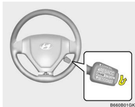
1. Push the control switch downward to "SET (COAST)" and hold it. The vehicle will decelerate.
