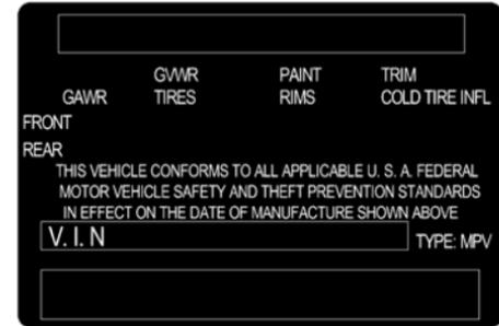
The compliance label is located on the driver's side of the center pillar outer panel.
