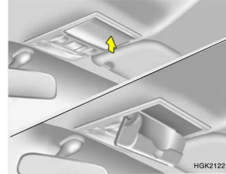
The spectacle case is located on the front overhead console. Push the end of the cover to open or close the spectacle case.
