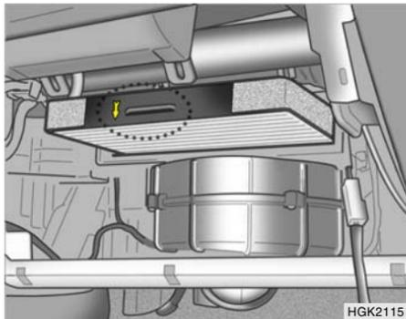
4. Replace the air conditioner filter with a new one.
