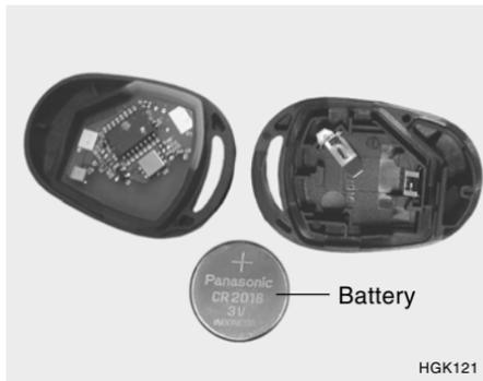
2. Remove the old battery from the case and note the polarity. Make sure the polarity of the new battery is the same (+side facing down), then insert it in the transmitter.
