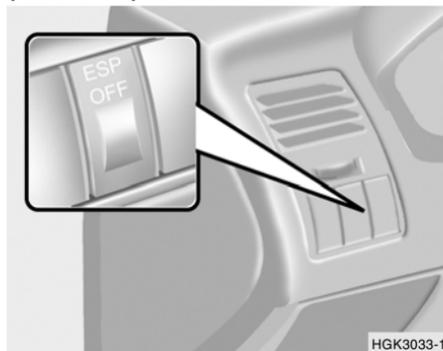
The Electronic Stability Program (ESP) system is designed to stabilize the vehicle during cornering maneuvers. ESP checks where you are steering and where the vehicle is actually going. ESP applies the brakes at individual wheels and intervenes in the engine management system to stabilize the vehicle.
