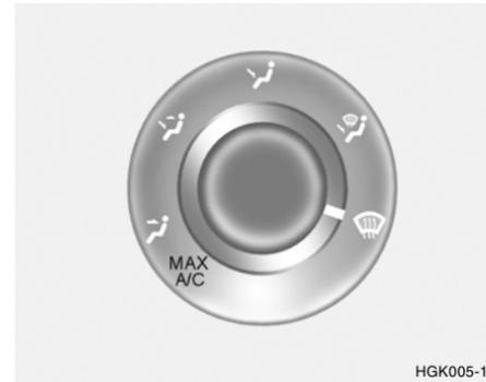
This is used to direct the flow of air. Air can be directed to the floor, instrument panel outlets, or windshield. Five symbols are used to represent Face, Bi-Level, Floor, Floor-Defrost and Defrost air position. The MAX A/C mode is used to cool the inside of the vehicle faster.
