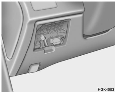
The fuse box for the lights and other electrical accessories will be found low on the dashboard on the driver's side. Inside the box you will find a list showing the circuits protected by each fuse.
