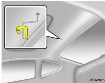
2. Insert the hexagonal head wrench provided with the vehicle into the socket. This wrench can be found in the vehicle's trunk or glove box.
