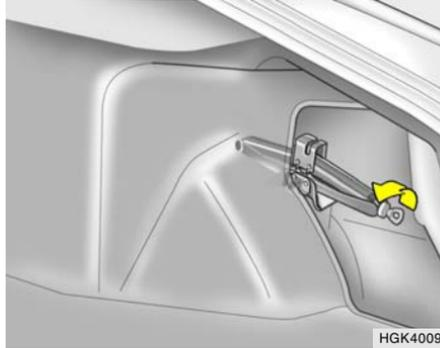
The jack is located behind the right side of luggage trim. Remove the jack cover by unscrewing the bolts. Turn the jack end counterclockwise to lower the jack height by using a screw driver or wrench and remove it from the bracket.
