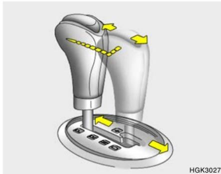
Whether the vehicle is stationary or in motion, sports mode is selected by pushing the selector lever from the "D" position into the manual gate. To return to "D" range operation, push the selector lever back into the main gate.
