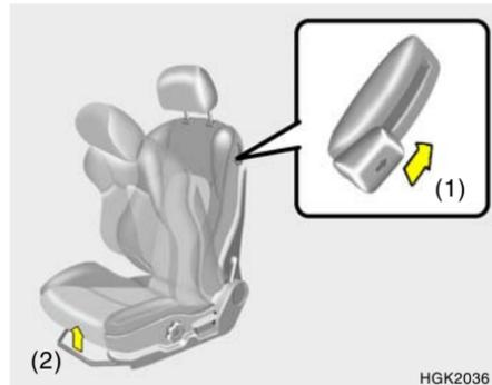
By pulling up the walk in device lever (1) at the left-upper side of the driver side seatback, the seatback will tilt forward. Then pull the lock release lever (2) up to move the seat forward.
