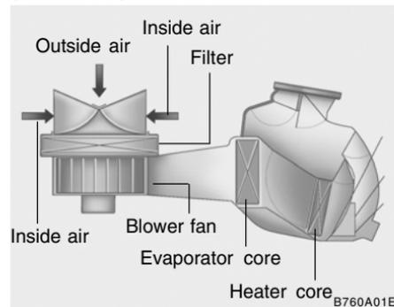
The air conditioner filter is located in front of the blower unit behind the glove box. It operates to decrease the amount of pollutants entering the car. To replace the air conditioner filter, refer to the page 6-20.
