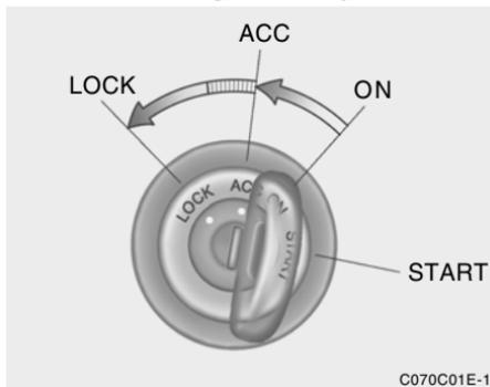
1. Turn the ignition key counterclockwise from the "ACC" position to the "LOCK" position.
