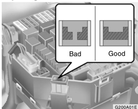
A fusible link will melt if the electrical circuits from the battery are ever overloaded, thus preventing damage to the entire wiring harness. (This could be caused by a short in the system drawing too much current.) If this ever happens, have a Hyundai dealer determine the cause, repair the system and replace the fusible link. The fusible links are located in a relay box(2.0L )or below the positive (+) post cover of the battery (2.7L) for easy inspection.
