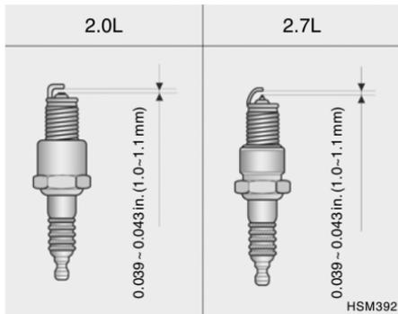
Your engine was originally equipped with platinum-tipped or iridium-tipped spark plugs. Platinum-tipped or iridium-tipped spark plugs will last longer than conventional type spark plugs. Platinum-tipped spark plug can be identified by blue lines on the ceramic shell.
