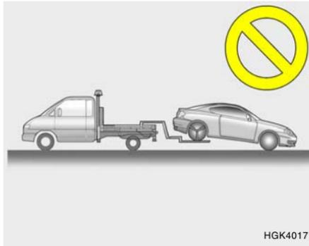
**A vehicle with an automatic transaxle should never be towed from the rear with the front wheels on the ground. This can cause serious damage to the transaxle. Be sure to use a towing dolly under the front wheels.**
