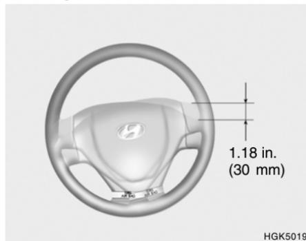
To check the steering wheel free-play, stop the car with the wheels pointed straight ahead and gently move the steering wheel back and forth. Use very light finger pressure and be sensitive to changes in resistance that mark the limits of the free-play. If the free-play is greater than specified, have it inspected by your Hyundai dealer and adjusted or repaired if necessary.
