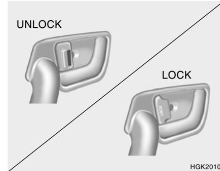
To lock the doors from the inside, simply close the door and push the lock switch to the "LOCK" position. When this is done, neither the outside nor the inside door handle can be used.
