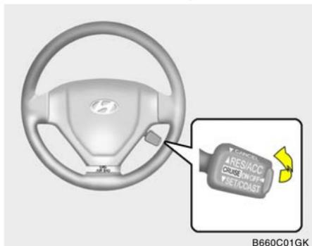
To disengage the cruise control system, pull the control switch toward the steering wheel to "CANCEL" position.
