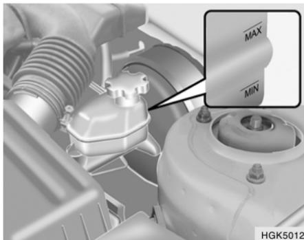
The fluid level in the brake fluid reservoir should be checked periodically. The level should be between the "MIN" and "MAX" marks on the side of the reservoir. If the level is at or below the "MIN" mark, carefully add fluid to bring it up to "MAX". Do not overfill.
