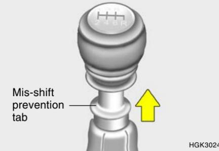
When shifting into reverse gear, pull the mis-shift prevention tab and shift into reverse gear position. (B Type: 6 speed type)
