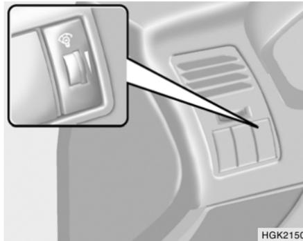
The instrument panel lights can be made brighter or dimmer by turning the instrument panel light control knob.
