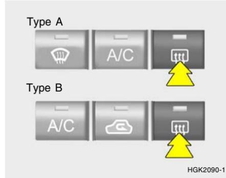
The outside rearview mirror heater is actuated in connection with the rear window defroster. To heat the outside rearview mirror glass, push in the switch for the rear window defroster. The rearview mirror glass will be heated for defrosting or defogging and will give you improved rear vision in inclement weather conditions. Push the switch again to turn the heater off. The outside rearview mirror heater automatically turns itself off after 15 minutes.
