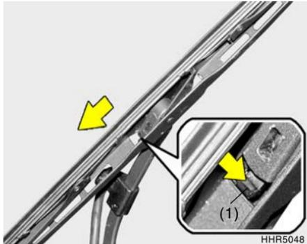
1. Push down the wiper blade with the locking clip (1) pressed to detach it from the wiper arm.
