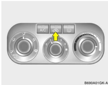
For normal heating operation, set the air intake control to the "Fresh" position and the air flow control to "Floor".
