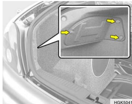
2. To remove the cover of the rear luggage trim, turn the knob by hand to the counterclockwise.
