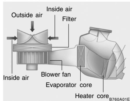
The climate control air filter is located in front of the blower unit behind the glove box. It operates to decrease the amount of pollutants entering the car. To replace the climate control air filter, refer to page 6-18.
