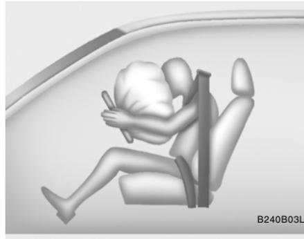
A fully inflated airbag in combination with a properly worn seat belt slows the driver's or the passenger's forward motion, thus reducing the risk of head and chest injury.
