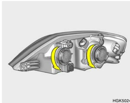
5. Turn the plastic cover counterclockwise and remove it.
