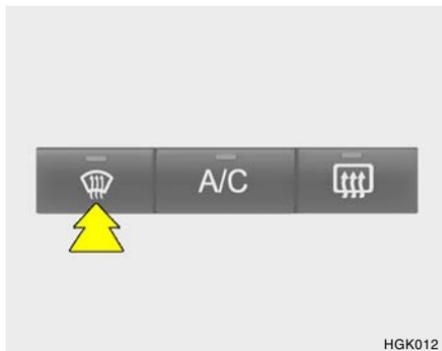
When the "Defrost" button is pressed, the "Defrost" mode will be automatically selected and the air will be discharged through the windshield defrost vents. To assist in defrosting, the air conditioning will operate if ambient temperature is higher than 38.3 °F (3.5 °C) and automatically turns off if the ambient temperature drops below 38.3 °F (3.5 °C).
