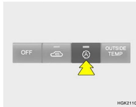
This is used to select fresh outside air or recirculate inside air automatically.
