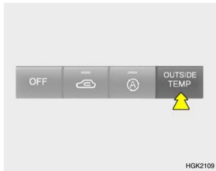
Pressing the **OUTSIDE TEMP** button displays the ambient temperature on the display.
