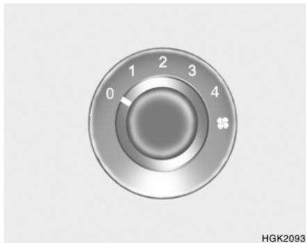
This is used to turn the blower fan on or off and to select the fan speed. This blower fan speed, and therefore the volume of air delivered from the system, may be controlled manually by setting the blower control between the "1" and "4" positions. The "0" position turns the blower fan off.
