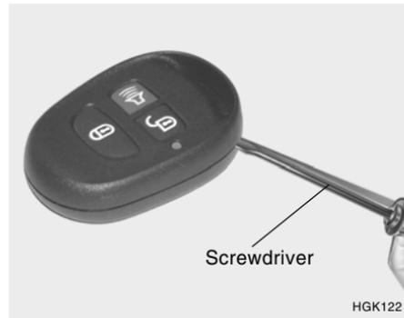
1. Carefully separate the case with a blade screwdriver as shown in the illustration.
