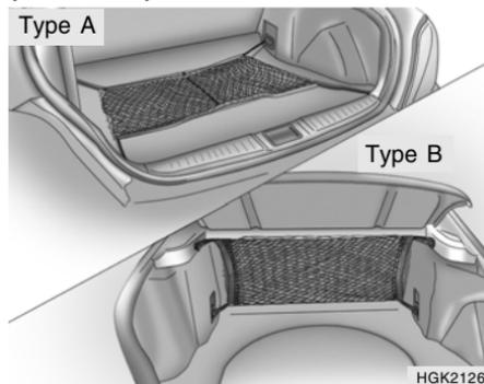
Some objects can be kept in the net in the luggage compartment. Use the luggage net on the floor (if installed) or at the back of the luggage compartment to prevent objects from sliding.
