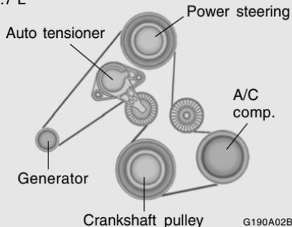
When the air conditioning is being used regularly, the compressor drive belt tension should be checked at least once a month with the engine turned off.
