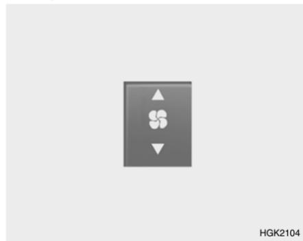
The fan speed can be set to the desired speed by pressing the appropriate fan speed control button. The higher the fan speed is, the more air is delivered. Pressing the "OFF" button turns off the fan.
