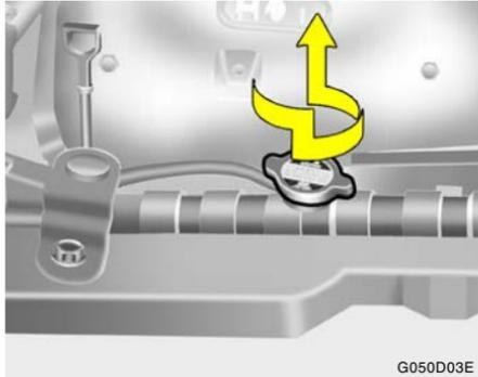
4. Turn the radiator cap counterclockwise without pressing down on it, until it stops. This relieves any pressure remaining in the cooling system. And remove the radiator cap by pushing down and turning counterclockwise.
