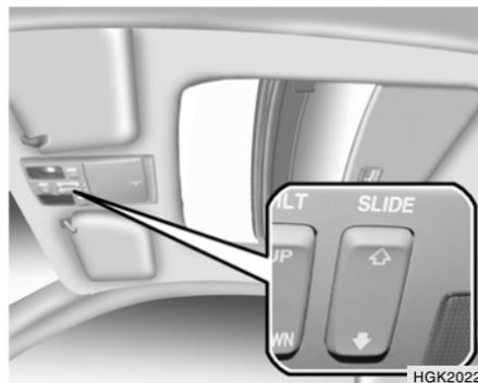
The sunroof can be electrically opened or closed with the ignition key in the "ON" position. The sunroof is moved to its fully open position by pushing the "↑" switch, and to stop at the desired position, push in any switches (↑↓, Up, Down). To close, press and hold the "↓" button. Release the button when the sunroof reaches the desired position.
