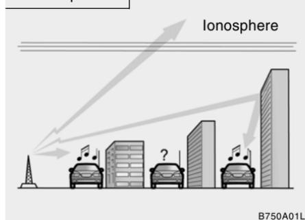
AM and FM radio signals are broadcast from transmitter towers located around your city. They are intercepted by the radio antenna on your car. This signal is then received by the radio and sent to your car speakers.
