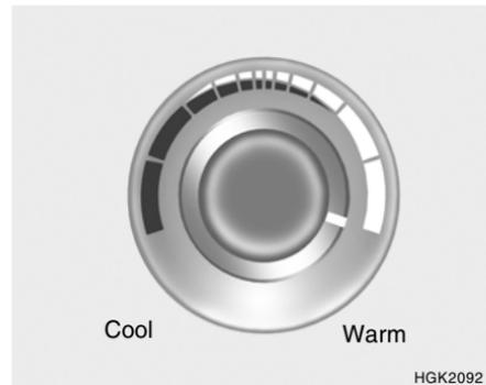
This control is used to adjust the degree of heating or cooling desired.
