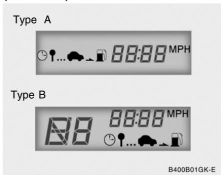
The trip computer is a microcomputer-controlled driver information gauge that displays information related to driving, such as estimated distance to empty, average speed and drive time on the LCD.
