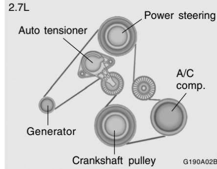
Drive belts should be checked periodically for proper tension and adjusted if necessary. At the same time, belts should be examined for cracks, wear, fraying or other evidence of deterioration and replaced if necessary.
