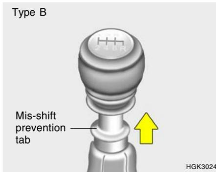
When shifting into reverse gear, pull the mis-shift prevention tab and shift into reverse gear position. (B Type: 6 speed type)
