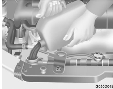
5. Start the engine, top off the radiator with water and then add coolant to the reservoir until the level is between "L" and "F".
