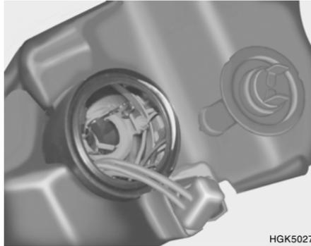
8. Remove the protective cap from the replacement bulb and install the new bulb by matching the plastic base with the headlight hole. Reattach the bulb spring and reconnect the connector.
