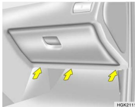
1. Remove the mounting screws on the down-side of the glove box.
