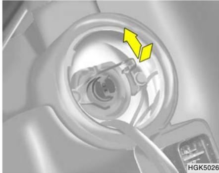
7. Push the bulb spring to remove the headlight bulb.
