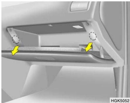
3. Remove the glove box by pulling strongly.
