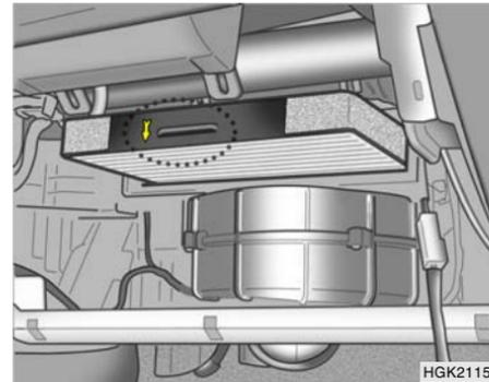
4. Replace the climate control air filter with a new one.
