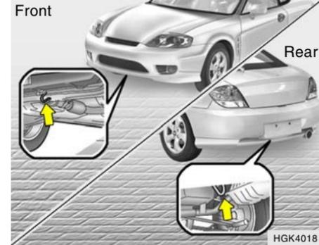
For emergency towing when no commercial tow vehicle is available, attach a tow cable, chain or strap to one of the towing hooks under the front/rear of your car. Do not attempt to tow your vehicle in this manner on any unpaved surface. This could result in serious damage to your car.
