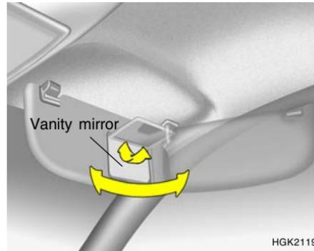
Your Hyundai is equipped with sun visors to give the driver and front passenger either frontal or sideward shade. To reduce glare or to shut out direct rays of the sun, turn the sun visor down. A vanity mirror is provided on the back of the sun visor for the front passenger.
