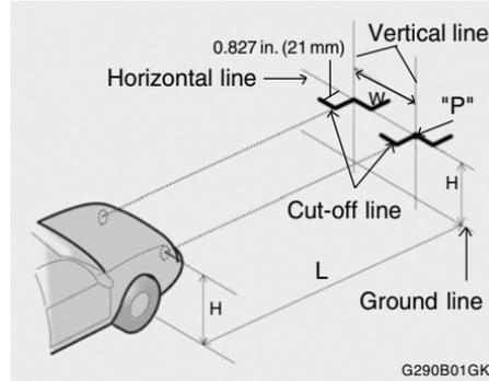
If the vehicle has had front body repair and the headlight assembly has been replaced, the headlight aiming should be checked using an aiming screen as shown in the illustration. Turn on the headlight switch.
