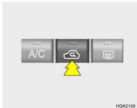
This is used to select fresh outside air or recirculating inside air.
