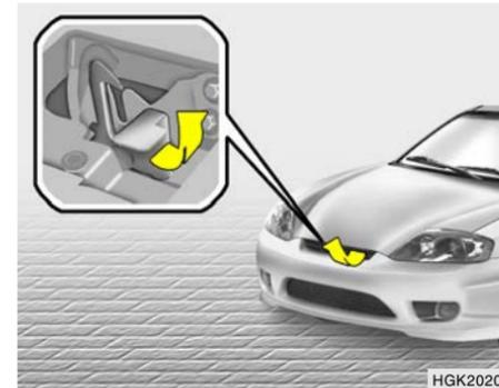
2. Press the safety hook lever up and lift the hood.
