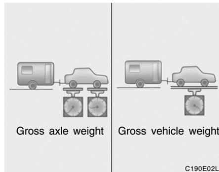
2. **The total gross vehicle weight with trailer must not exceed the Gross Vehicle Weight Rating (GVWR) shown on the vehicle identification plate (see page 8-1). The total gross vehicle weight is the combined weight of the vehicle, driver, all passengers and their luggage, cargo, hitch, trailer tongue load and other optional equipment.**
