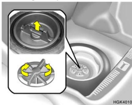
Remove the installation bolt to remove the spare tire. To replace the spare tire in its storage compartment, tighten the bolt firmly with your fingers until there is no more play in the spare tire.
