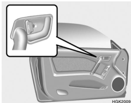
The central door locking is operated by pushing the driver's door lock switch toward the front or rear of the vehicle. If the passenger door is open when the switch is pushed, the door will remain locked when closed.
