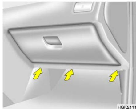
1. Remove the mounting screws on the down-side of the glove box.
