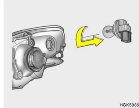
11. To replace the front turn signal light bulb, remove from the bulb holder and install the new bulb.
