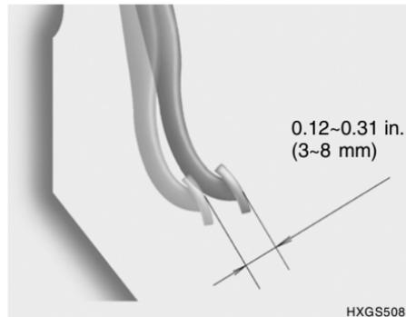
With the engine off, press down on the brake pedal several times to reduce the vacuum in the brake booster. Then, using your hand, press down slowly on the brake pedal until you feel a change in resistance. This is the brake pedal free-play. The free-play should be within the limits specified in the illustration. If it is not, have it inspected by your Hyundai dealer and adjusted or repaired if necessary.
