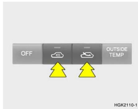
This is used to select fresh outside air or recirculation inside air.
