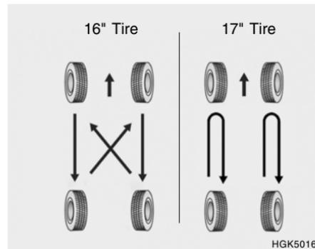
Tires should be rotated every 6,000 miles (10,000 km). If you notice that tires are wearing unevenly between rotations, have the car checked by a Hyundai dealer so the cause may be corrected.
