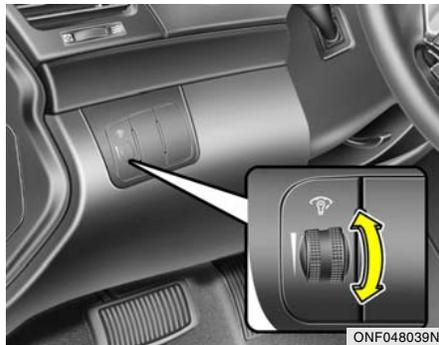
The instrument panel lights can be made brighter or dimmer by turning the instrument panel light control knob.
