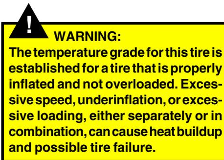
**Uniform Tire Quality Grading** - Quality grades can be found on the tire sidewall between the tread shoulder and the maximum section width. For example :
