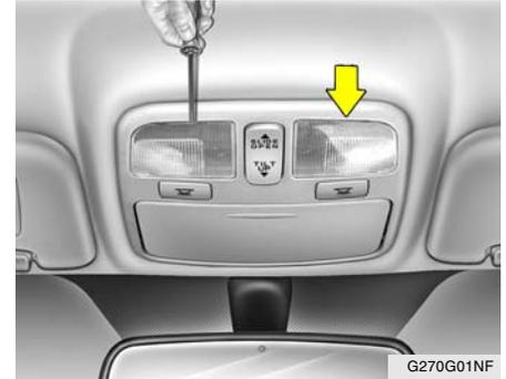
1. Remove the plastic cover with a flat-head screwdriver.
