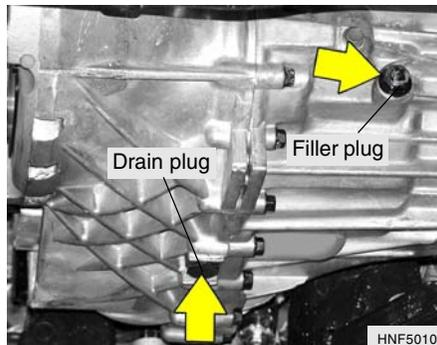
Transaxle lubricant in the manual transaxle should be checked at those intervals specified in the vehicle maintenance schedule in Section 5.
