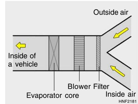
The climate control air filter is located in the right side of the instrument panel. It operates to decrease the amount of pollutants entering the car.
