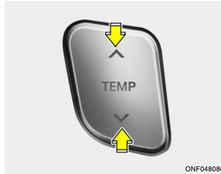
2. Push the "TEMP" button to set the desired temperature. The temperature will increase to the maximum "HI" by pushing the up button. The temperature will decrease to the minimum "LO" by pushing the down button.
