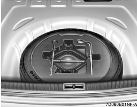
Take out the tool receptacle and turn the installation bolt counterclockwise to remove spare tire from the trunk.
