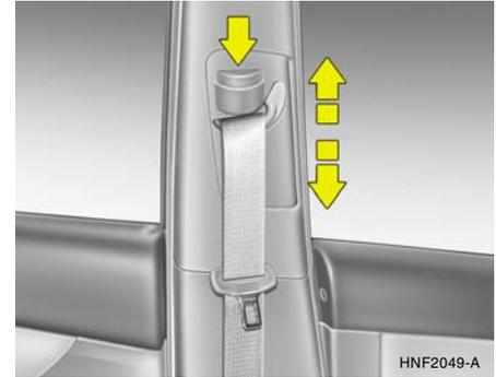
You can adjust the height of the shoulder belt anchor to one of 4 positions for maximum comfort and safety.
