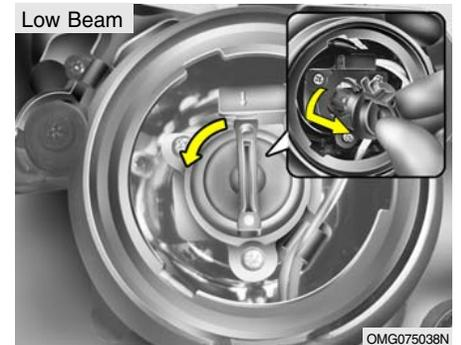
9. Remove the protective cap from the replacement bulb and install the new bulb by matching the plastic base with the headlight hole.
