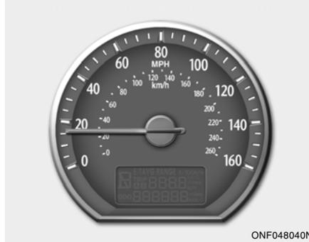
Your Hyundai's speedometer is calibrated in miles per hour and kilometers per hour.
