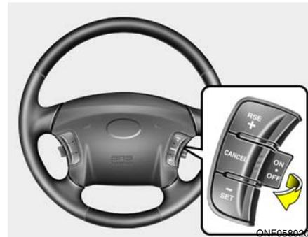
1. Pull the cruise control ON/OFF switch. The "CRUISE" indicator light in the instrument cluster will illuminate. This turns the system on.
