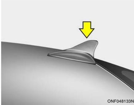
The satellite antenna is installed on the roof of your car to listen to a satellite radio broadcast. This antenna is permanently attached and can not be removed
