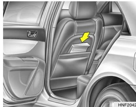
The seatback pockets for holding papers are located on the backside of the front seats.
