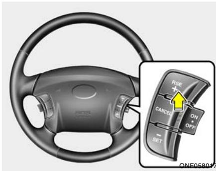
The vehicle will automatically resume the speed set prior to cancellation when you push the control switch "RESUME (+)" and release it to return (when travelling above 25 mph).
