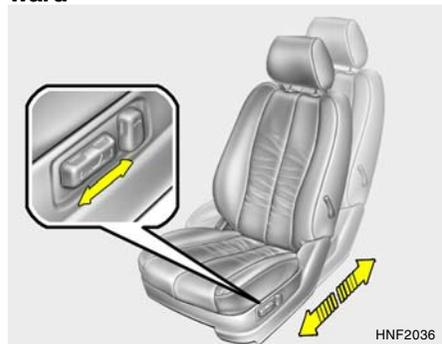
Pull the control knob forward or rearward to move the seat forward or rearward to the desired position. Release the control knob and the seat will remain at that position.
