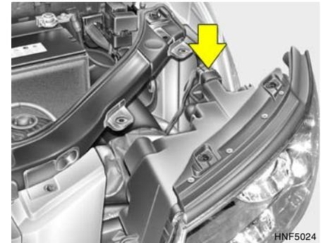
5. Disconnect the power cord from the back of the headlight.
