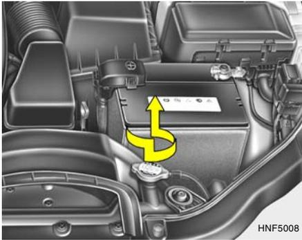
2. Wrap a thick cloth around the radiator cap and slowly turn the radiator cap counterclockwise without pressing down on it, until it stops. This relieves any pressure remaining in the cooling system. When you are sure that all the pressure has been released, remove the radiator cap by pushing down and turning counterclockwise.
