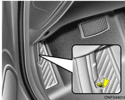
1. Pull the release knob to unlatch the hood.
