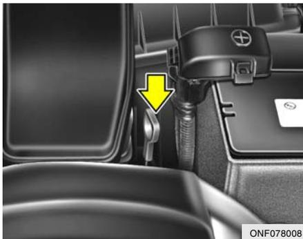
The automatic transaxle fluid level should be checked regularly.
