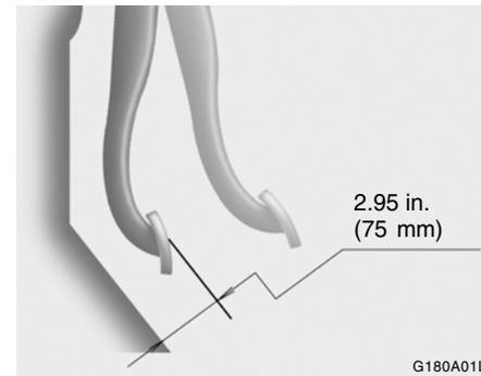
You need a helper to check the brake pedal clearance. With the engine running, have your helper press down on the brake pedal several times and then hold it down with a force of about 110 lbs (50 kg, 490 N). The brake pedal clearance is the distance from the top surface of the brake pedal to the asphalt sheeting under the floor mat. If the brake pedal clearance is not within the limits specified in the illustration, have it inspected by your Hyundai dealer and adjusted or repaired if necessary.
