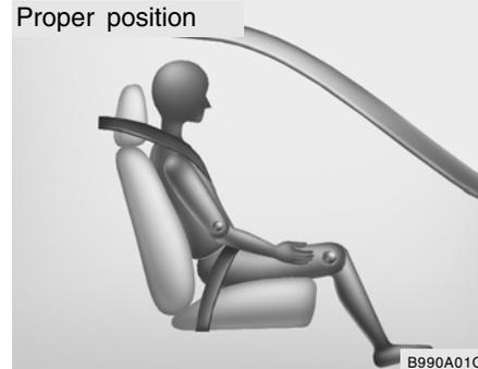
When an adult is seated in the front passenger seat, if the "PASSENGER AIR BAG OFF" indicator is on, turn the ignition key to "LOCK" and ask the passenger to sit properly (sitting upright with the seat back in an upright position, centered on the seat cushion with their seat belt on, legs comfortably extended and their feet on the floor). Restart the engine and have the person remain in that position. This will allow the system to detect the person and to enable the passenger air bag.
