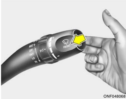
To use the windshield washer, pull the wiper/washer lever toward the steering wheel. When the washer lever is operated, the wipers automatically make two passes across the windshield. The washer continues to operate until the lever is released.
