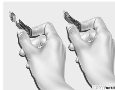
4. Replace the blown fuse by pressing a new fuse of the same rating into place. The fuse should be a snug fit. If it is not, have the fuse clip repaired or replaced by a Hyundai dealer. If you do not have a spare fuse, you may be able to borrow a fuse of the same or lower rating from an accessory you can temporarily get along without (the radio or cigarette lighter, for example). Always remember to replace the borrowed fuse.
