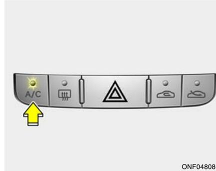
The air conditioning is turned on or off by pushing the A/C button on the heating/air conditioning control panel.
