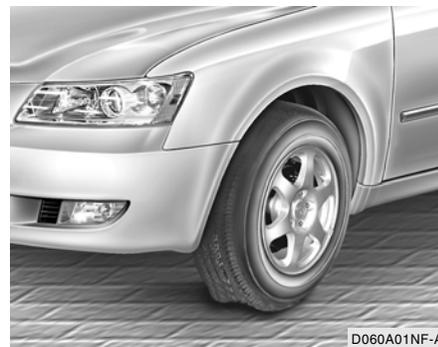
The procedure described on the following pages can be used to rotate tires as well as to change a flat tire. When preparing to change a flat tire, check to be sure the gear selector lever is in "P" (automatic transaxle) or reverse gear (manual transaxle) and that the parking brake is set, then:
