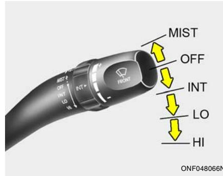
If a single wipe is desired to clear mist, push the windshield wiper and washer control lever upwards.
