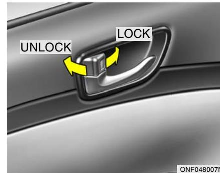
To lock the doors from the inside, simply close the door and push the lock switch to the "LOCK" position.
