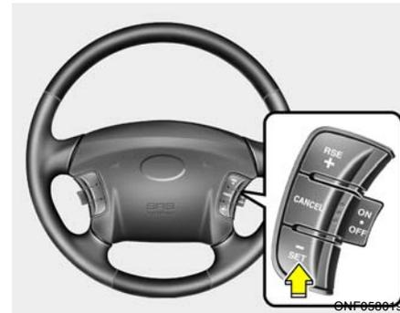
1. Push the control switch "SET (-)" and hold it. While the control switch is pushed, the vehicle speed will gradually decrease.
