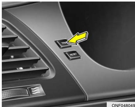
Pushing in the TRIP switch when the ignition switch is in "ON" position changes the display as follows;
