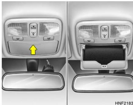
The sunglasses holder is located on the front overhead console. Push the end of the cover to open the sunglasses holder.
