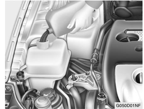
6. Run the engine at idle until the coolant circulates. If the cooling fan operates and the coolant starts to circulate, add the coolant to the reservoir.
