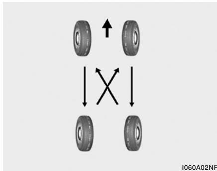
Tires should be rotated every 7,500 miles (12,000 km). If you notice that tires are wearing unevenly between rotations, have the car checked by a Hyundai dealer so the cause may be corrected.
