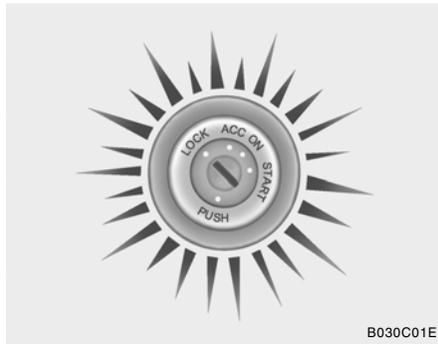
Whenever either front door is opened, the ignition switch will be illuminated for your convenience, provided the ignition switch is not in the "ON" position. The light will go off approximately 10 seconds after closing the door or when the ignition switch is turned on.
