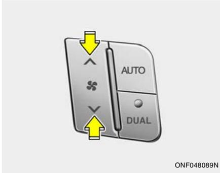
The fan speed can be set to the desired speed by pressing the fan speed control button. The higher the fan speed is, the more air is delivered. Pressing the "OFF" button turns off the fan.
