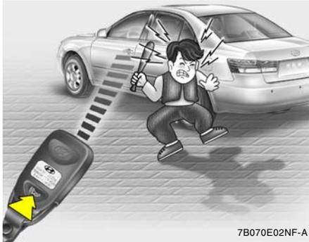
1. Push the "PANIC" button on the backside of the transmitter.
