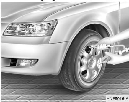
If you have a tire gauge, remove the valve cap and check the air pressure. If the pressure is lower than recommended, drive slowly to the nearest service station and inflate to the correct pressure. If it is too high, adjust it until
