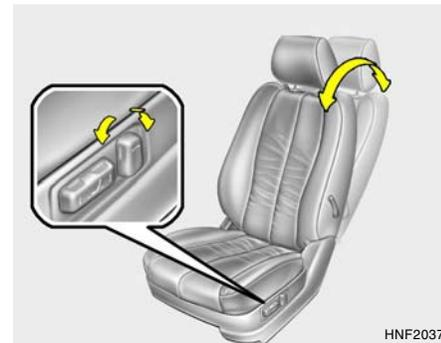
Pull the upper portion of the control knob forward or rearward to recline the seatback to the desired position. Release the control knob and the seatback will remain in that position.
