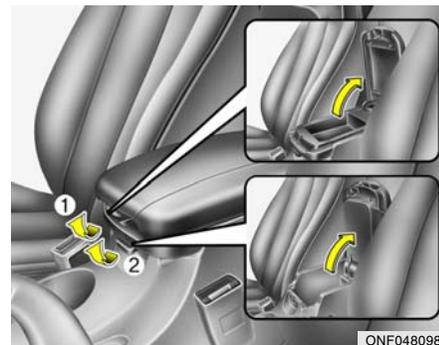
The center console box is used for storing cassette tapes or small articles. To use the center console box, pull up the handle and lift the lid as shown.
