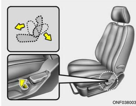
To recline the seatback, lean forward to take your weight off it, then pull up on the recliner control lever at the outside edge of the seat. Now lean back until the desired seatback angle is achieved. To lock the seatback into position, release the recliner control lever.
