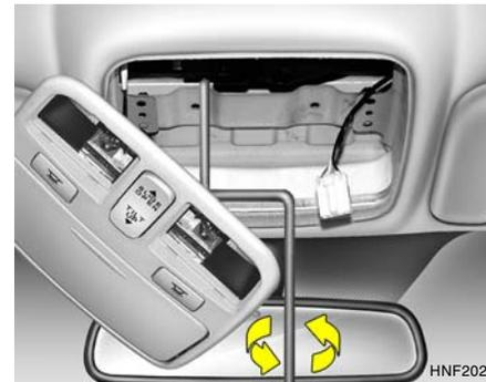
3. Insert the hexagonal head wrench provided with the vehicle into the socket. This wrench can be found in the vehicle's trunk or glove box.
