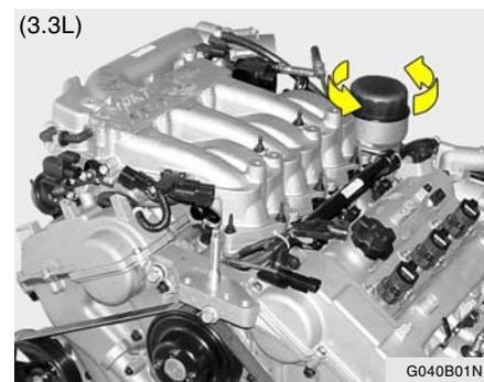
5. Remove the oil filter by turning it counter-clockwise with a oil filter wrench of the proper size. A certain amount of oil will come out when you remove the filter. So be sure to have your drain pan in place underneath it.
