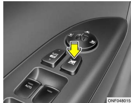
In order to prevent operation of the passenger front and rear windows, a window lock switch is provided on the armrest of the driver's door. To disable the power windows, press the window lock switch. To revert to normal operation, press the window lock switch a second time.
