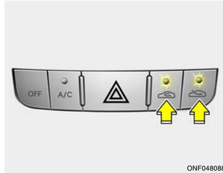
This is used to select fresh outside air or recirculation of inside air. To change the air intake control mode (Fresh mode, Recirculation mode), push the control button.
