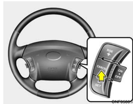
To disengage the cruise control system, push the control switch "CANCEL".
