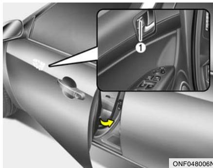
The doors can be locked without a key. To lock the doors from the outside, first push the inside lock switch (1) to the "LOCK" position, so that the red mark on the switch is not visible, then close the door.
