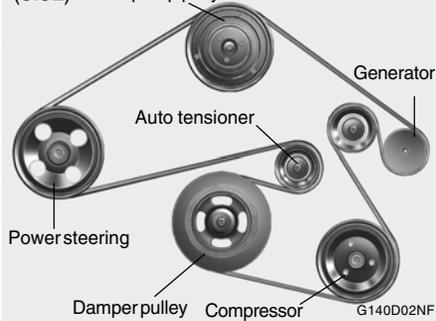
Drive belts should be checked periodically for proper tension. At the same time, belts should be examined for cracks, wear, fraying or other evidence of deterioration and replaced if necessary.
