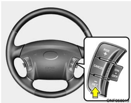
3. Push the "SET (-)" switch after you have set the vehicle speed at the desired speed.
