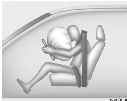
A fully inflated airbag, in combination with a properly worn seat belt, slows the driver's forward motion, reducing the risk of head and chest injury.
