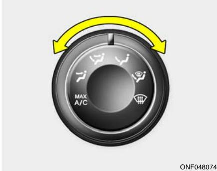
The mode selection knob controls the direction of the air flow through the ventilation system. Air can be directed to the floor, dashboard outlets, or windshield. Five symbols are used to represent Face, Bi-Level, Floor, Floor-Defrost and Defrost air position.
