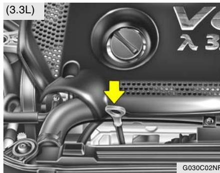
Before checking the oil, warm up the engine to the normal operating temperature and be sure your car is parked on level ground. Turn the engine off.
