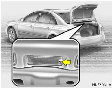
2. Remove the luggage compartment light cover on the rear package tray panel with a flat-head screwdriver.
