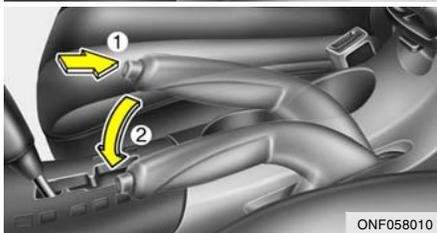
Always engage the parking brake before leaving the vehicle. This also turns on the parking brake indicator light when the key is in the "ON" or "START" position. Before driving away, be sure that the parking brake is fully released and the indicator light is off.
