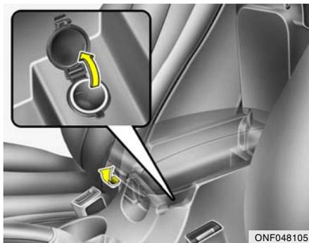
These supply 12V electric power to operate electric accessories or equipment only when the key is in the "ON" or "ACC" position.
