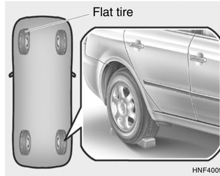
Block the wheel that is diagonally opposite from the flat to keep the vehicle from rolling when the car is raised on the jack.
