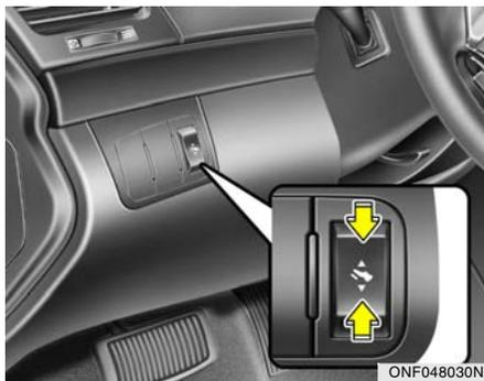
To adjust the position of the accelerator and brake pedals, turn the ignition key to the "ON" position with the selector lever in the "P" position and push the switch.
