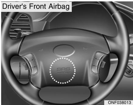
Your Hyundai is equipped with an advanced Supplemental Restraint (Airbag) System. The indications of the system's presence are the letters "SRS AIRBAG" embossed on the airbag pad cover in the steering wheel and the passenger's side front panel pad above the glove box.
