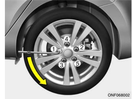
The wheel nuts should be loosened slightly before raising the car. To loosen the nuts, turn the wrench handle counterclockwise. When doing this, be sure that the socket is seated completely over the nut so it cannot slip off. For maximum leverage, position the wrench so the handle is to the left as shown in the drawing. Then, while holding the wrench near the end of the handle, push down on it with steady pressure. Do not remove the nuts at this time. Just loosen them about one-half turn.
