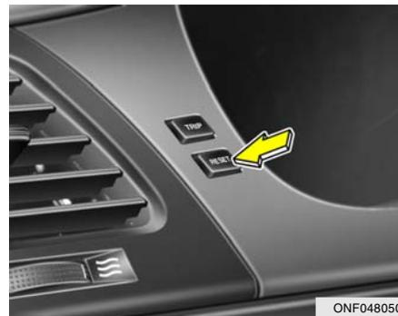
Push in the RESET switch more than 1 second to initialize the displayed information such as tripmeter, average fuel consumption and drive time.
