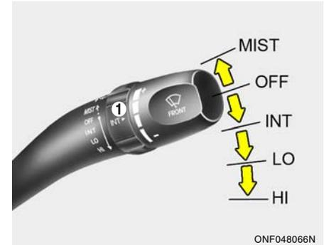
To use the intermittent wiper feature, place the wiper switch in the "INT" position. With the switch in this position, the interval between wipes can be varied from approximately 1 to 18 seconds by turning the interval adjuster barrel (1).
