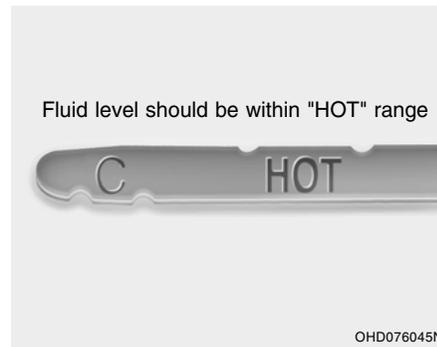
3. Confirm that the fluid level is in “HOT” range on the level gauge. If the fluid level is lower, add the specified fluid from the fill hole. If the fluid level is higher, drain the fluid from the drain hole.
