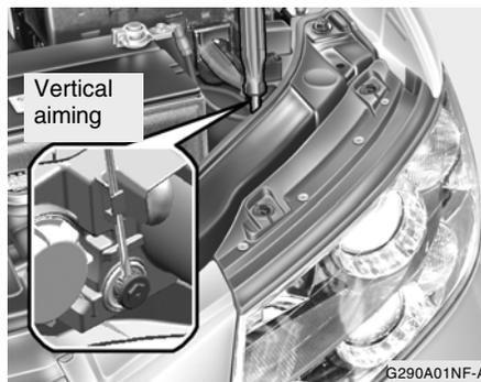
6. Draw a vertical line (through the center of each headlight beam pattern) and a horizontal line (through the center of each headlight beam pattern) on the aiming screen measured from ground to center mark on headlight lens.
