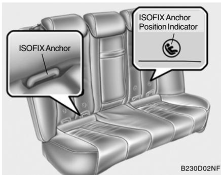
The ISOFIX anchors are located between the seatback and the seat cushion of the rear seat left and right outboard seating positions.
