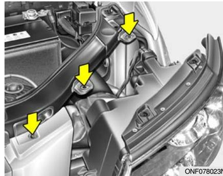
4. Using a socket wrench of the correct size, remove the headlight assembly mounting bolts and bumper mounting bolt.
