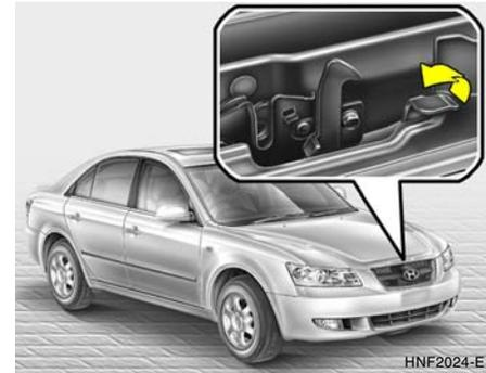
2. Pull the secondary latch up and lift the hood.
