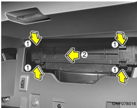
3. Remove the climate control air filter case by pulling out the cover.
