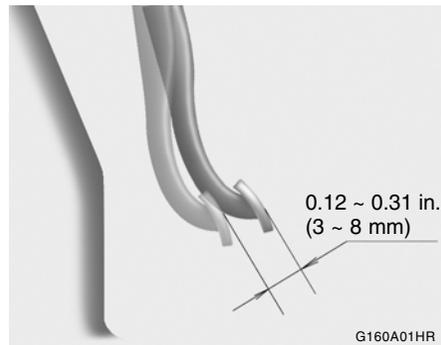
With the engine off, press down on the brake pedal several times to reduce the vacuum in the brake booster. Then, using your hand, press down slowly on the brake pedal until you feel a change in resistance. This is the brake pedal free-play. The free-play should be within the limits specified in the illustration above. If it is not, have it inspected by your Hyundai dealer and adjusted or repaired if necessary.
