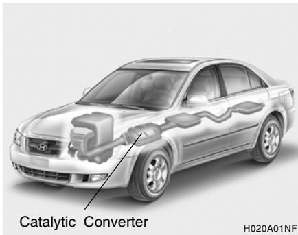
Hyundai vehicle is equipped with a monolith type three-way catalytic converter to reduce the carbon monoxide, hydrocarbons and nitrogen oxides contained in the exhaust gas. Exhaust gases passing through the catalytic converter cause it to operate at a very high temperature. The introduction of large amounts of unburned gasoline into the exhaust may cause the catalytic converter to overheat and create a fire hazard. This risk may be reduced by observing the following:
