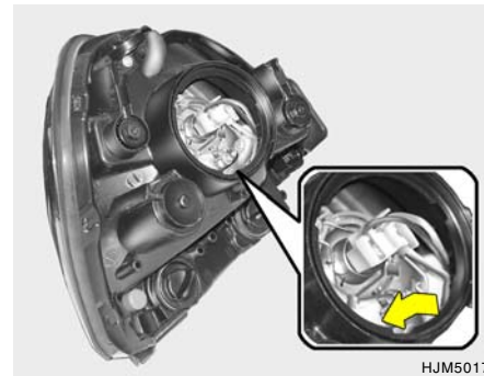
7. Disconnect the connector from the bulb base in the back of the headlight.
