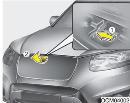
2. Go to the front of the vehicle, raise the hood slightly, push the secondary latch (1) inside of the hood center and lift the hood (2).
