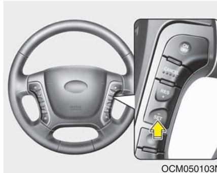
3. Push the -SET switch, and release it at the desired speed. The SET indicator light in the instrument cluster will illuminate. Release the accelerator at the same time. The desired speed will automatically be maintained.
