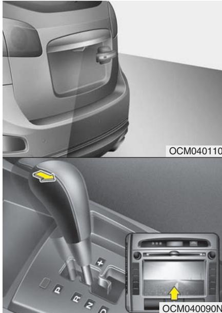
The rearview camera will activate when the back-up light is ON with the ignition switch ON and the shift lever in the R (Reverse) position.
