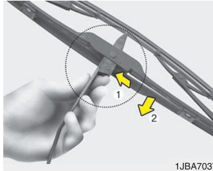
2. Compress the clip and slide the blade assembly downward.
