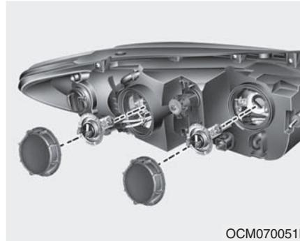
4. Remove the headlight bulb cover by turning it counterclockwise.
