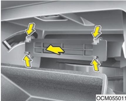
3. Remove the climate control air filter case by pulling out both sides of the cover.
