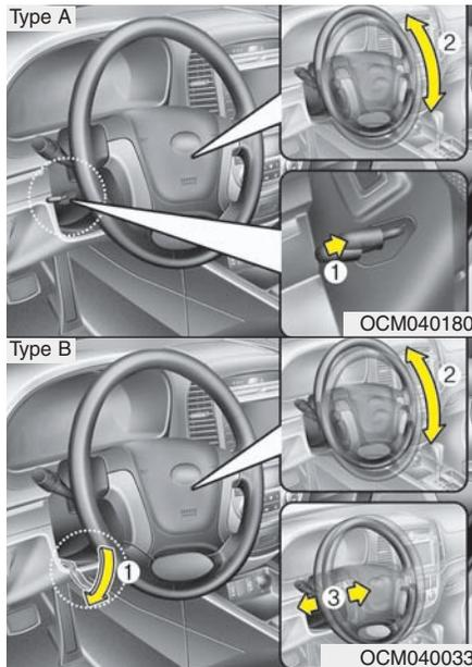
To change the steering wheel angle, pull down the lock release lever (1), adjust the steering wheel to the desired angle (2) and height (if equipped) (3), then pull up the lock-release lever to lock the steering wheel in place. Be sure to adjust the steering wheel to the desired position before driving.
