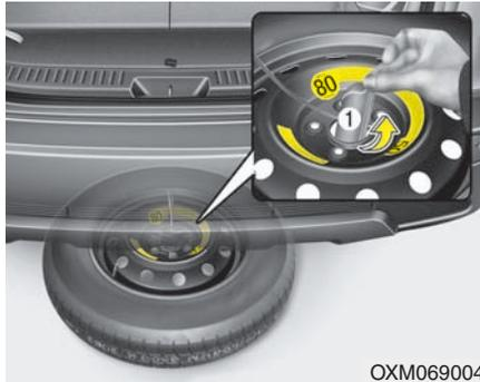
4. After the spare tire reaches the ground, continue to turn the wrench counterclockwise, and draw the spare tire outside. Never rotate the wrench excessively, otherwise the spare tire carrier may be damaged.
