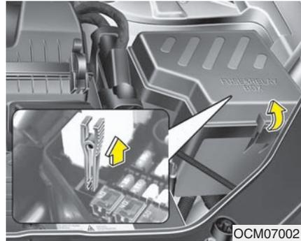
3. Pull the suspected fuse straight out. Use the removal tool provided in the engine compartment fuse panel.
