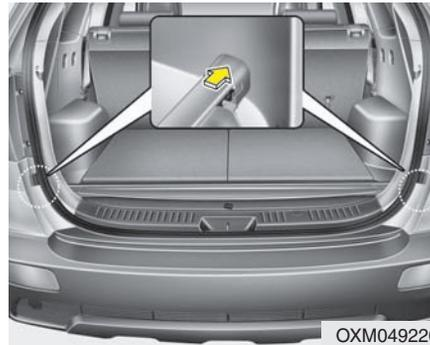
When not in use, place the cargo security screen on the lower portion of the cargo area. (if equipped)
