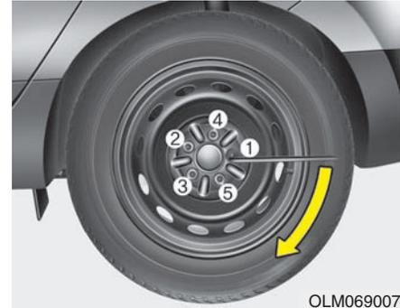
Then position the wrench as shown in the drawing and tighten the wheel nuts. Be sure the socket is seated completely over the nut. Do not stand on the wrench handle or use an extension pipe over the wrench handle. Go around the wheel tightening every nut following the numerical sequence shown in the image until they are all tight. Then double-check each nut for tightness. After changing wheels, have an authorized HYUNDAI dealer tighten the wheel nuts to their proper torque as soon as possible.
