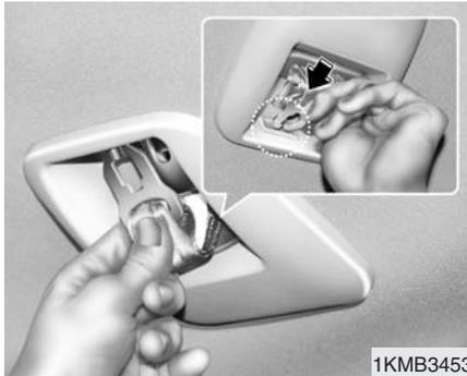
3. Insert the tongue plate (A) into the hole on the belt assembly cover.
