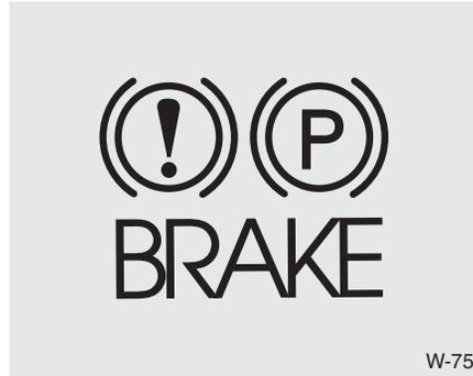
Check the brake warning light by turning the ignition switch ON (do not start the engine). This light will be illuminated when the parking brake is applied with the ignition switch in the START or ON position.
