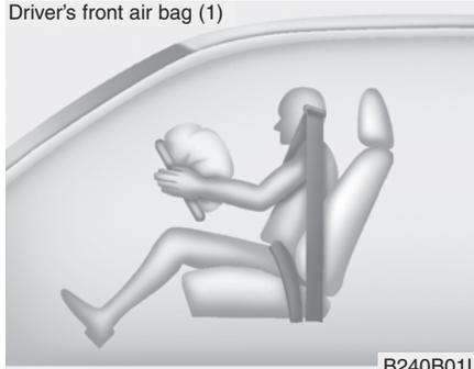
The front air bag modules are located both in the center of the steering wheel and in the front passenger's panel above the glove box. When the SRSCM detects a sufficiently severe impact to the front of the vehicle, it will automatically deploy the front air bags.
