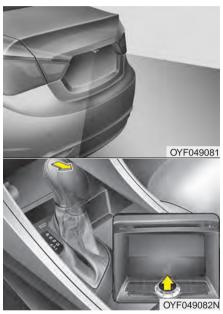
The rearview camera will activate when the back-up light is ON with the ignition switch ON and the shift lever in the R position.
