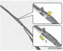
2. Lift up the wiper blade clip. Then pull down the blade assembly and remove it.
