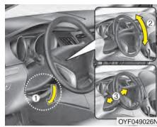
To change the steering wheel angle, pull down the lock release lever (1), adjust the steering wheel to the desired angle (2) and height (if equipped) (3), then pull up the lock-release lever to lock the steering wheel in place. Be sure to adjust the steering wheel to the desired position before driving.
