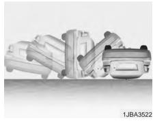
Front air bags may not inflate in rollover accidents because air bag deployment would not provide protection to the occupants.
