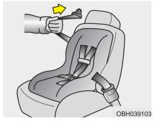
4. Slowly allow the shoulder portion of the seat belt to retract and listen for an audible "clicking" or "ratcheting" sound. This indicates that the retractor is in the "automatic locking" mode. If no distinct sound is heard, repeat steps 3 and 4.
