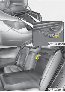
5. Pull on the seatback folding lever located in the trunk, then fold the seat toward the front of the vehicle.
