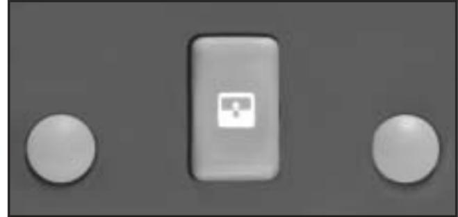
The vehicle may have a power sliding sunroof. To operate it, the ignition or RAP must be in the ON position. The switch used to operate the sunroof is located in the overhead console.
