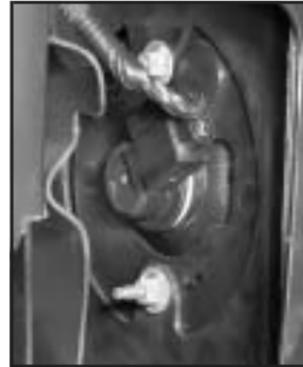
1. Locate the lamp assembly behind the front bumper. It is easiest to come in from the side of the vehicle through the wheel opening.
