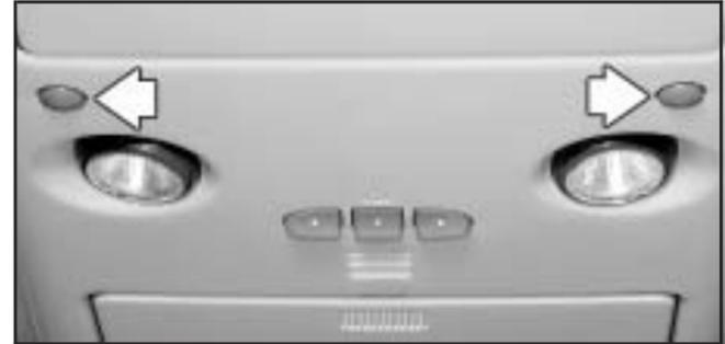
Your vehicle has reading lamps located in the overhead console. Press the button located next to the lamp to turn it on. The lamps can be adjusted to point in the direction you want.
