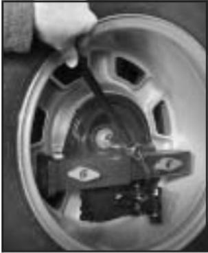
3. Place the end of the spanner wrench on the nut and then turn the wheel wrench counterclockwise to loosen the nut holding the tire to the carrier.
