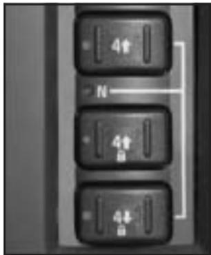
The transfer case buttons are located to the right of the instrument panel cluster. Use these switches to shift into and out of the different all-wheel drive modes.
