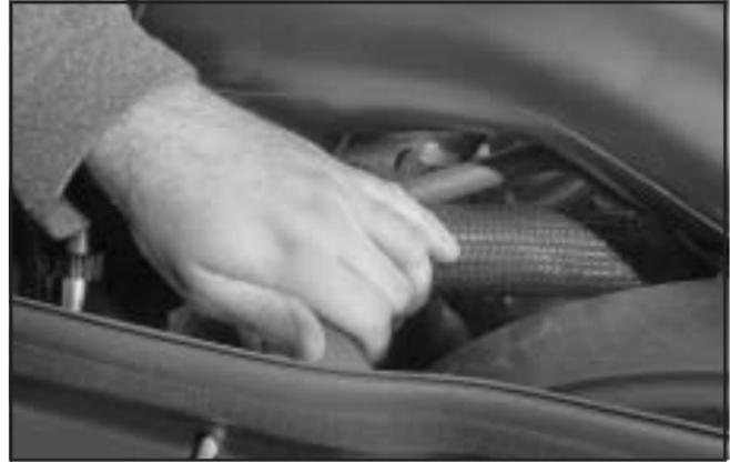
5. With the coolant surge tank pressure cap off, start the engine and let it run until you can feel the upper radiator hose getting hot. Watch out for the engine cooling fan.
