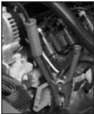
The remote positive (+) terminal is located near the engine accessory drive bracket. On some vehicles, the terminal may be covered by a red plastic cover. To access the remote positive (+) terminal, open the cover.
