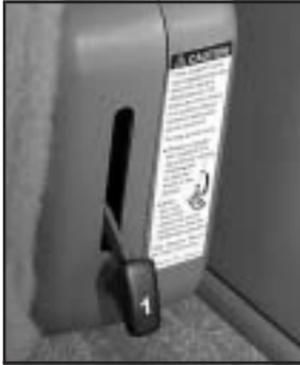
5. Pull up on the release lever labeled 1 and then pull up on the seatback until the seatback locks into the upright position.
