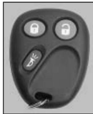
**i (Unlock):** Press this button once to unlock the driver's door. The interior lamps will come on. Pressing unlock again within three seconds will cause the remaining doors to unlock.
