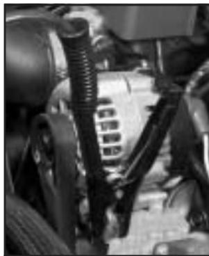
The remote negative (-) terminal is located on the engine accessory drive bracket and is marked GND.
