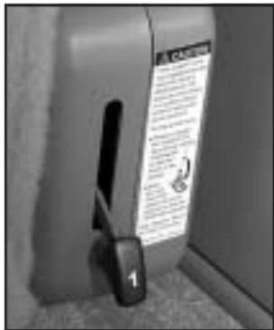
1. Pull up on the release lever labeled 1 and then pull up on the seatback until the seatback locks into the upright position.
