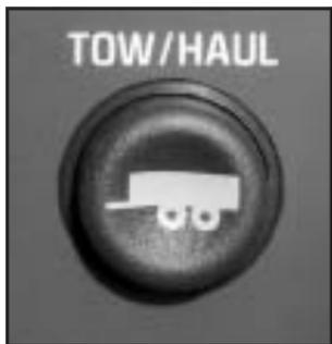
Press the button on the instrument panel to the right of the steering wheel to enable the tow/haul mode.
