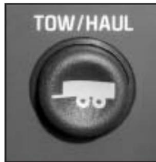
Your vehicle is equipped with a tow/haul mode. The button is located on the instrument panel to the right of the steering wheel.
