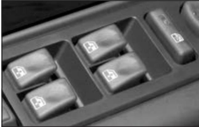
A power window switch is located on the armrest of each side door. The switches operate while the ignition is in RUN or ACCESSORY or while Retained Accessory Power (RAP) is active. See *Retained Accessory Power (RAP)* on page 2-26.
