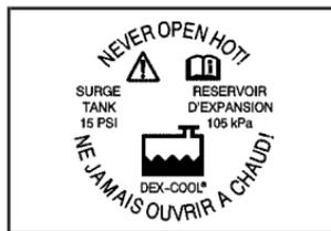
1. Locate the coolant surge tank pressure cap that has this label.
