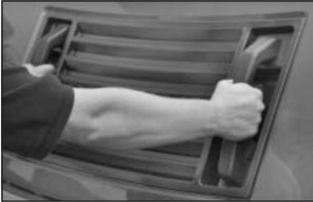
3. Then go to the front of the vehicle and pull the assist handles toward you to lift the hood.
