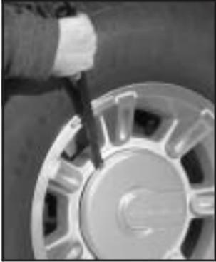
1. To remove the center cap, place the flat end of the wheel wrench in the slot on the wheel and gently pry the center cap out.
