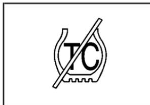
The traction off light will come on when a traction control system or anti-lock brake system problem has been detected. The vehicle may need service.
