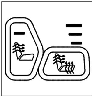
Your vehicle may have heated front seats. The buttons used to control this feature are located on the front doors. The engine must be running for the heated seat feature to work.
