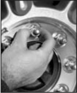
9. After mounting the spare, put the wheel nuts back on with the rounded end of the nuts toward the wheel.
