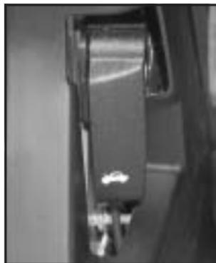
2. Pull the handle located inside the vehicle to the lower left of the steering wheel.
