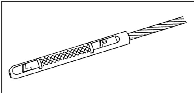
If the oil is below the cross-hatched area (L), you will need to add at least one quart/liter of oil. But you must use the right kind. This section explains what kind of oil to use. For engine oil crankcase capacity, see *Capacities and Specifications on page 422*.
