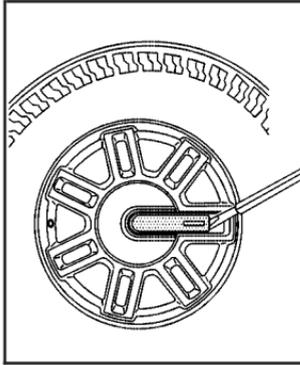
2. Remove the center cap, if equipped, by placing the flat end of the wheel wrench in the slot on the wheel and gently pry the center cap out.
