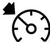
The cruise symbol on the instrument panel comes on when the cruise control is engaged.
