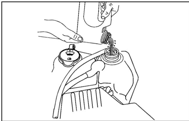
4. Fill the coolant recovery tank to the FULL COLD mark.
