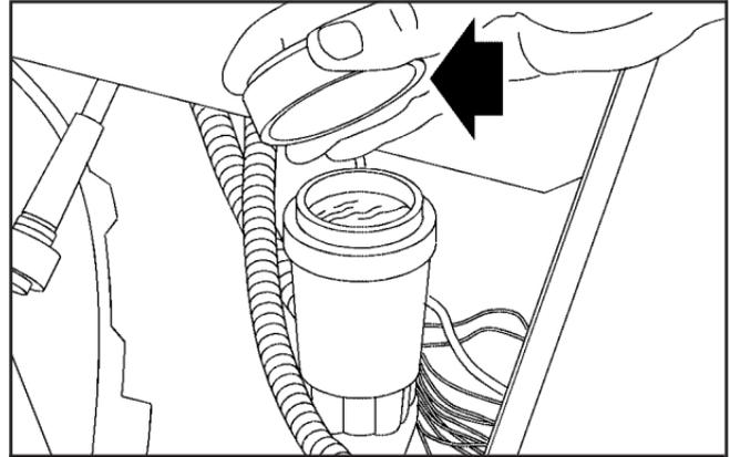
Refer to the Maintenance Schedule to determine how often you should check the fluid level in your clutch master cylinder reservoir and for the proper fluid. See *Recommended Fluids and Lubricants* on page 440.
