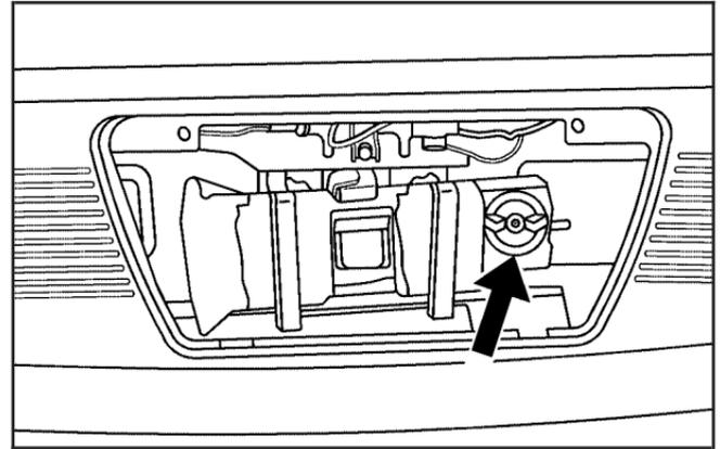
3. Turn the wing nut counterclockwise to release the jack tool bag and jack.
