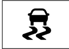
If you have the StabiliTrak<sup>®</sup> system, this light will come on when the StabiliTrak<sup>®</sup> system has been turned off.
