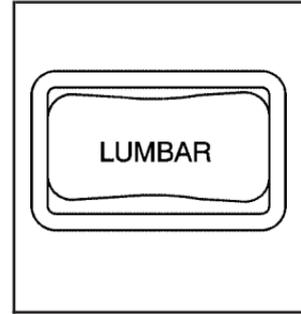
If your vehicle has this feature, the control is located on the outboard side of the seat(s).
