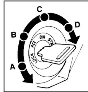
With the key in the ignition switch, you can turn to four different positions.
