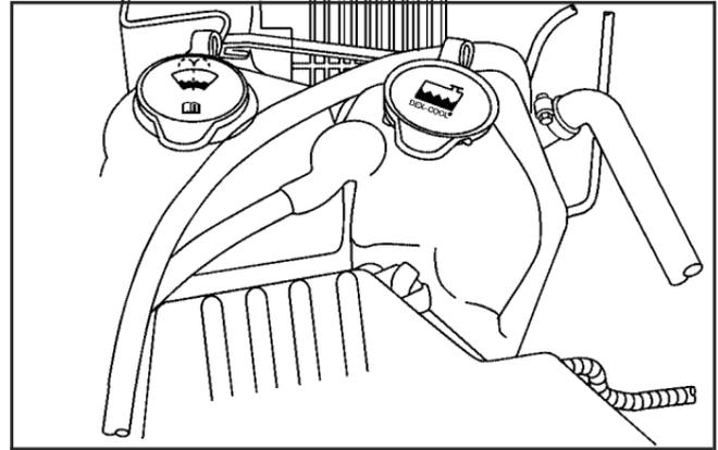
When the engine is cold, the coolant level should be at least up to the FULL COLD mark. If it is not, you may have a leak at the pressure cap or in the radiator hoses, heater hoses, radiator, water pump or somewhere else in the cooling system.
