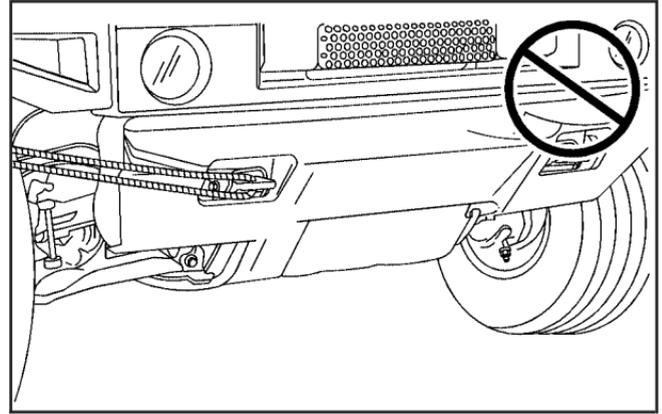
If your vehicle has a brush guard, never tow or apply any loads onto the brush guard.
