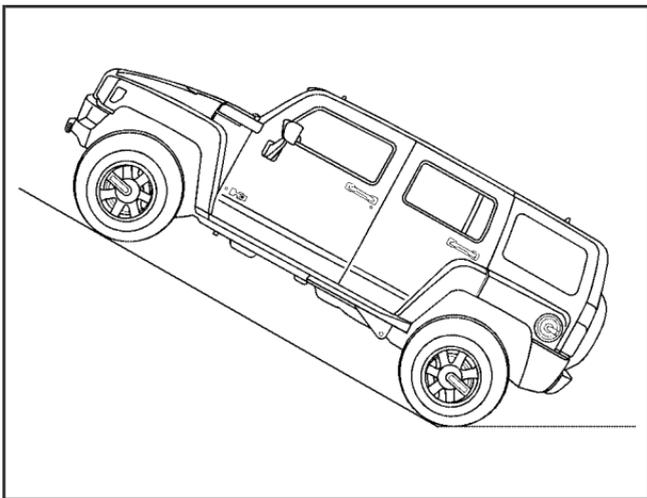
Design specifications required a minimum gradeability of 60% (31 degrees) slope, with the vehicle fully loaded, on high friction surfaces with maximum vehicle speed not to exceed 6 mph (9.7 km/h). The vehicle is expected to traverse this grade only for short durations. Never stop and idle the vehicle or park it on this grade.
