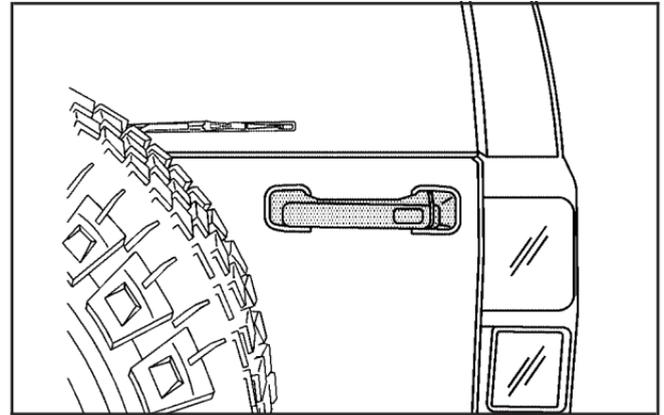
To open the swing-gate, pull the door handle. Pull the swing-gate rearward slightly and it will automatically open.
