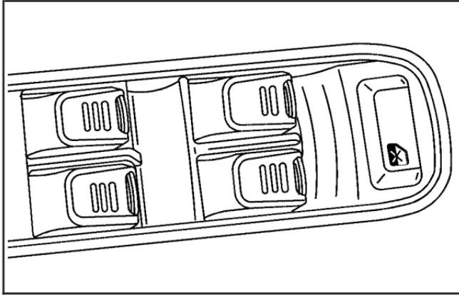
The power window controls are located on the armrest of each door.
