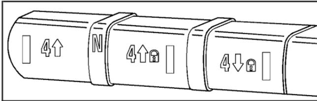
The transfer case buttons are located to the right of the instrument panel cluster. Use these switches to shift into and out of the different Full-Time Four-Wheel Drive modes.
