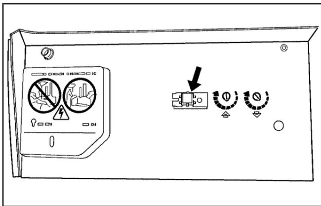
2. Go to the garage. Locate the garage door motor head and press and release the “learn” button.
