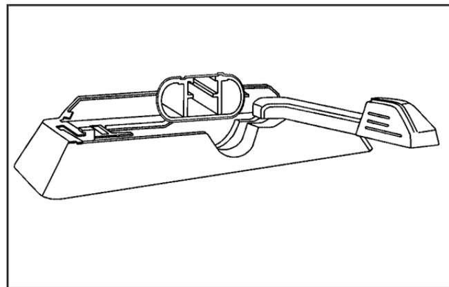
3. Pull the lever labeled "PULL" from left to right to loosen the crossrail.
