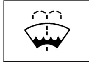
Open the cap with the washer symbol on it. Add washer fluid until the tank is full. See *Engine Compartment Overview on page 322* for reservoir location.
