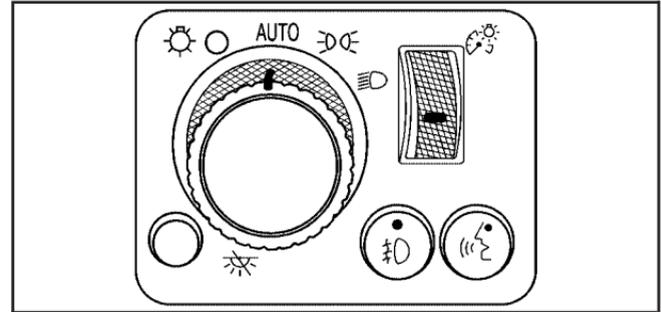
The control on the driver's side of your instrument panel operates the exterior lamps.
