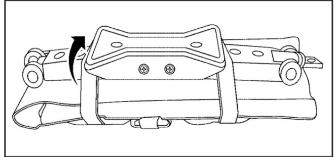
2. Secure the tool bag to the jack by securely wrapping the straps around the jack. Then, slide the straps through the rings on the bag and secure.
