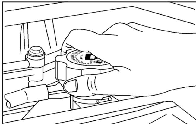
1. Remove the radiator pressure cap when the cooling system, including the upper radiator hose, is no longer hot. Turn the pressure cap slowly counterclockwise about one full turn. If you hear a hiss, wait for that to stop. A hiss means there is still some pressure left.
