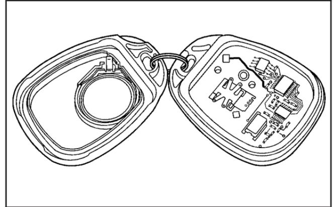
1. Insert a coin, or similar object, in the slot between the covers of the transmitter housing. Gently pry the transmitter apart.
