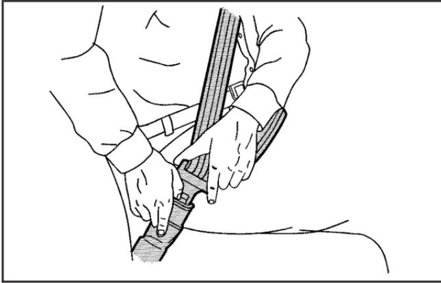
To unlash the belt, push the button on the buckle. The belt should go back out of the way. When the safety belt is not in use, slide the latch plate up the safety belt webbing. The latch plate should rest on the stitching on the safety belt, near the guide loop on the side wall.
