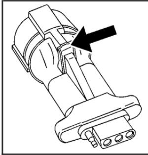
Use this adapter to connect a standard four-way pin connector to the seven-wire harness on your vehicle.
