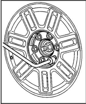
4. Use the wheel wrench to tighten the nuts firmly. Try to move the tire back and forth slightly to be sure it is secure.
