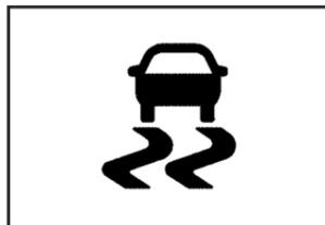
This light will come on steady when the traction control system has been turned off. This light flashes when TCS is active.
