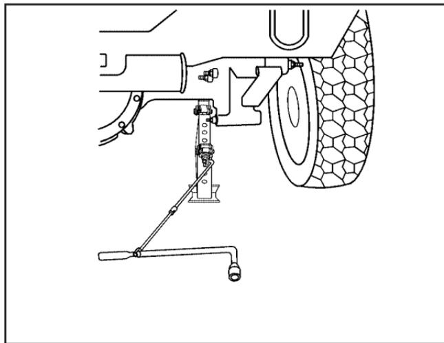
**Rear Tire Flat:** You will need to use the jack handle and both jack handle extensions. Attach the wheel wrench to the jack extensions. Attach the jack handle to the jack. From the rear of the vehicle align the jack under the rear axle. Turn the wheel wrench clockwise to raise the vehicle. Raise the vehicle far enough off the ground so there is enough room for the spare tire to clear the ground.
