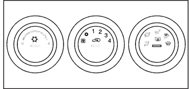
This system controls the heating, cooling, and ventilation of the vehicle. In-between modes are available by moving the right control knob between modes with symbols. The in-between mode will be a combination of the two modes that the control is centered between.
