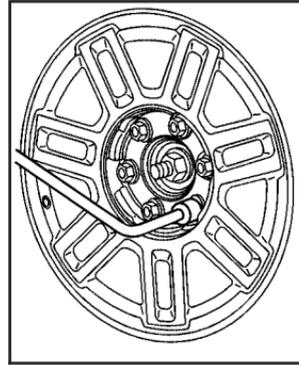
2. Turn the wheel wrench counterclockwise to loosen the wheel nuts. Do not remove them yet.
