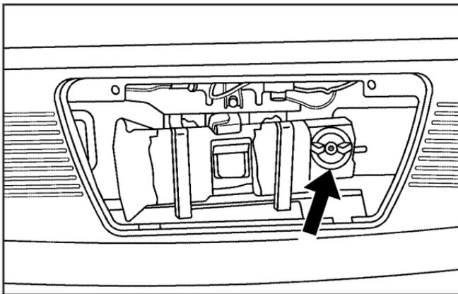
4. Reinstall the wing nut retainer to fasten the jack and tool bag in the storage compartment. Make sure that the wing nut passes through the tool bag and the jack before you tighten it.
