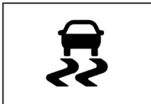
To turn the system off, press and hold the TCS button for five seconds.
