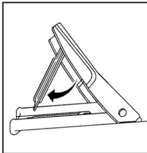
To use the wheel blocks, lift the wheel block as shown and lock into place.
