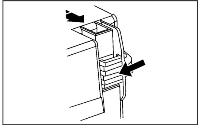
To remove the cover, push in on the tabs at the ends of the cover and lift. To reinstall the cover, line up the tabs and push down on the cover until the tabs clicks into place.
