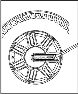
1. Remove the center cap by placing the flat end of the wheel wrench in the slot on the wheel and gently pry the center cap out.
