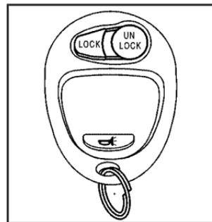
**UNLOCK:** Press this button to unlock the driver’s door and turn on the interior lamps. The parking lamps may also flash, and the horn may chirp, when this button is pressed.
