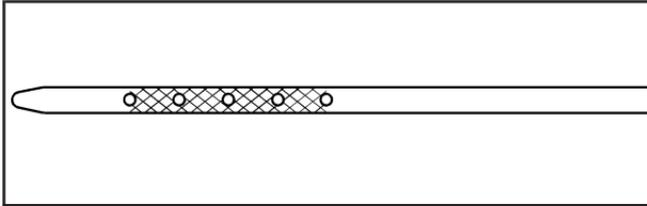
If the oil is below the cross-hatched area at the tip of the dipstick, add at least one quart/liter of the recommended oil. This section explains what kind of oil to use. For engine oil crankcase capacity, see *Capacities and Specifications on page 5-117*.
