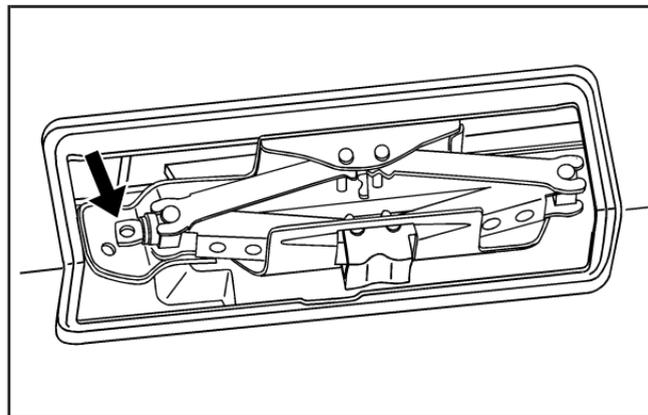
3. Turn the hole at the top of the jack clockwise until the jack is held tight in the mounting bracket.
