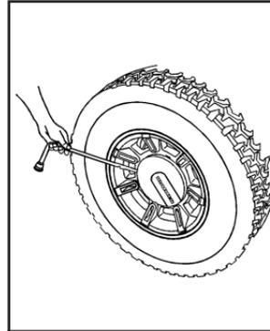
2. To remove the center cap, place the flat end of the wheel wrench in the slot on the wheel and carefully pry the center cap out.
