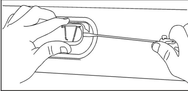
1. Push in on the notch with a flat tool and pull the lamp out.
