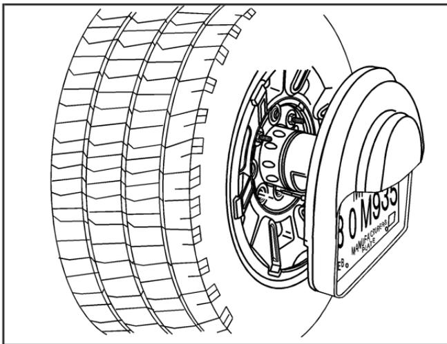
5. Slide the license plate holder onto the spare or flat tire. Secure it from the back of the tire carrier with the wing nut.
