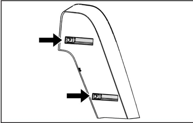
1. To access the jack pull on the two latches to remove the trim cover.
