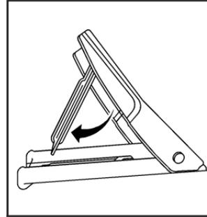
Remove the wheel blocks from the tool bag. Then lift the wheel block as shown to lock it into place.
