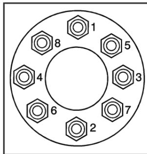
15. Tighten the nuts firmly in a crisscross sequence as shown by turning the wheel wrench with the wheel wrench extender clockwise.
