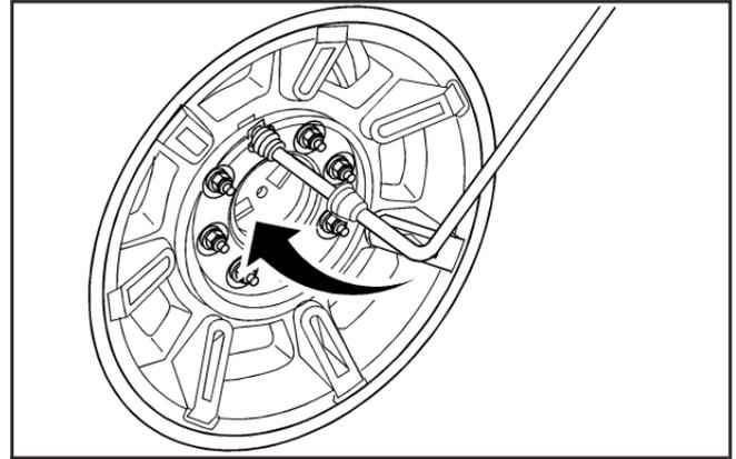
4. Use the wheel wrench and the wheel wrench extension to tighten the nuts firmly. Try to move the tire back and forth slightly to be sure it is secure.
