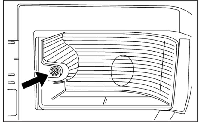
1. Remove the screw and lift off the lens.
