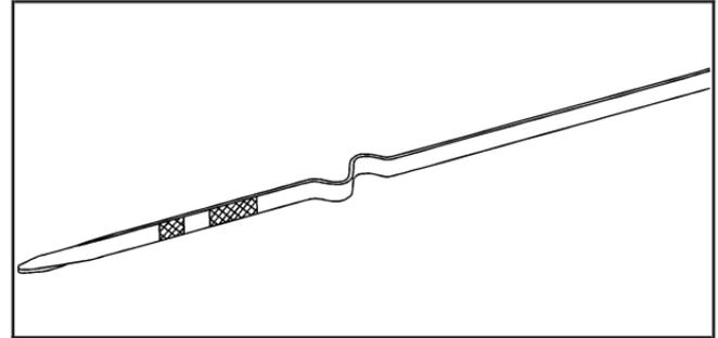
5. Safe operating level is within the HOT cross hatch band on the dipstick. If the fluid level is not within the HOT band, and the transmission temperature is between 160°F and 200°F (71°C and 93°C), add or drain fluid as necessary to bring the level into the HOT band. If the fluid level is low, add only enough fluid to bring the level into the HOT band. It does not take much fluid, generally less than one pint (0.5L). Do not overfill.
