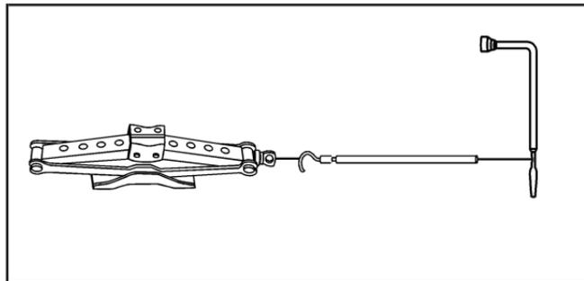
**Front Flat Tire:** Attach the jack handle with the hook end connected to the hole on the jack. Slide the wheel wrench onto the jack handle extension.
