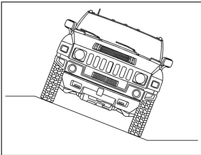
Also, your vehicle should be able to traverse a 40% (22°) side slope at 6 mph (9.7 km/h) while fully loaded on high friction surfaces.
