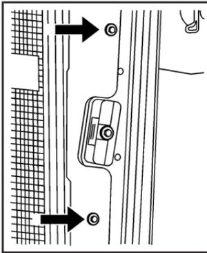
3. Remove the two screws from the rear lamp assembly and remove the rear lamp assembly.
