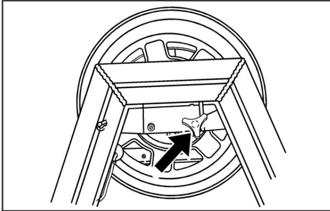
2. Unscrew the wing nut on the back of the tire carrier.
