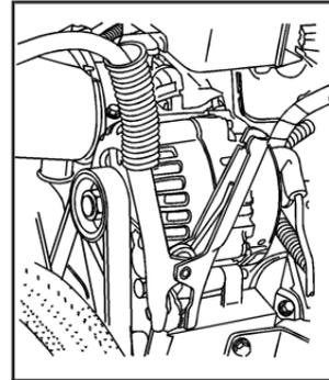
The remote negative (-) terminal is located on the engine accessory drive bracket and is marked GND (Ground).
