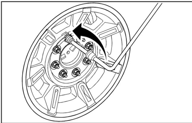
4. Turn the wheel wrench counterclockwise to loosen the wheel nuts. Do not remove them yet.
