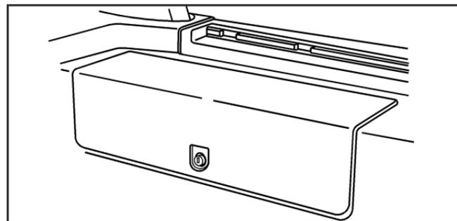
To access the jack, remove the cover, unlock it and then pull the cover off.
