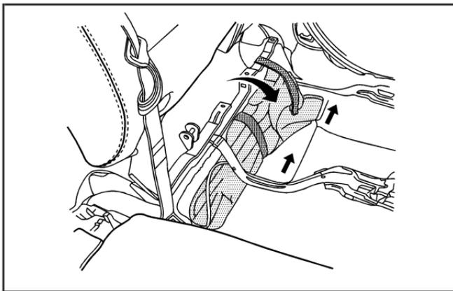
8. Place the narrow end of the tool bag under the seat rails as shown and slide the tool bag under the rear seat.
