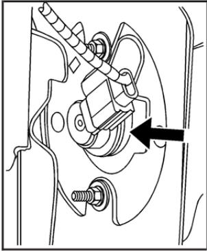
1. Locate the lamp assembly behind the front bumper through the wheel opening.
