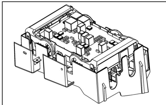
The underhood fuse block in the engine compartment is located on the driver side of the vehicle near the battery. Lift the cover for access to the fuse/relay block.
