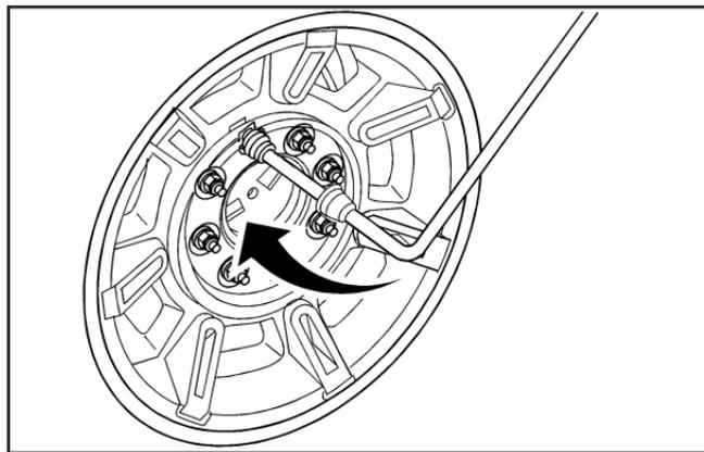
13. Tighten each wheel nut by hand. Then use the wheel wrench to tighten the nuts by turning it clockwise until the wheel is held against the hub. You will not be tightening the nuts fully yet.
