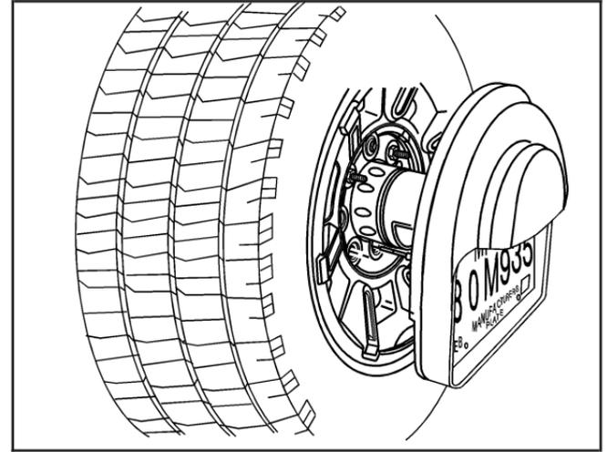
6. Slide the license plate holder onto the spare or flat tire. Secure it from the back of the tire carrier with the wing nut.
