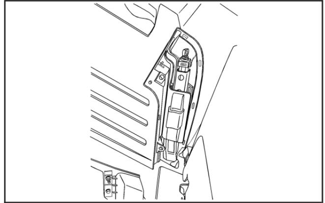
2. Insert the wheel wrench into the hole and turn it counterclockwise to release it.
