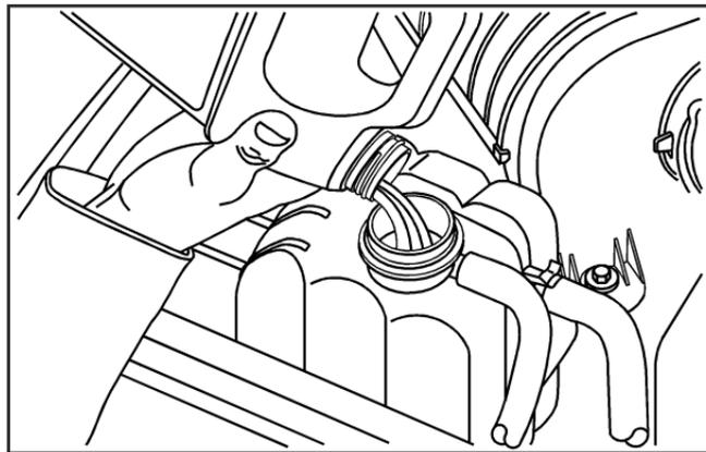
4. Fill the coolant surge tank with the proper mixture, to the FULL COLD mark.
