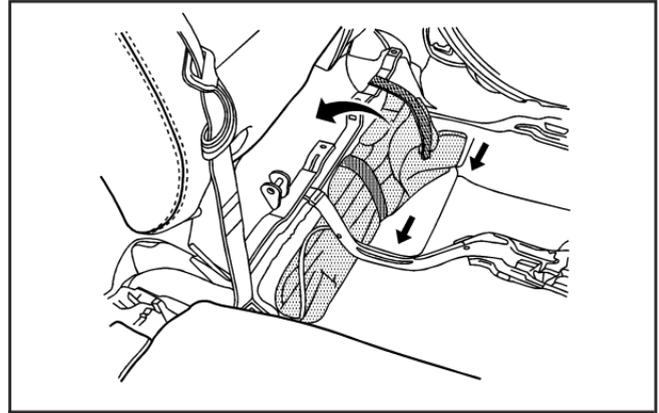
2. Remove the strap from the seat rail. Then carefully slide the tool bag out from under the seat rail as shown.
