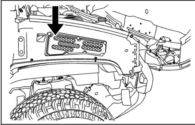
**Notice:** If you spray water into the engine air cleaner/filter intake and water enters the engine air cleaner/filter housing, as shown in the illustration, you could damage your vehicle's engine. The repairs would not be covered by your warranty. Do not spray water into the engine air cleaner/filter intake and/or housing.
