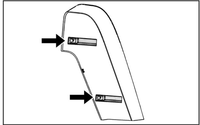
7. Replace the trim cover. Make sure the latches are pushed down.
