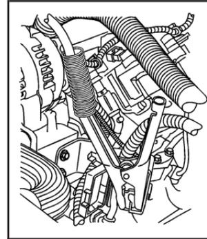
The remote positive (+) terminal is located near the engine accessory drive bracket. On some vehicles, the terminal may be covered by a red plastic cover. To access the remote positive (+) terminal, open the cover, if equipped.
