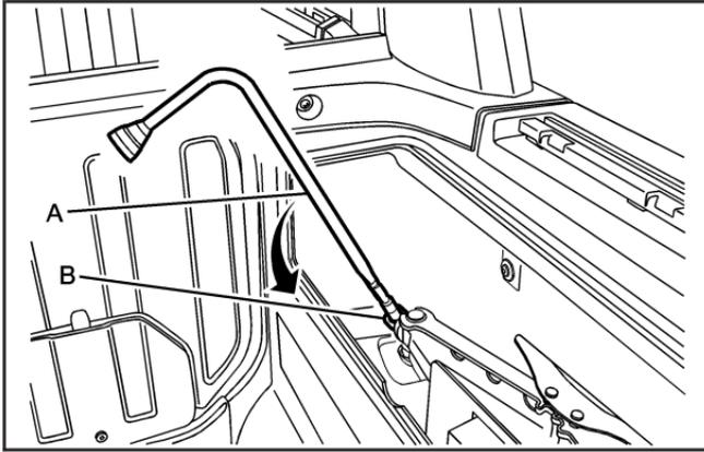
Release the jack by inserting the wheel wrench (A) into the hole (B) and turn counterclockwise.
