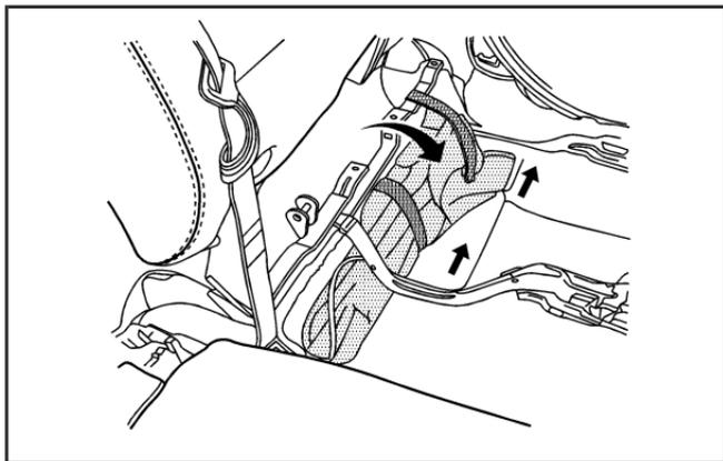
8. Place the narrow end of the tool bag under the seat rails as shown. Slide the tool bag under the rear seat. Be careful not to pinch the seat cables or electrical harnesses.
