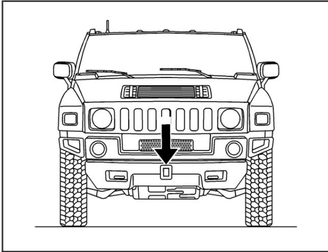
Your vehicle is equipped with a front mounted receiver.
