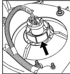
3. Turn the bulb/socket retainer counterclockwise to unlock the bulb/socket.
