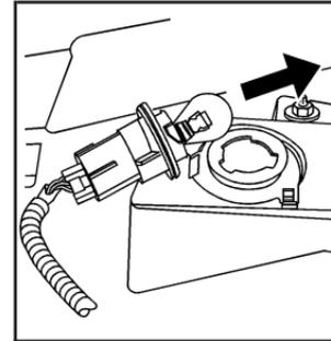
3. Turn the bulb socket counterclockwise and remove it from the lamp housing.
