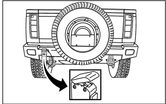
2. Lift up on the latch on the left side of the vehicle to release the spare tire carrier from the vehicle. The handle will stay in the raised position until the spare tire carrier is closed and latched properly.
