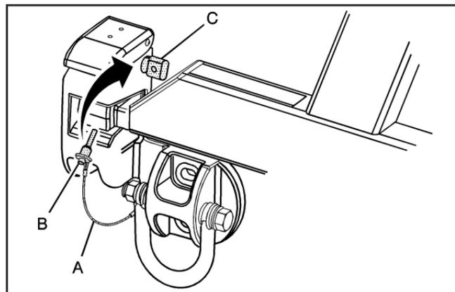
3. Reinstall the cable (A) by pushing in the button on the pin (B) and inserting the pin into the latch bolt nut (C).
