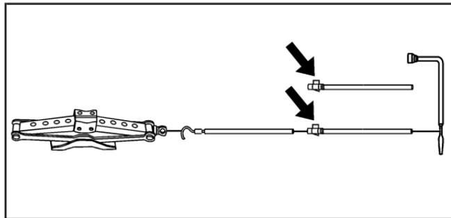
**Rear Flat Tire:** Assemble the jack together with the jack handle and the jack handle extensions.
