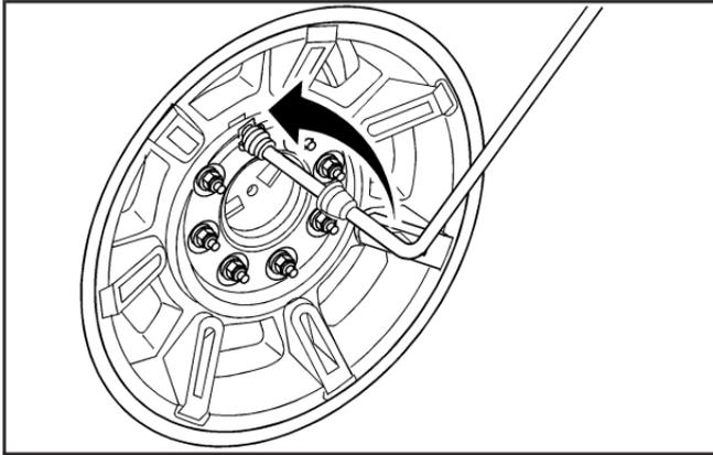
5. Remove the three wheel nuts holding the spare tire onto the tire carrier.
