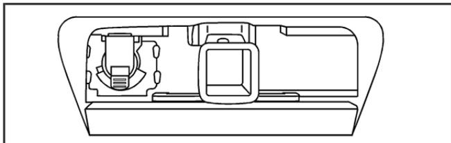
Your vehicle is equipped with the seven-wire trailer towing harness. This harness with a seven-pin universal trailer connector is attached to a bracket on the hitch platform.
