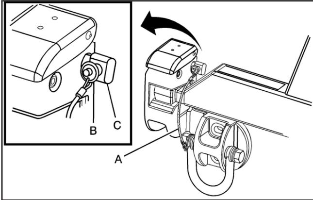
1. Press the button on the pin (B), which is attached to the cable (A), to remove the pin from the latch nut (C).
