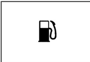
This light, under the fuel gage, comes on briefly while the engine is being started.
