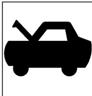
2. Pull the handle with this symbol on it. It is located inside the vehicle to the lower left of the steering column.
